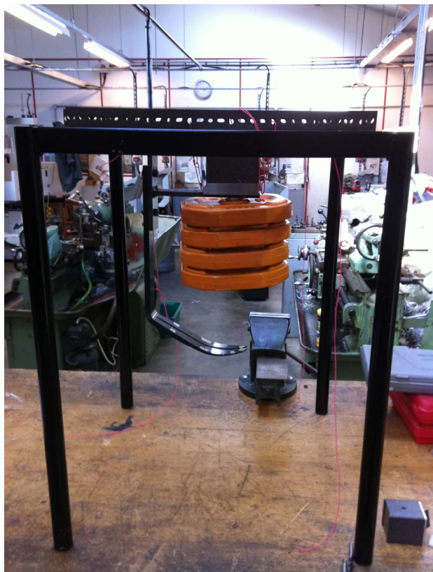
Figure 5. Prosthesis drop test rig.
