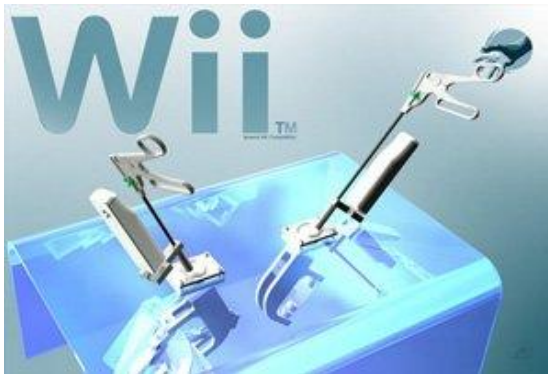
Figure 17: Customized Wii controllers as laparoscopic instruments (source: IMDS)
