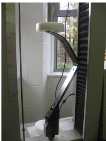
Figure 33. Prosthetic Blade Loading
