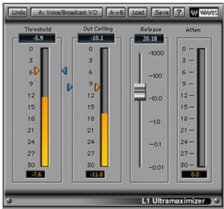
Figure 7. Contrary to the conventional audio normalisation, the maximiser plug-in allows to achieve the maximum level of the digital signal through 'lookahead' peak control, whereas its application does not degrade the quality of the initial audio signal (image: Waves L1 Ultramaximizer plug-in).
