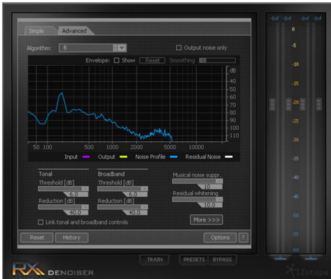
Figure 9. iZotope RX property window reveals the de-noising parameters that can be adjusted according to the spectrograph.
