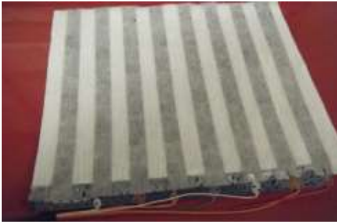
Figure 9: 8x8 matrix pressure mat tile with each element 5 mm wide and 15cm long [25]
