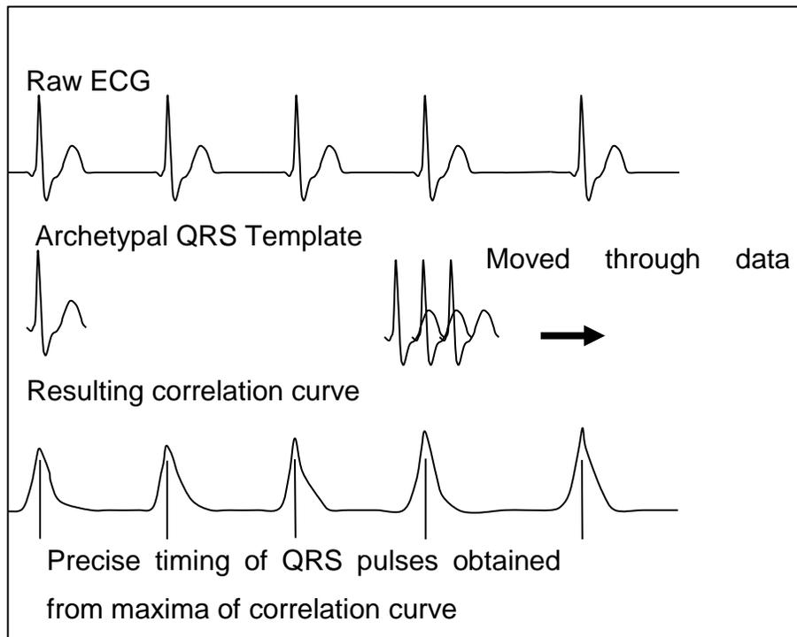
**Figure 12. Principle of Butfield and Bolton technique**
