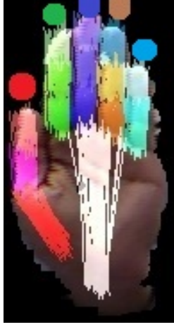
Figure 4.2: An example of hand part samples. The circles above the finger tips are sample patches for depth-background, depth-b, features, and the samples drawn as lines are centers of the hand parts samples for the depth-foreground, depth-f, feature.
