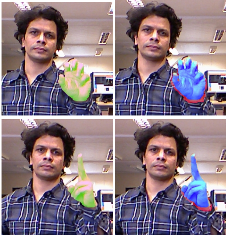
Figure 4.5: Examples of hand region segmentation. First column: green color (semi-transparent) represents the ground truth. Second column: blue color (semi-transparent) represents the segmented hand region using proposed technique, and red color denotes the segmentation error.
