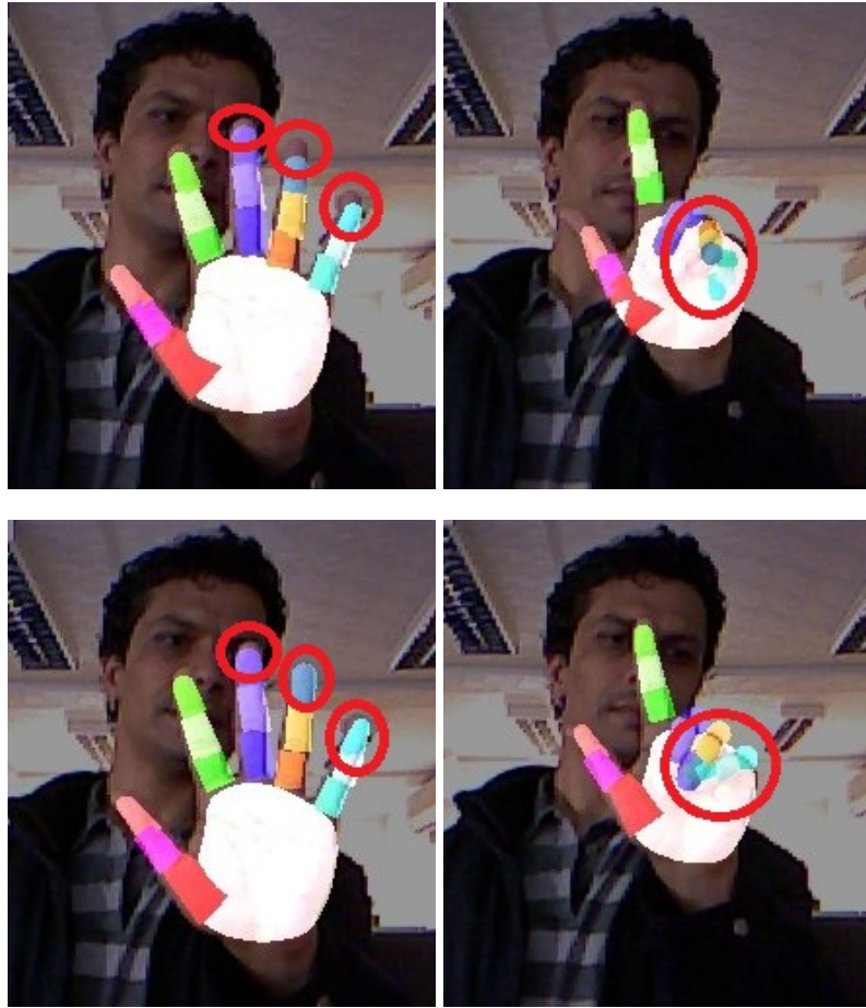
Figure 4.11: Results comparison between without context cue in first row and with context cue in second row. Index finger and little fingers are tracked well with context cue. Also, the context cue helps to recover the hand pose accurately as shown in second columns.
