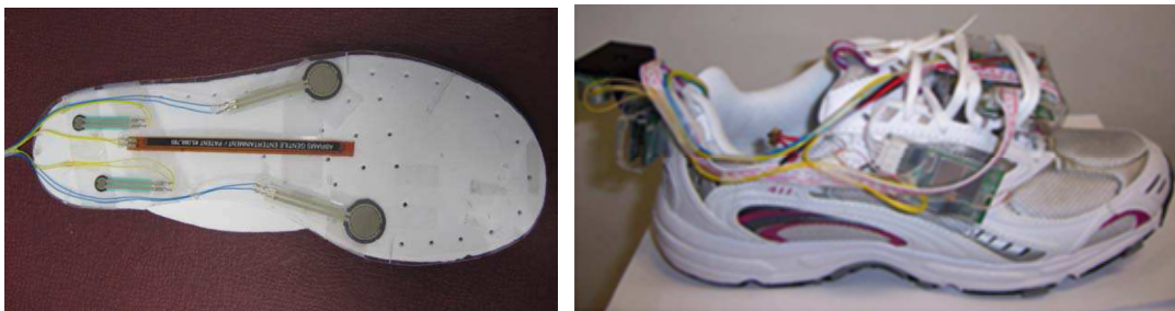
Fig. 3.1: Shoe system for abnormal gait detection. An insole with several force detection sensors attached was placed in a shoe (Chen et al. 2008) and was used for data analysis.
