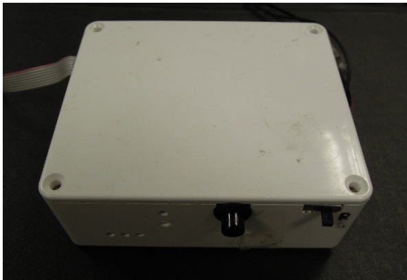
Fig. 3.17: Closed device housing and sensor unit showing the button that was used for user input.
