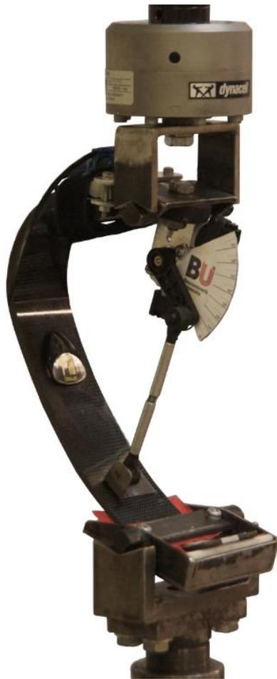
**Figure 4.9:** Test set up of the Ossur Cat.6Hi foot installed in the Instron test machine with the displacement instrumentation attached prior to calibration.
