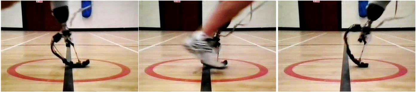
**Figure 4.6:** Still frames extracted from high-speed video (240fps) taken of a single stance phase during data acquisition showing heel strike, mid stance and toe-off.
