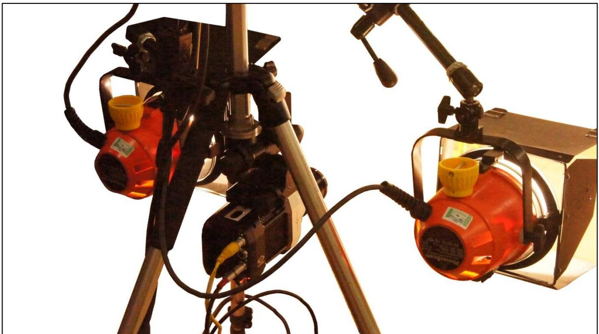
**Figure 7.4:** Image showing set up of the Phantom camera used for recording the action of the running foot on test with the two 500W halogen lights attached with a tripod.
