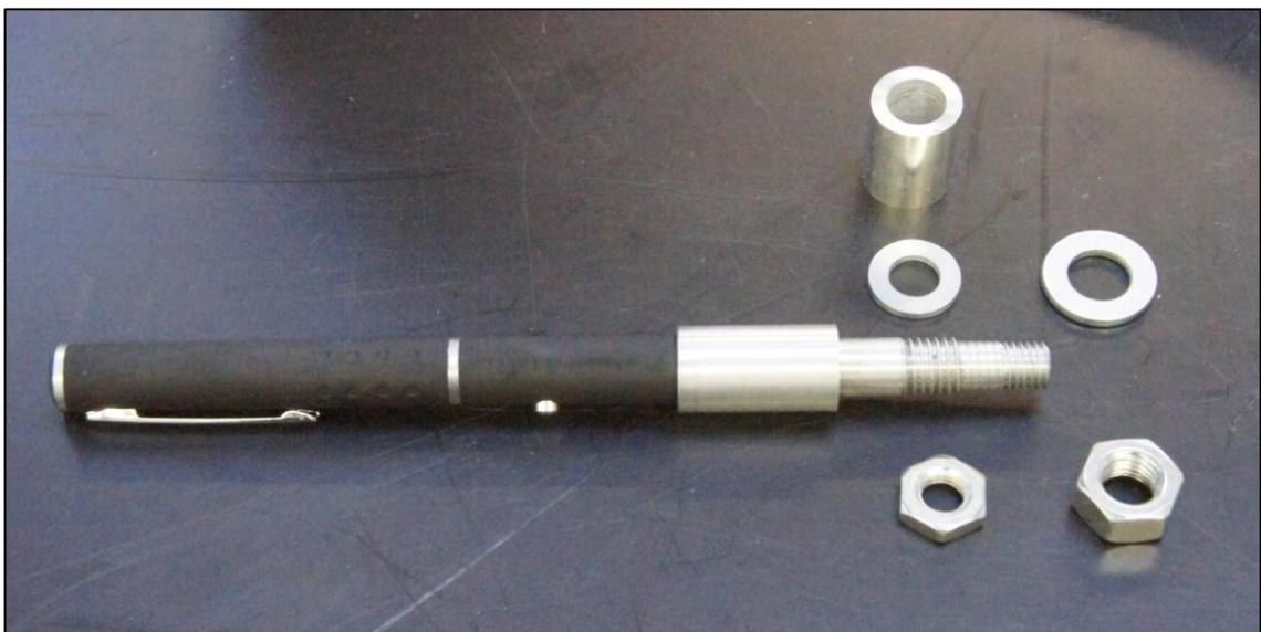
**Figure 8.5:** Image showing the fabricated cylindrical component attached to a generic laser pointer. This could be mounted to the shank of any Flex Run foot for marking the datum.
