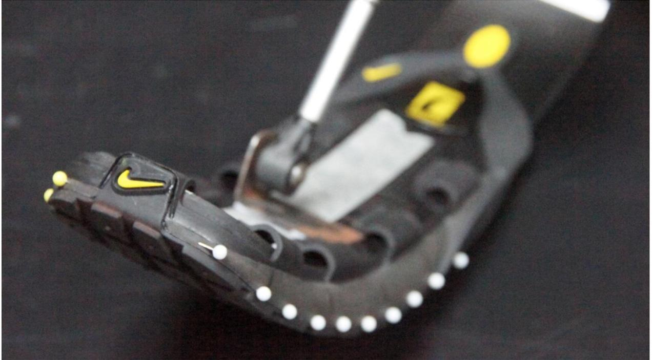
**Figure 7.3:** Image showing the pins that were inserted into the foam of the Nike running sole to demonstrate the ground contact position when filmed in HD super-high frame rate video.
