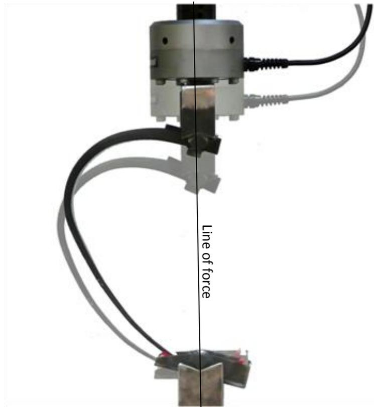
**Figure 3.19:** Pictorial representation of foot displacement during testing, demonstrating the deflected position of the foot and the line of force superimposed through the fulcrum points.
