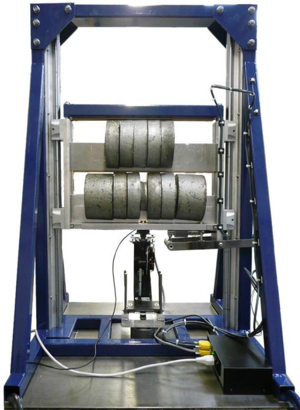
*Figure 5.10: Apparatus set-up to replicate the mass of the amputee athlete.*
