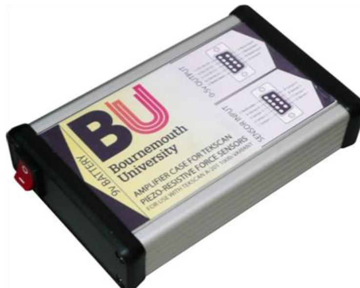
**Figure A1.3:** In-house signal conditioner for piezo-resistive sensors providing a 0-5v output.
