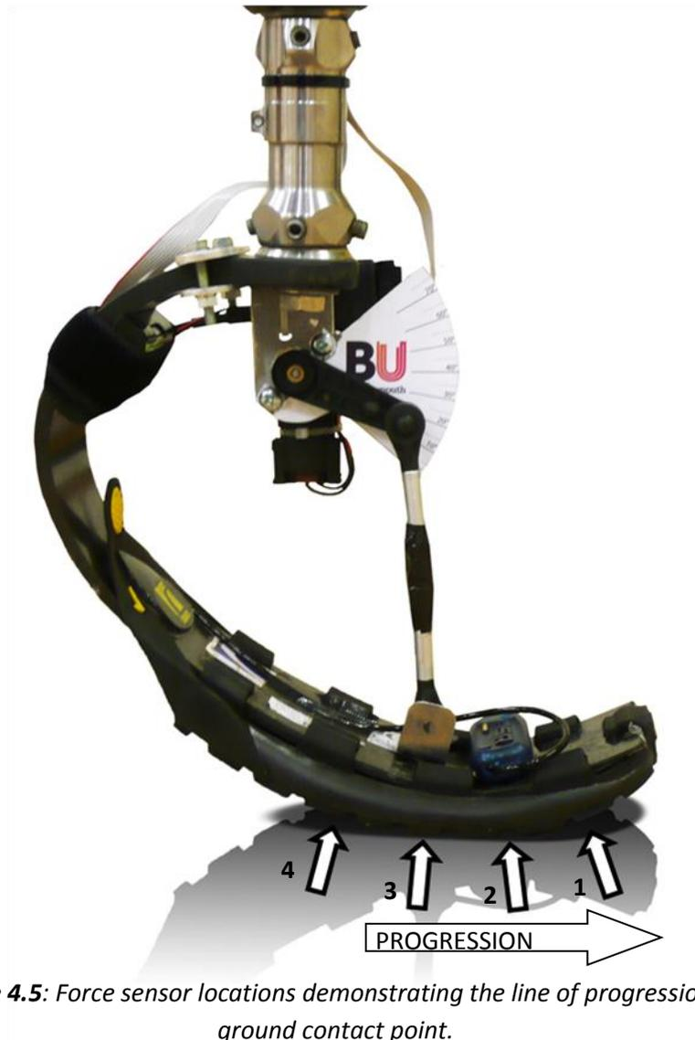
**Figure 4.5:** Force sensor locations demonstrating the line of progression of ground contact point.
