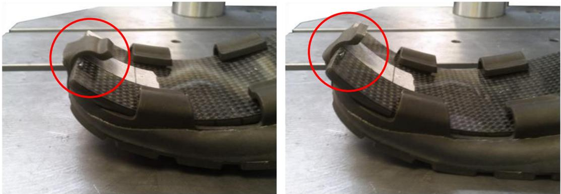
**Figure 3.11:** Lateral force exerted through the foot threatened to destroy the fastening cleats of the proprietary running sole.
