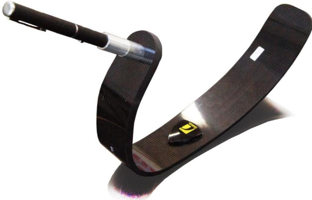
**Figure 8.5:** Image showing assembly of the laser device and foot prior to marking the position of the datum.
