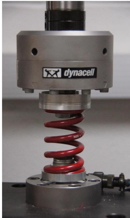
*Figure A3.5: Spring fixture used to amplify the displacement of the Instron crosshead for a given load and therefore improve data resolution*
