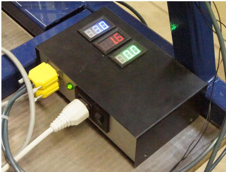
**Figure A3.2:** Amplifier case with output voltages displayed on the lid for each of the three channels requiring amplification.
