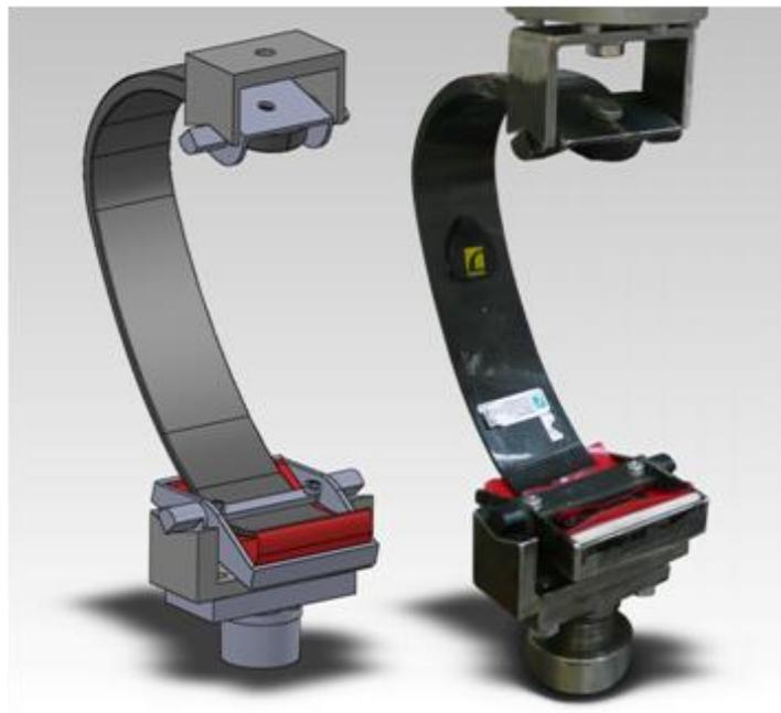
**Figure 3.15:** Testing fixture CAD design (left) and fabrication (right)
