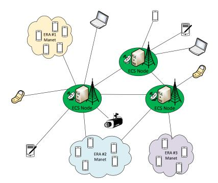
Fig. 1. Architecture of the emergency response network
