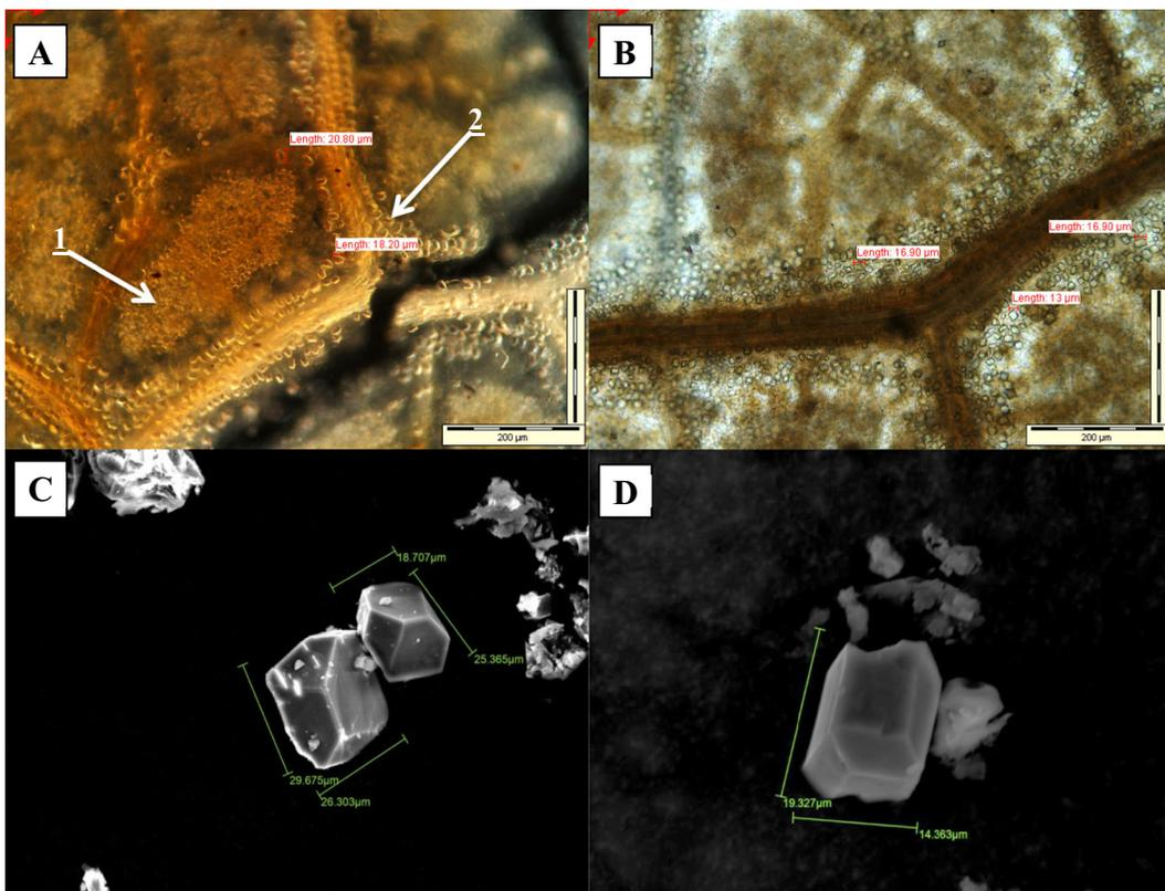
**Fig. 5** Calcium oxalate crystals observed and imaged in *Brosimum alicastrum* tissue using optical and scanning electron microscopy. **a** Druse / sand CaOx crystals (1) associated with the lamina, and prismatic CaOx crystals (2) associated with the vascular system of foliar tissue from a Haitian subject. **b** Prismatic and
