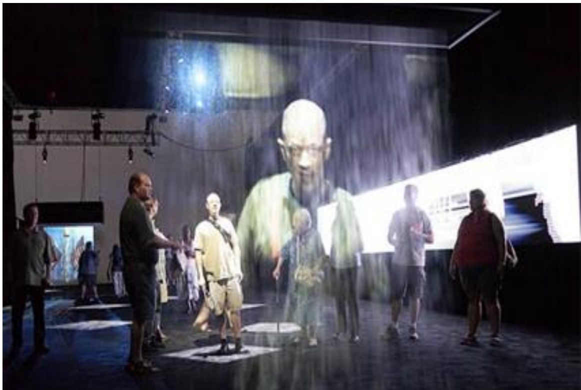
Fig. 49 - Fog Screen, A virtually invisible screen created of fog, 2006. (Gadget 2011)
