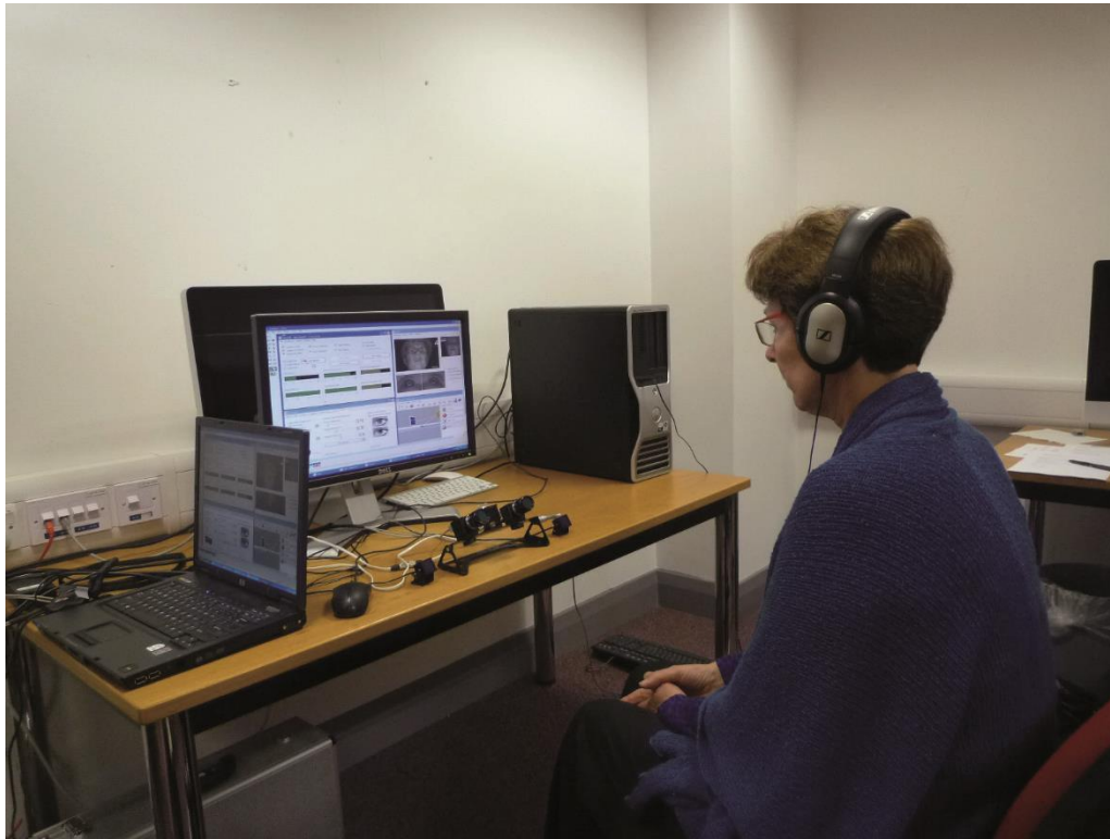
Figure 2. Equipment setup: display, eye tracker and headphones.
