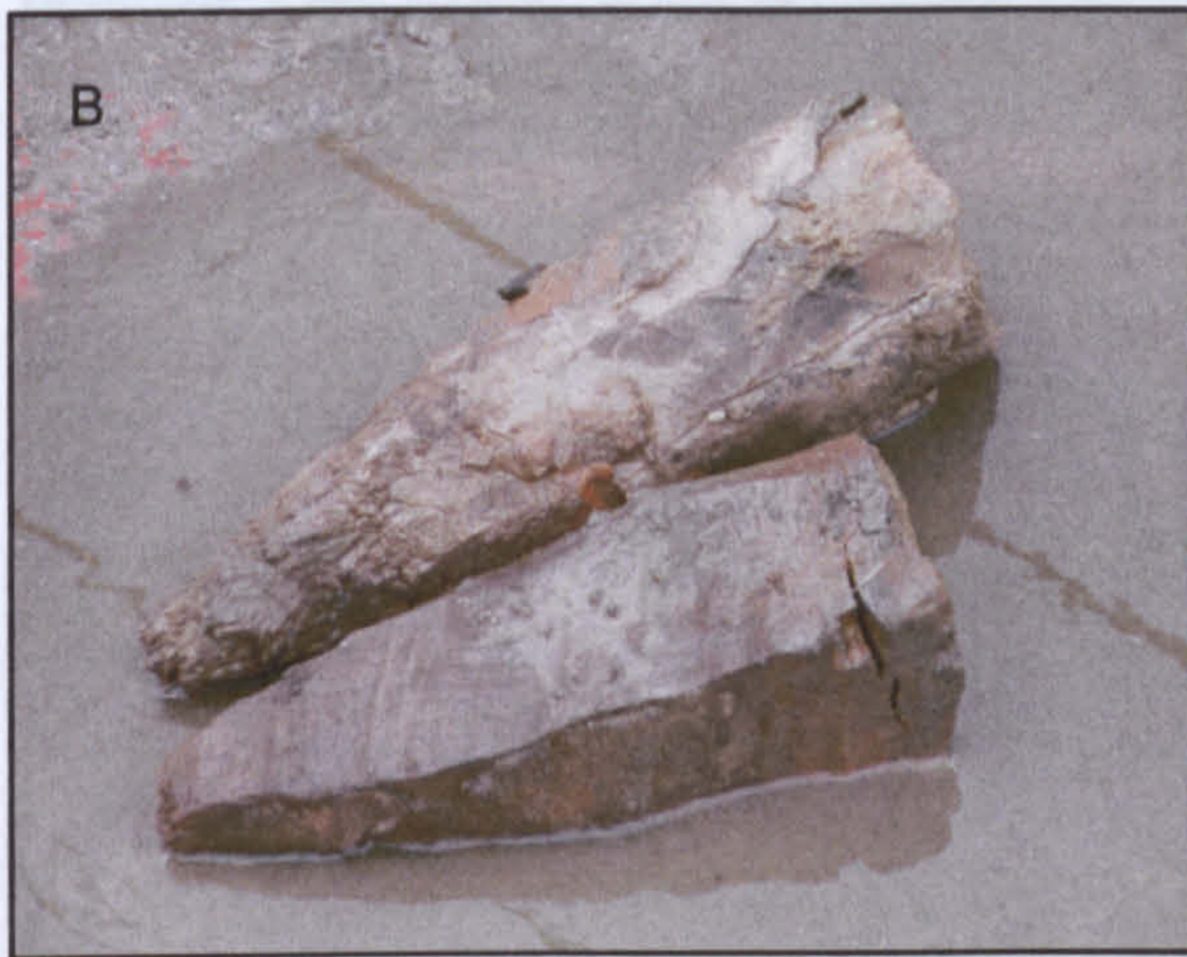
B: Oak points removed from the ends of piles during excavation. Length of longest point approximately 400mm.
