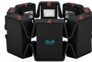
Fig. 1. Myo Armband uses 8 sensors on various muscles.
