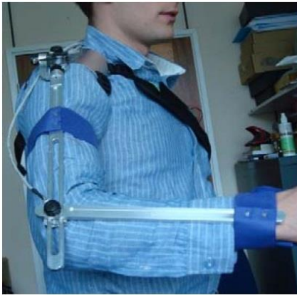
Fig. 2. AMMRIT custom made arm exoskeleton.
