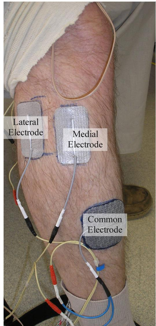
Figure 39: Example electrode placement (with 5x5 and 3.3x5.5 cm electrodes)
