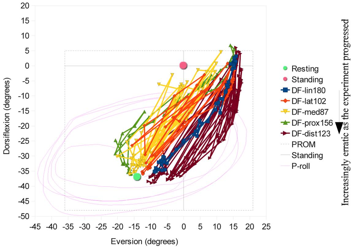
Figure 87: Single-channel stimulation - foot posture with current from  $I_{0\%}$  to  $I_{100\%}$  at five electrode positions, volunteer 25a. The foot response became increasingly erratic.
