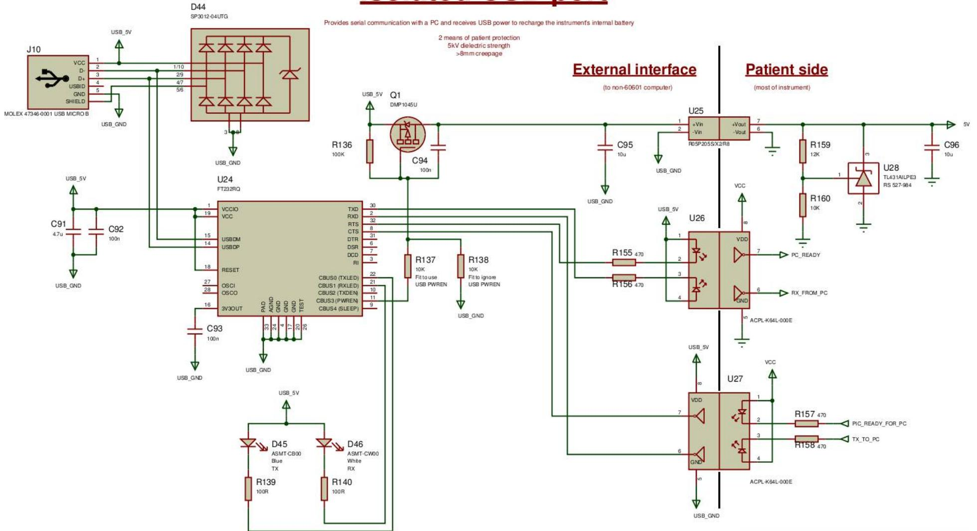
Figure 127: Isolated USB port providing communications and power across two means of patient protection at 250V AC.
