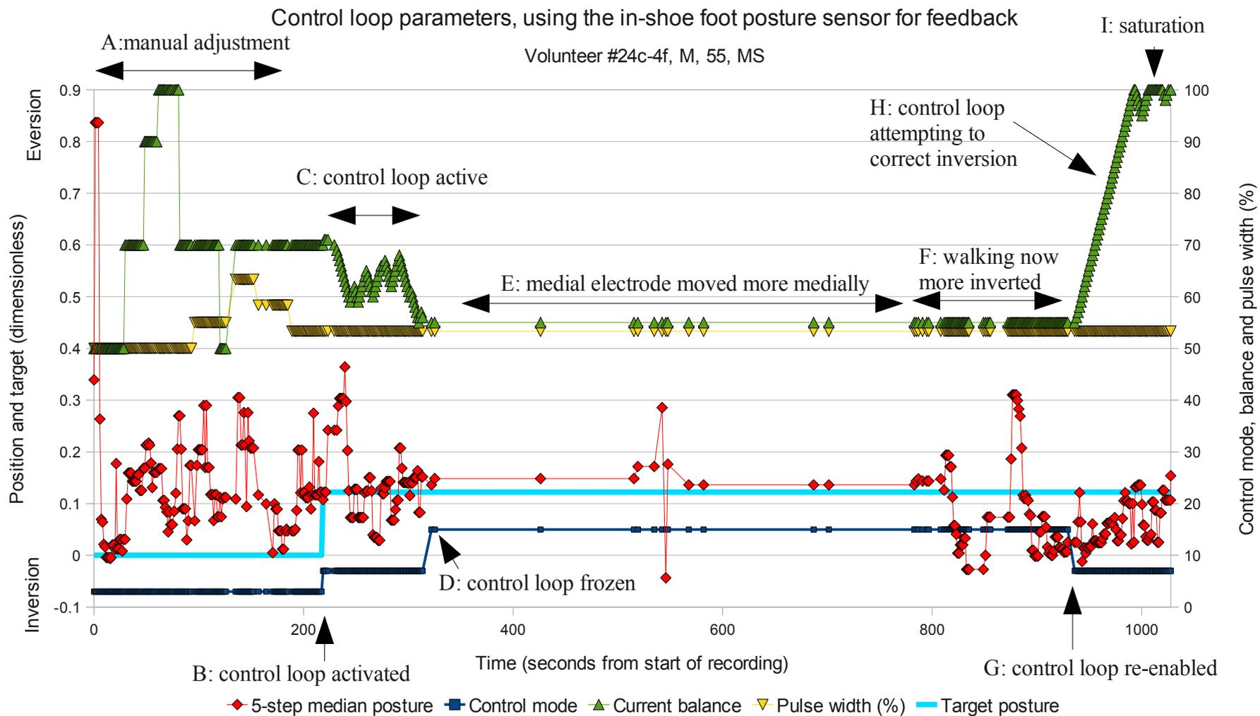
Figure 120: Closed loop control using the in-shoe foot posture sensor for feedback, volunteer 24.
