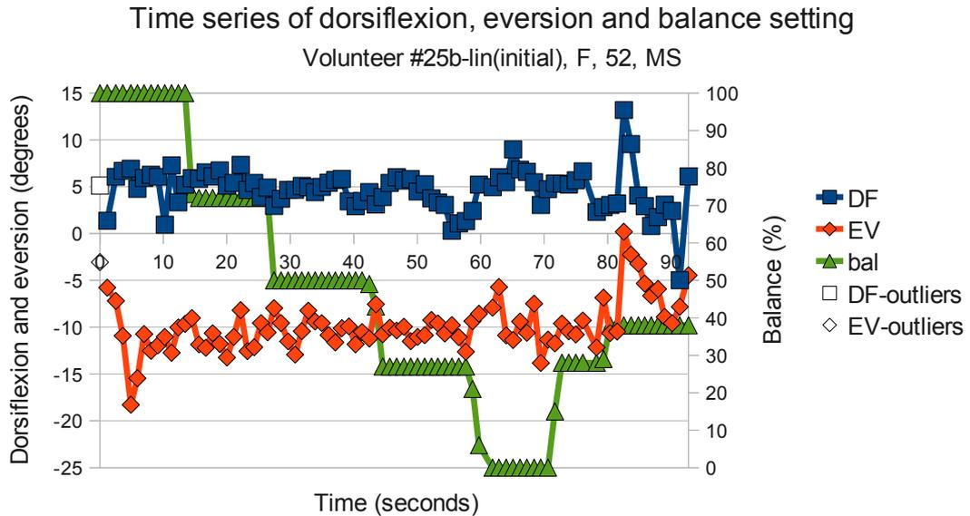
527 *Figure 115: Time series recorded during set-up for open-loop walking.*
