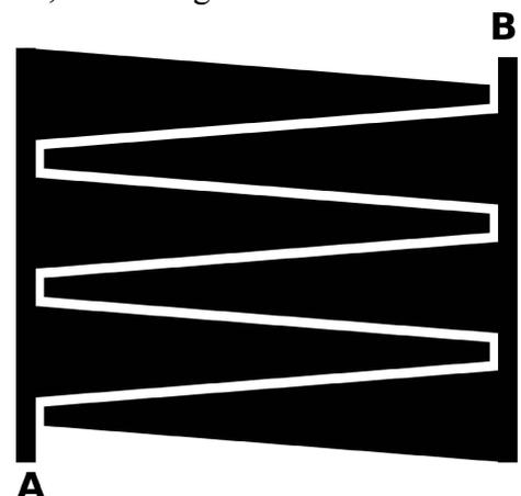
*Figure 122: Interdigitated electrodes for two-channel stimulation.*
