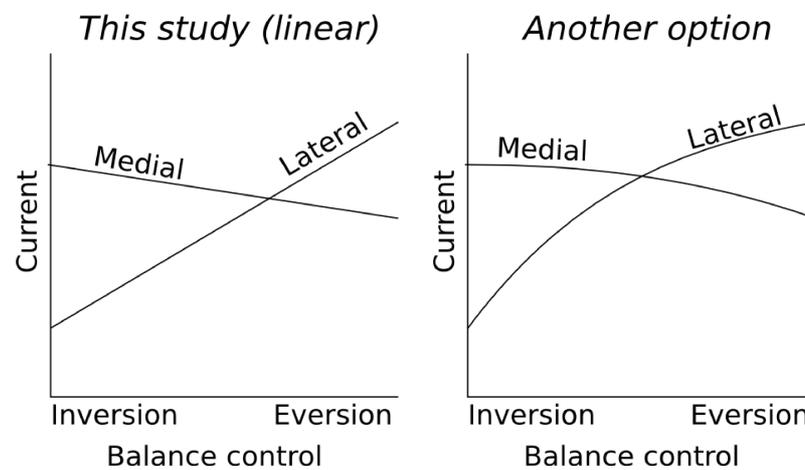
Figure 123: Example mappings from balance to current.
