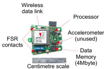
Figure 1: In-shoe signal processing board (approximately actual size)
