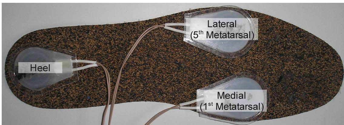
Figure 92: The FSRs of the in-shoe foot posture sensor (underside of a right-side sensor).
