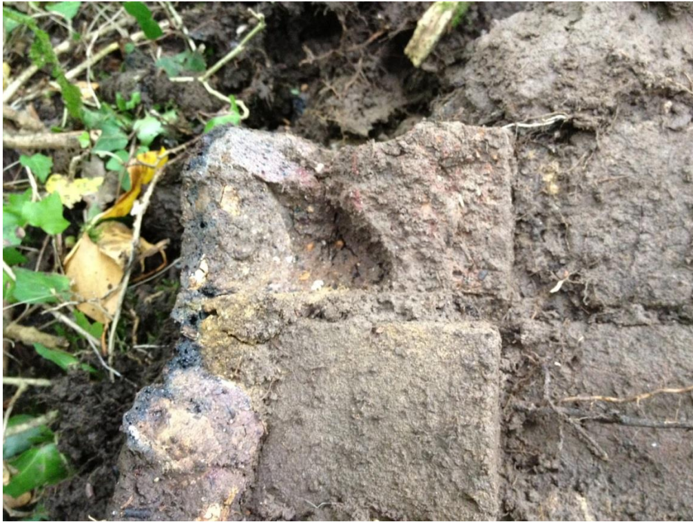
Figure 5.28. Example of a vitrified brick from Lower Lynch House
