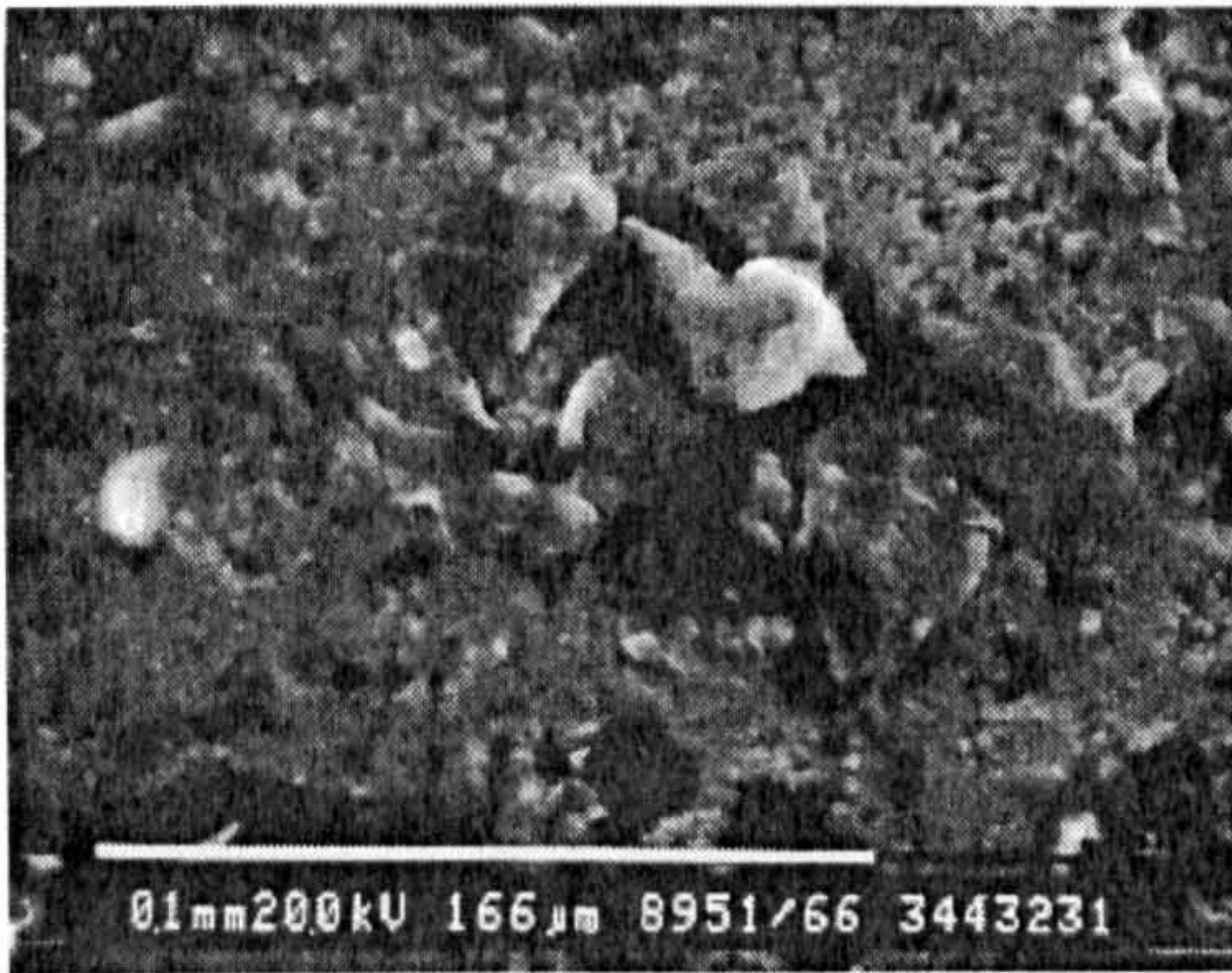
Fig 5-20 SEM of a pore with debris on wear track from Test 'B1'
