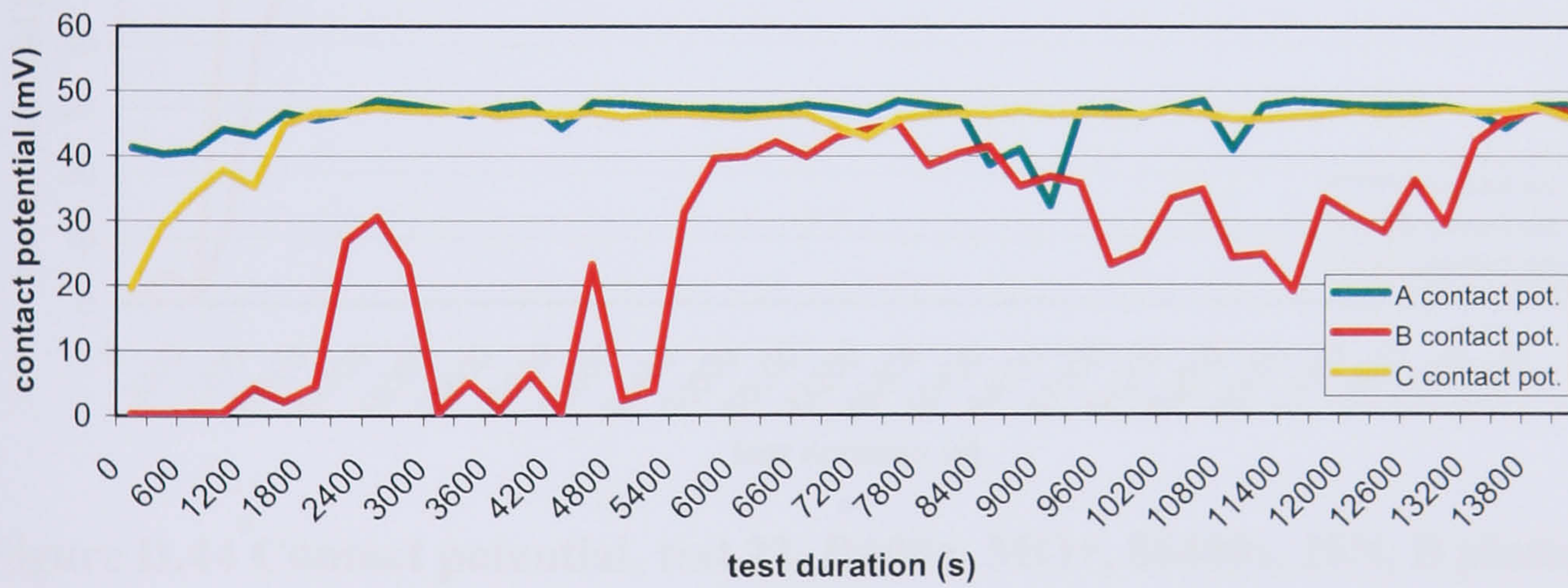
Figure D.40 Contact potential, test 20, R134a, POE, 14400s, 20N, B plates
