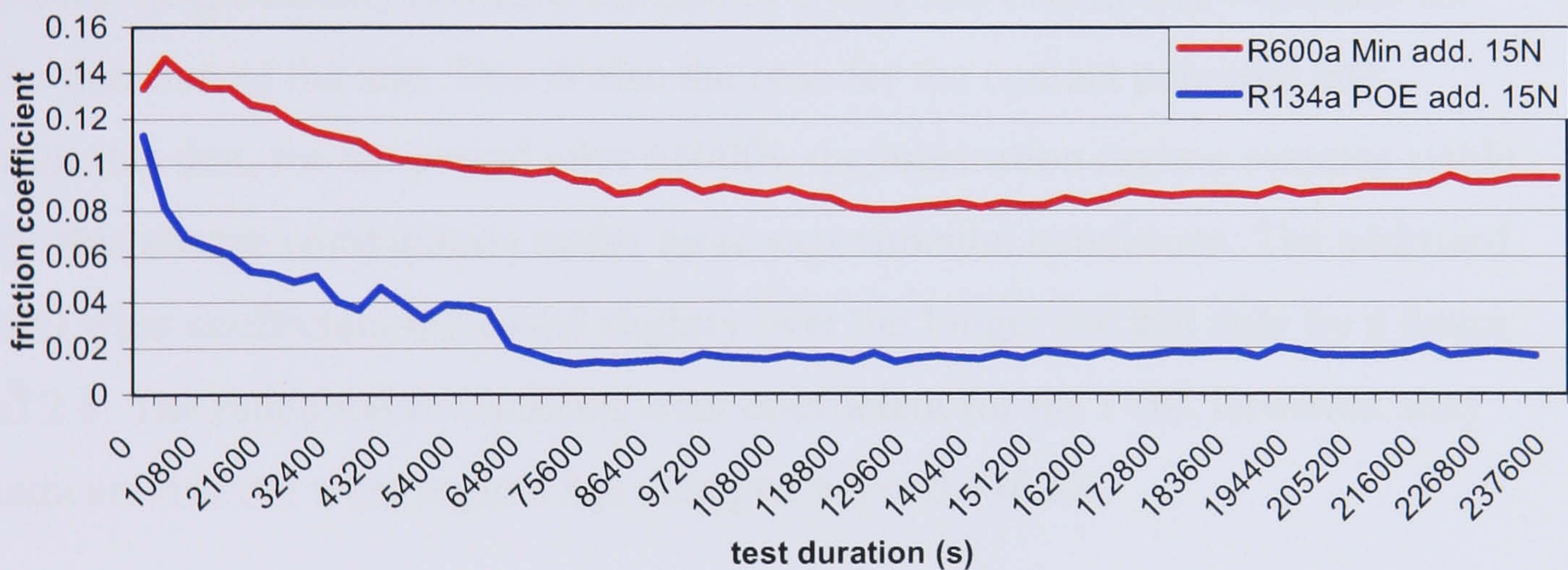
Figure 5.22 Reduced load test, friction coefficient 237600s, 15N, B plates
