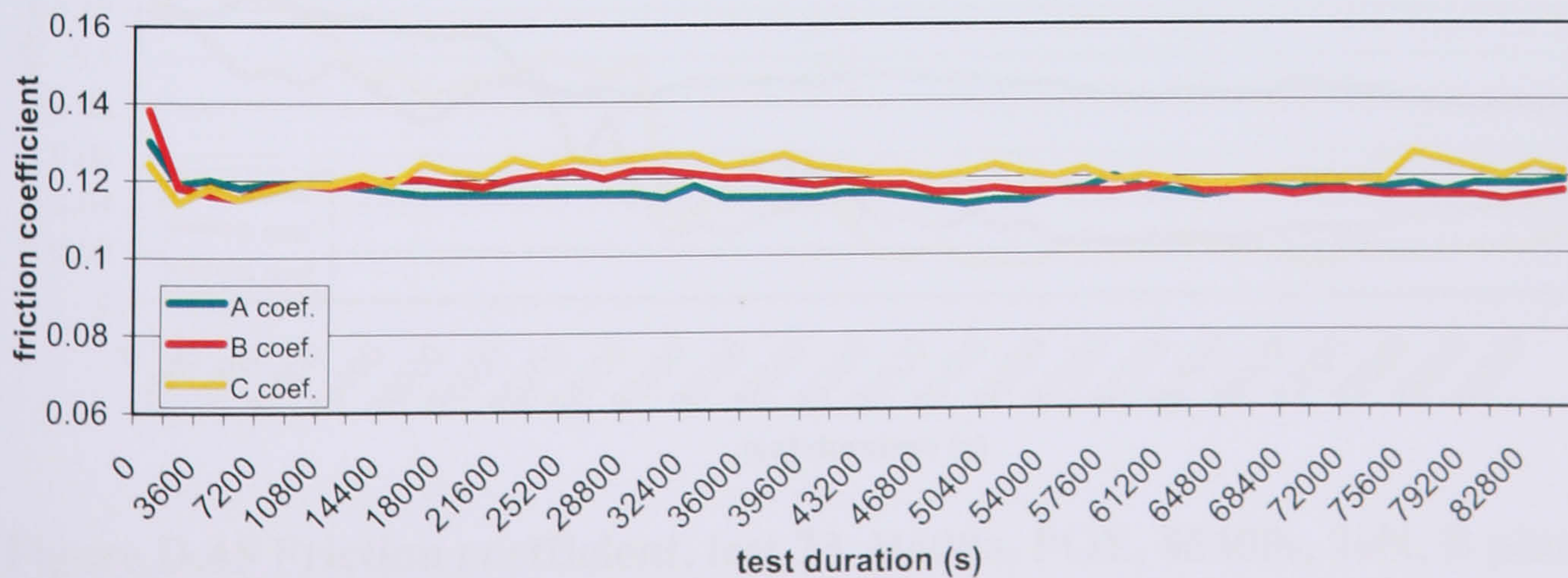
Figure D.41 Friction coefficient, test 21, R600a, MO, 86400s, 20N, B plates
