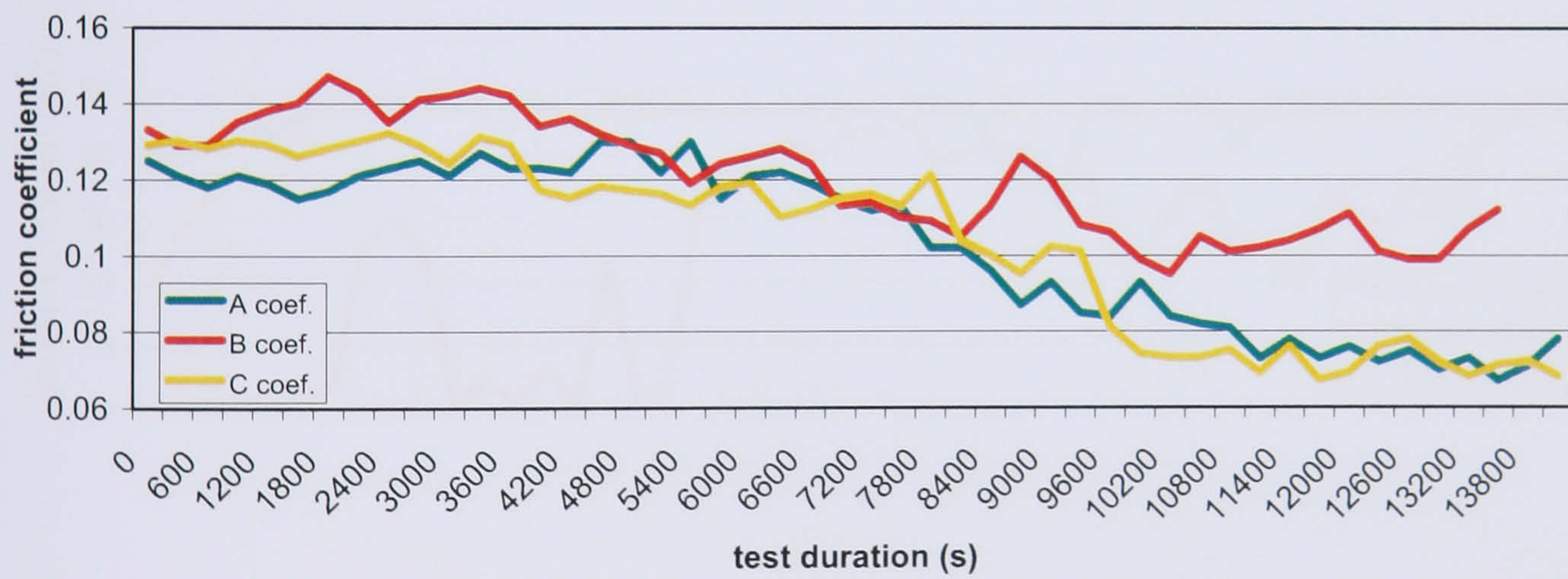
Figure D.37 Friction coefficient, test 19, R600a, POE, 14400s, 20N, B plates
