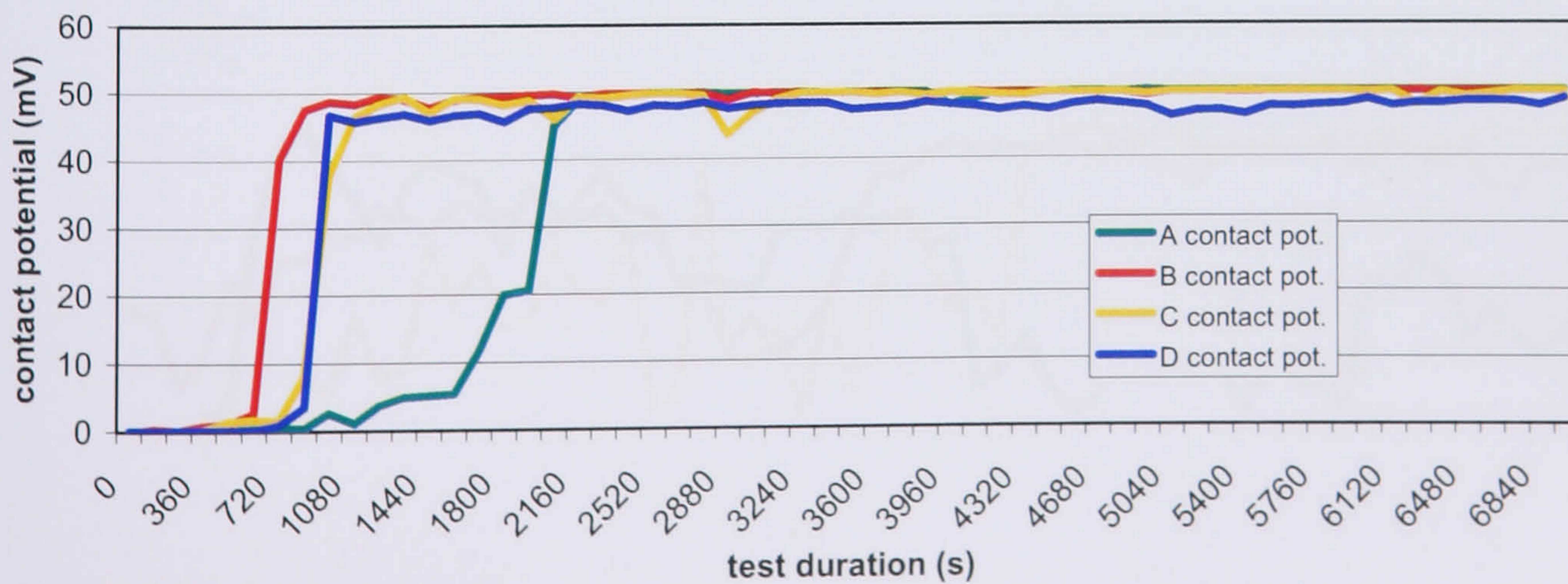
Figure D.28 Contact potential, test 14, R600a, MO+, 110°C
