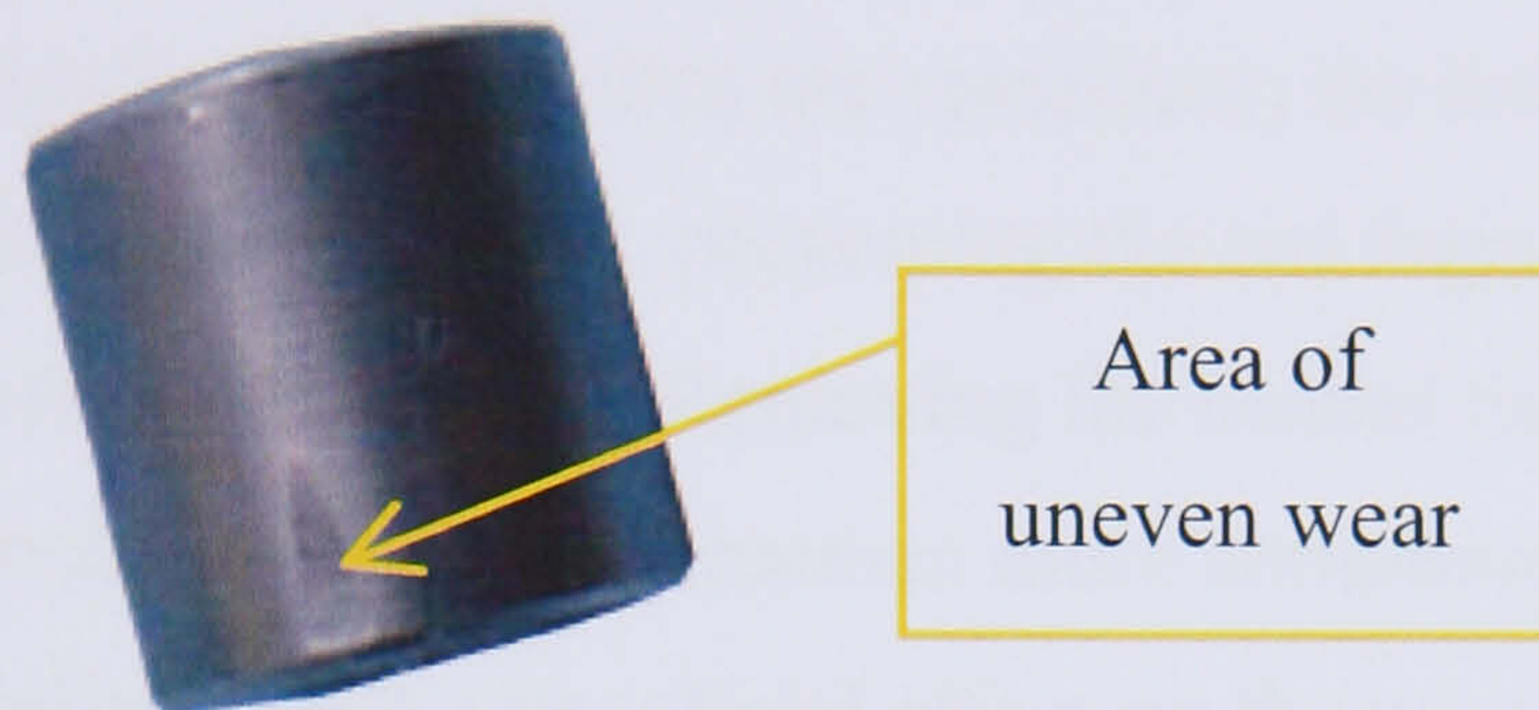
Figure 3.4 Uneven contact wear at pin sample
