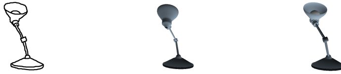
Figure 30: An example of the forward-backward ambiguity issue in inferred 3D pose of a lamp when not using the internal lines for additional information.
