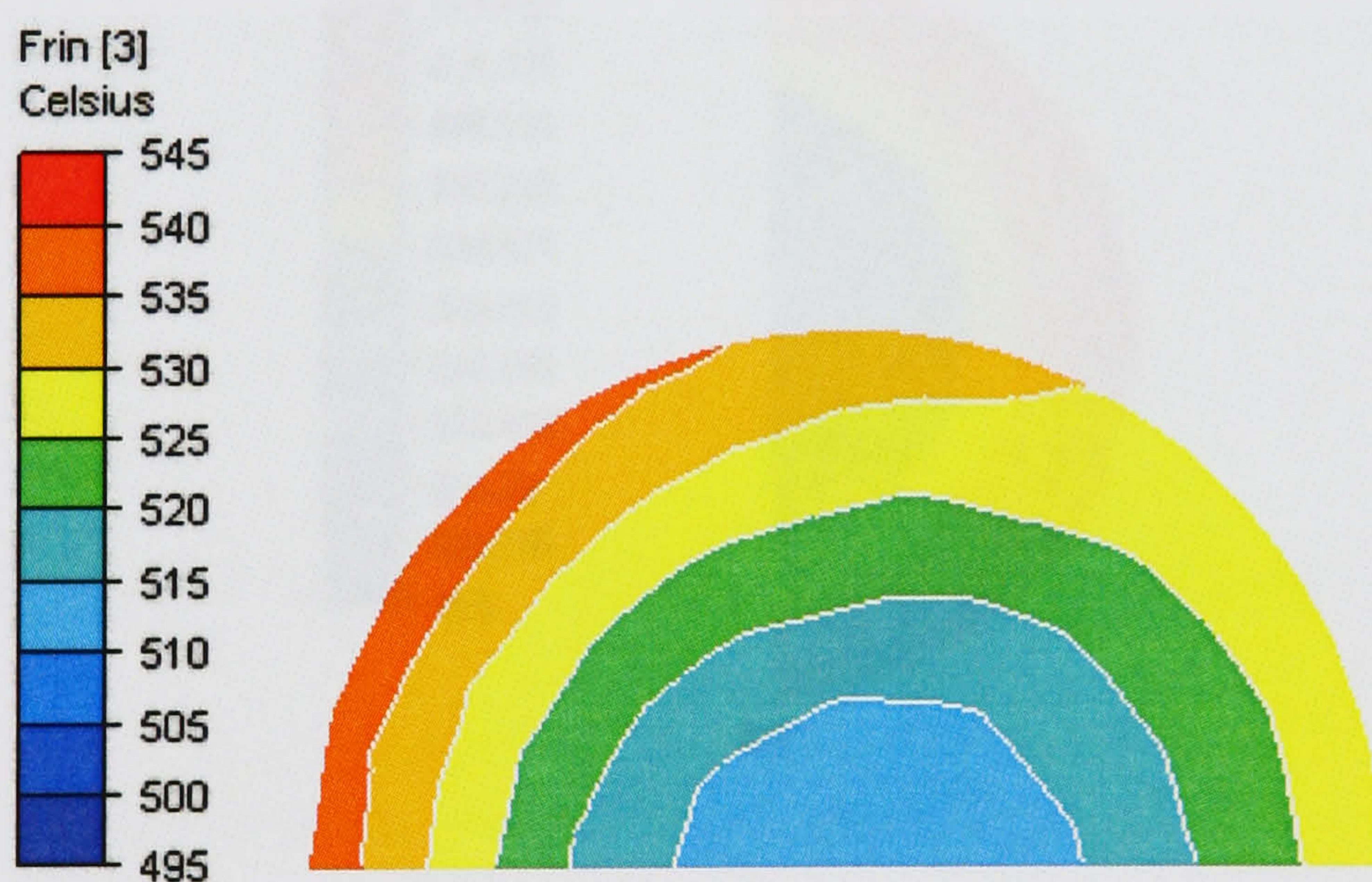
Figure 6.10(b) Cut plane of run 3 (in Celsius), Temperatures decrease towards the centre of the rod
