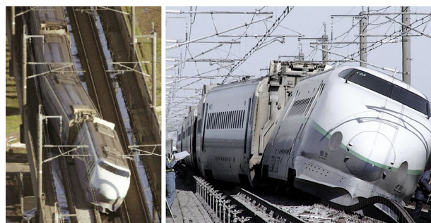
Fig. 2 The derailment accident of a Shinkansen train, in operation since 1964, which highlighted the need for increased focus on train post-derailment studies in both academic and industrial sectors [7]
