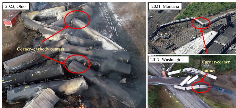
Fig. 4 Two typical contact–impact behaviours between the car bodies
