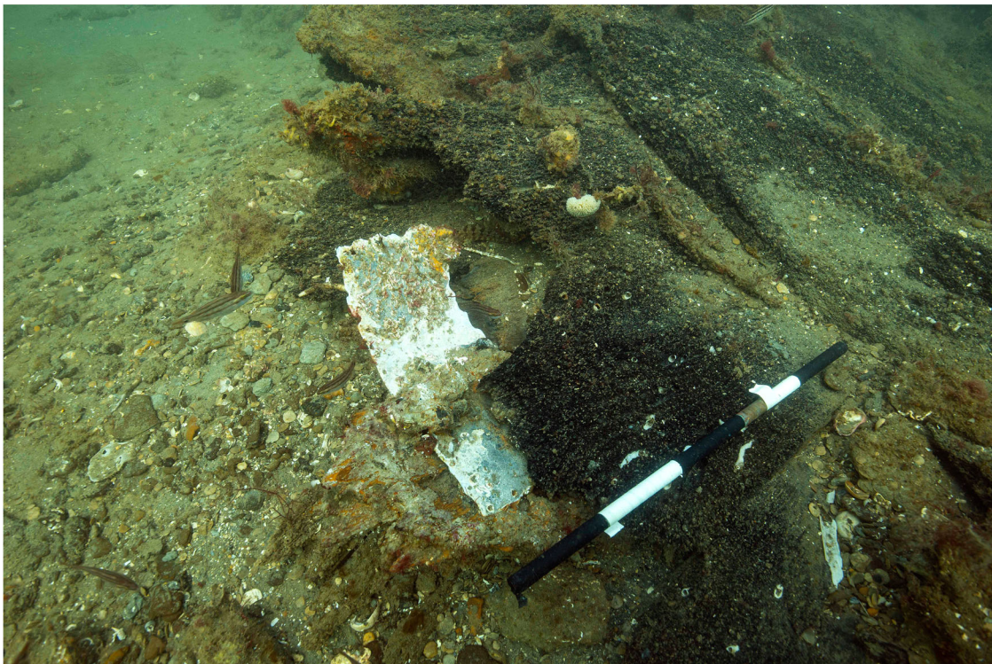
Figure 27. Photo showing lead tingle between sheathing and outer planks. Scale in photo is 50 cm with 10 cm increments (photo by Daniel Pascoe).
