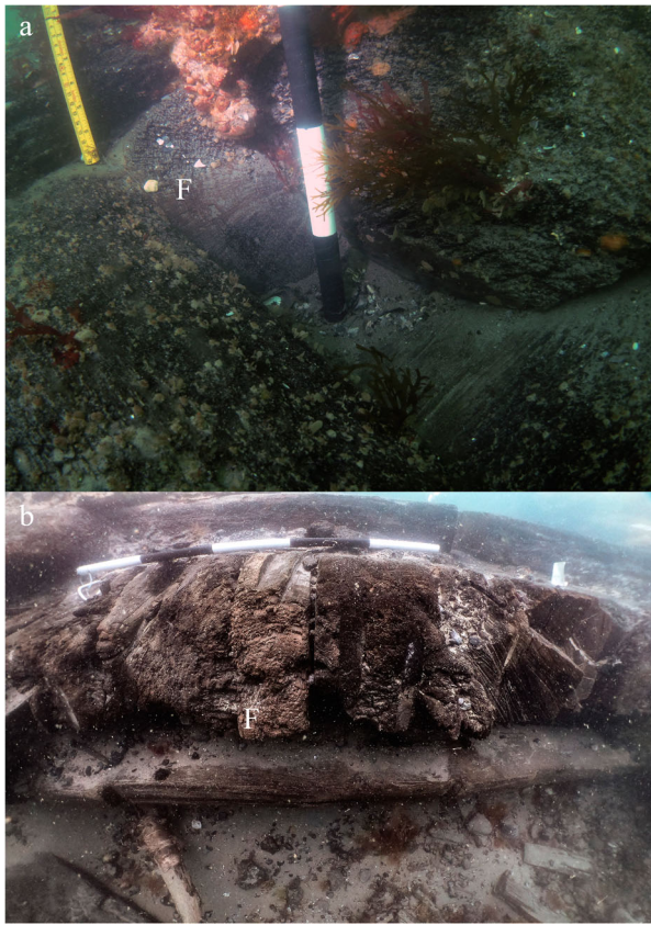
Figure 11. Structure from Invincible 1758. Photo A) showing filling timber between frame bends from starboard side stern structure from roughly gun deck level, the scale is 50 cm with 10 cm increments. Photo B) shows filling timber at roughly the floor heads on the starboard side amidships, the scale is 1 m with 20 cm increments (photos by Daniel Pascoe).
