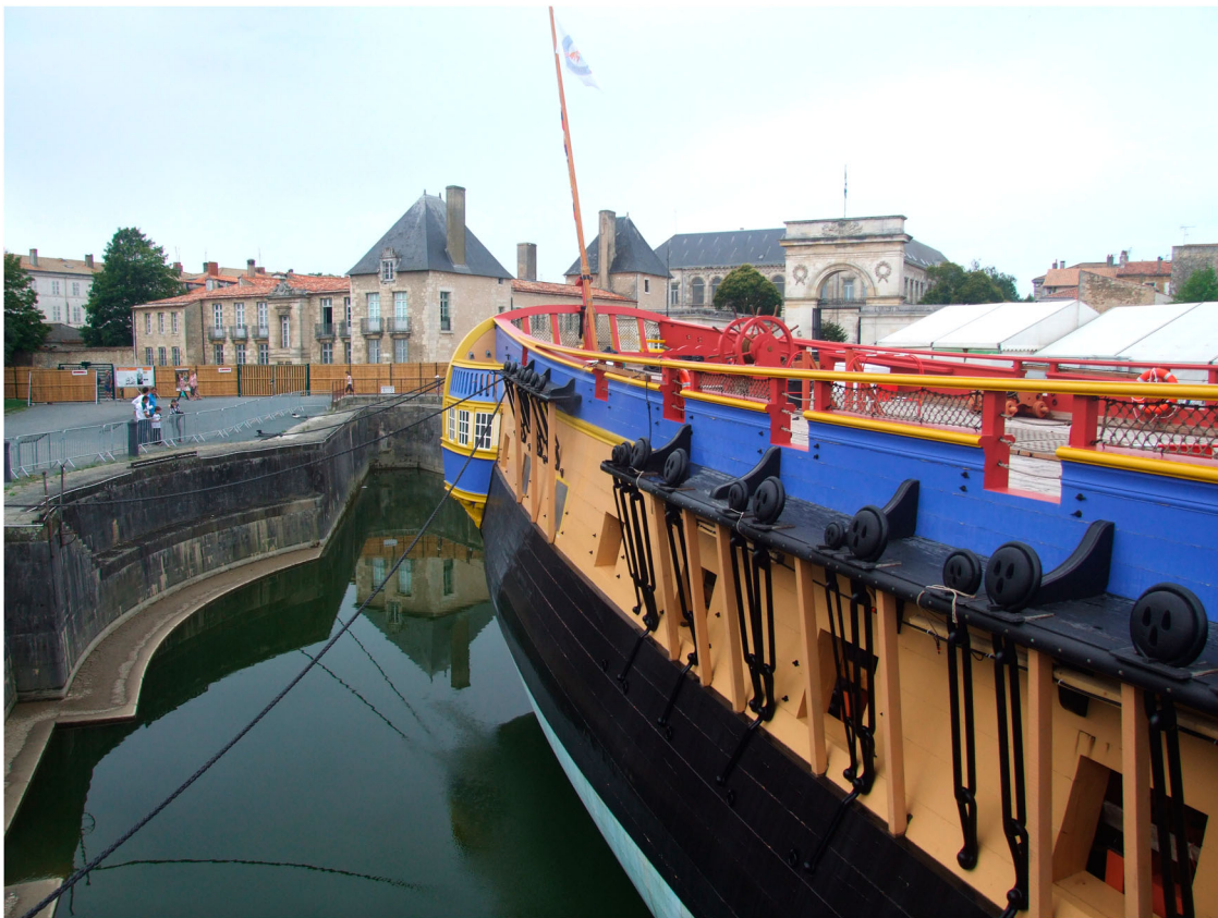
Figure 35. Photo of L' Hermione showing lower deadeye with shrouds and chain plates. The bottoms of the chain plates are bolted to the outside of the hull and the deadeyes are located along the chainwale (photo by Daniel Pascoe).
