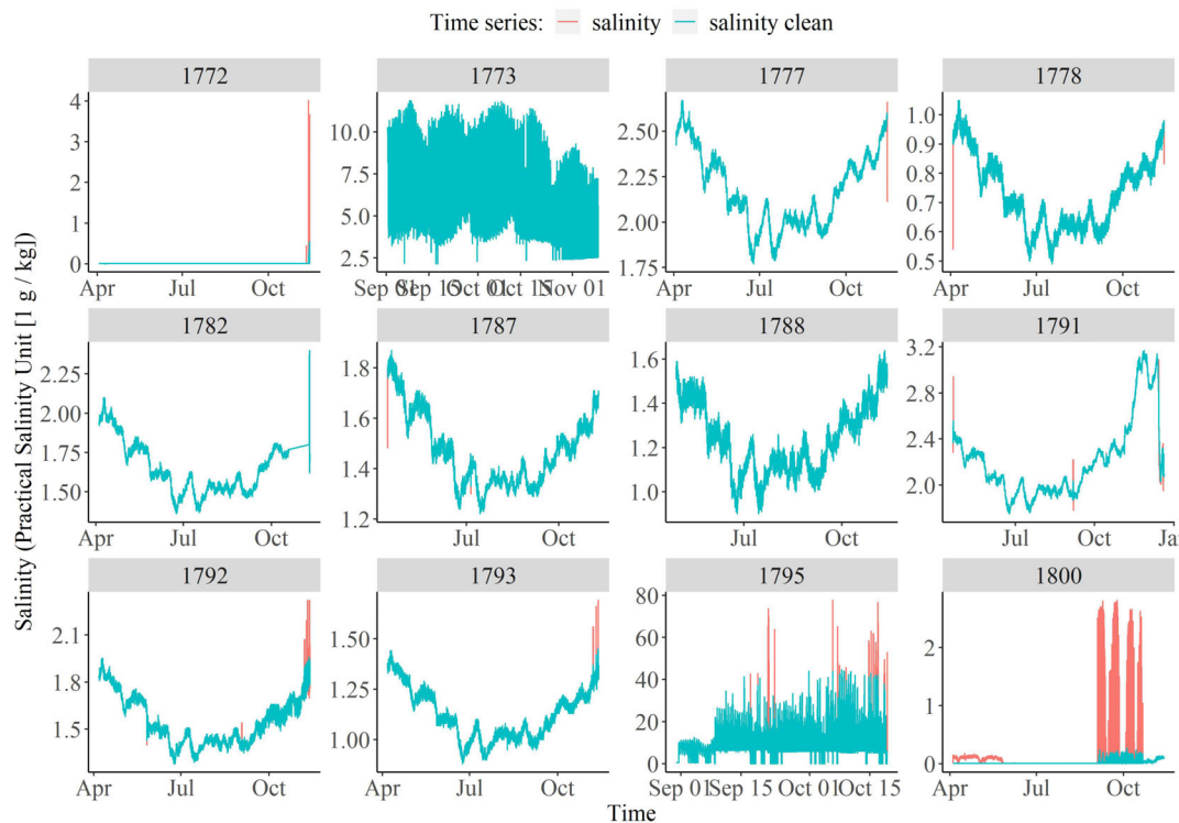
FIGURE 2 Plot showing the original and cleaned salinity measurements recorded at each logger. Cleaned salinity measurements were treated for statistical outliers. Even after cleaning, measurements taken on loggers 1772, 1795, and 1800 were considered unusable.
