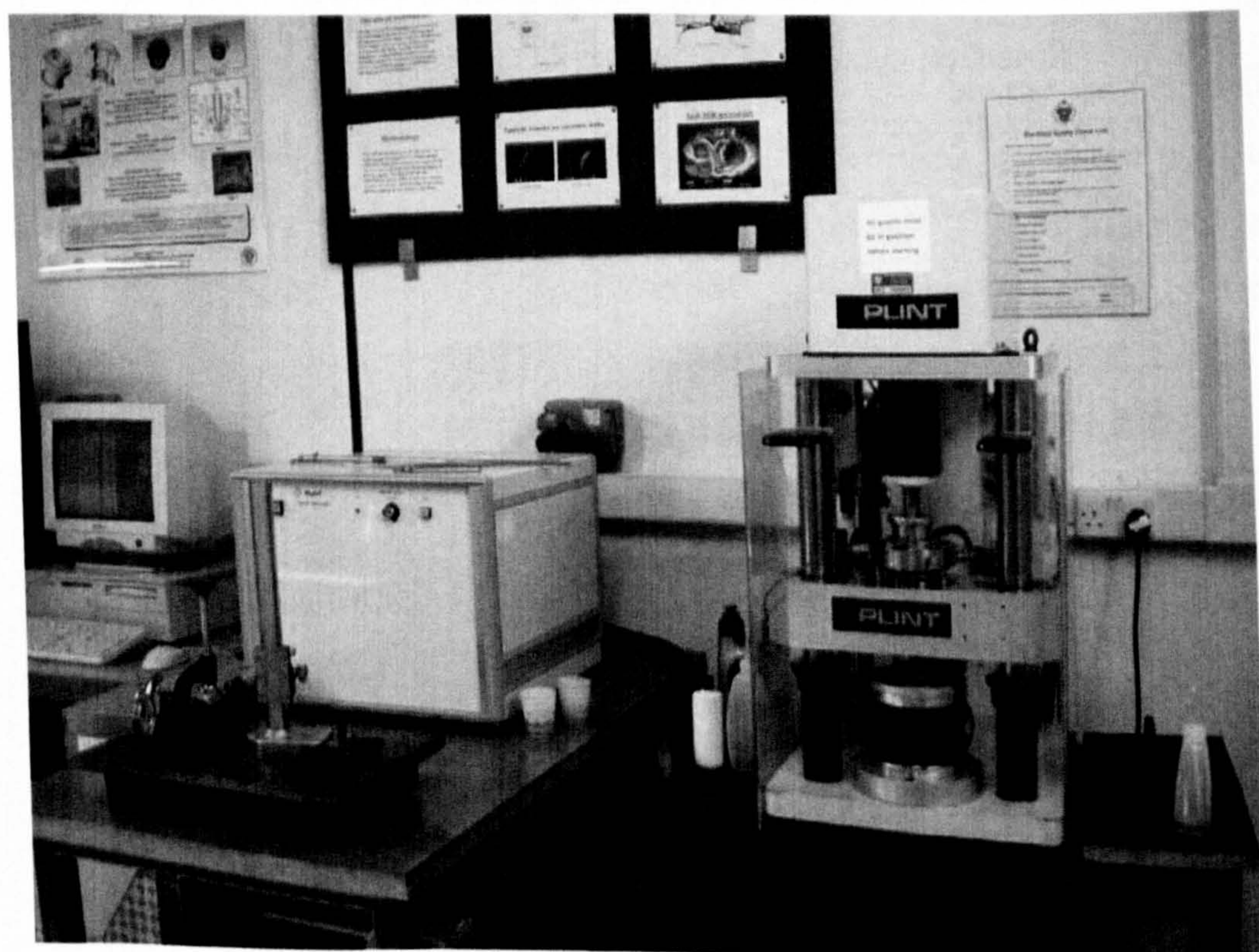
Figure 3.2 Rolling contact fatigue bench test
