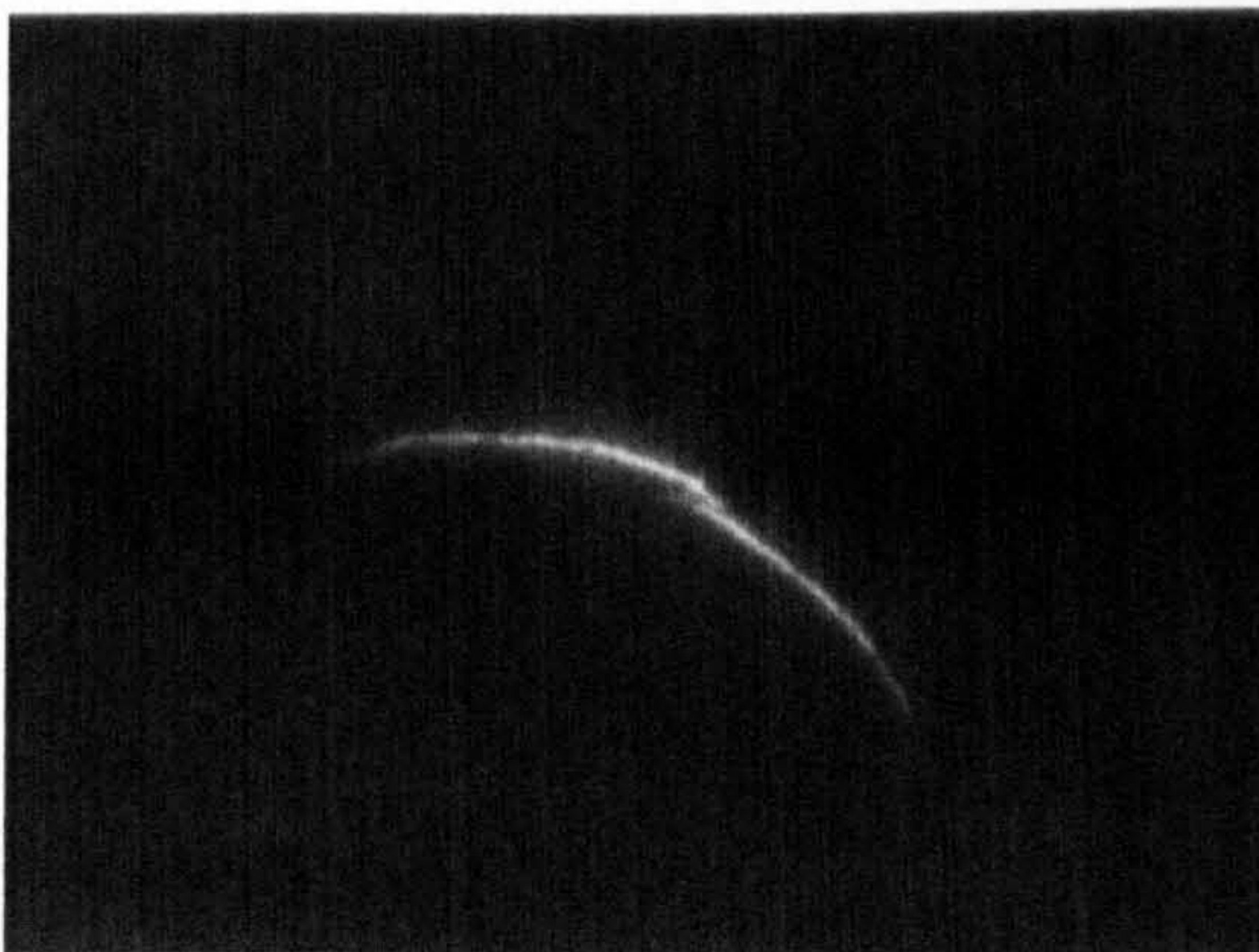
(a) Pre-test ring crack (UV light)
