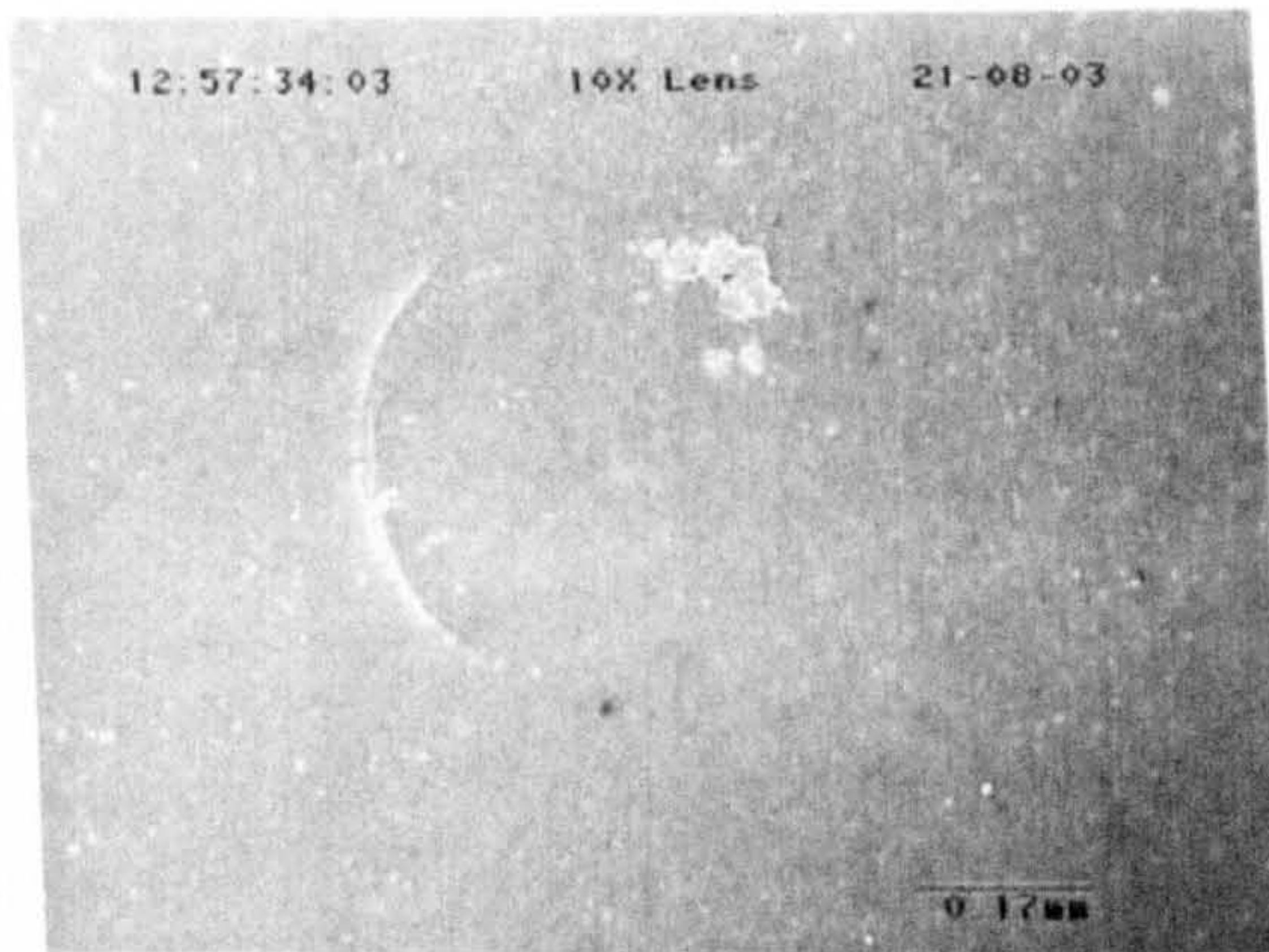
(a) Artificial crack before test
