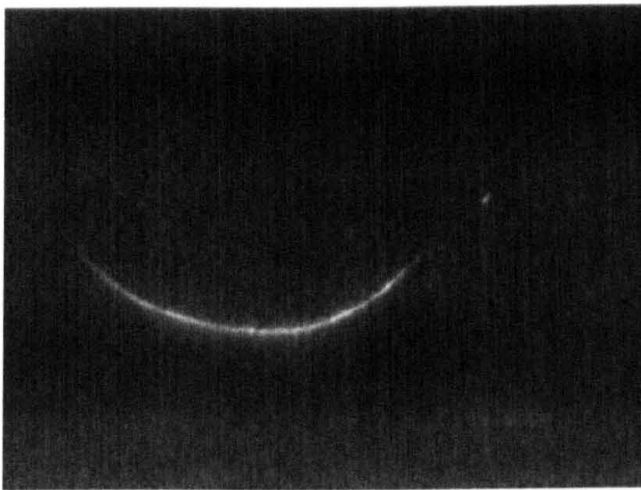
(a) Pre-test ring crack (UV light)
