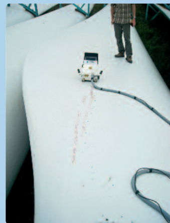
Figure: Q810 system on a turbine blade with detected wrinkle marked in red.
