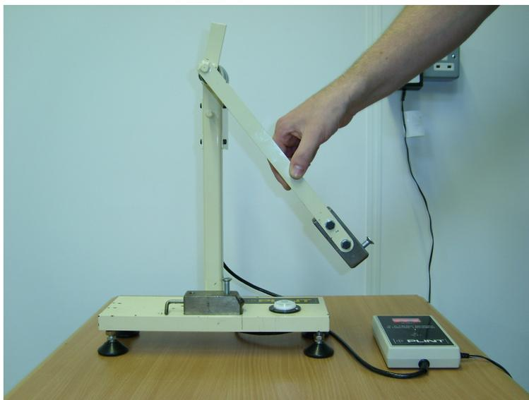
Fig: 2.3 Crack generation using a Plint impact pendulum
