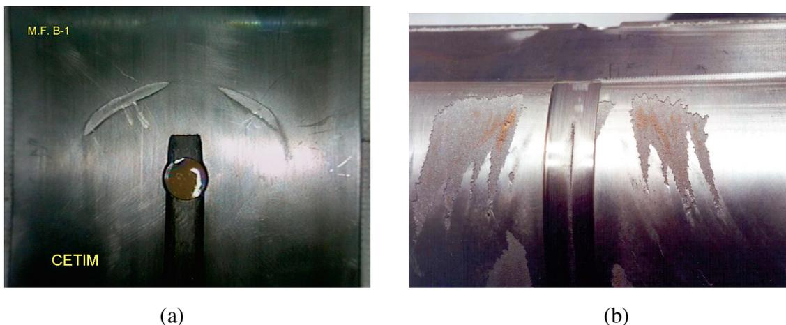
Fig: 1.7. (a) Cavitation erosion of diesel engine main bearing and (b) wear on hydrodynamic bearing surface (Chen 2005).
