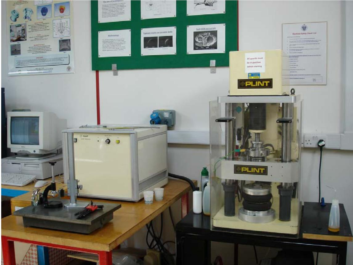
Fig: 2.9. Rolling contact fatigue test facility.
