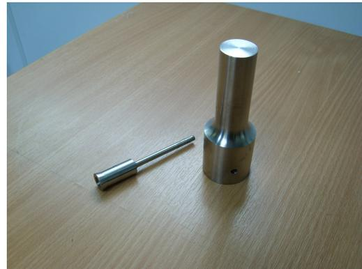
Fig: A3.10. Low and High powered piezoelectric transducer.
