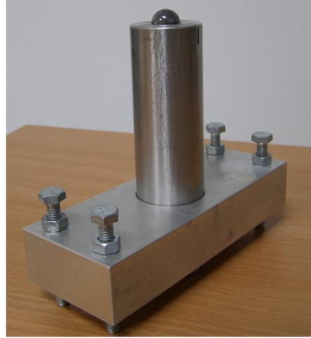
Fig: A3.11. Specimen holders' for cavitation experiments.
