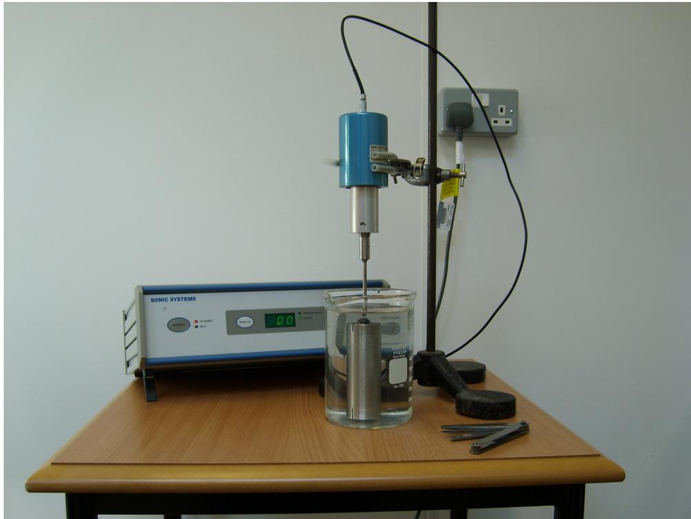
Fig: A3.8. Cavitation erosion test setup.
