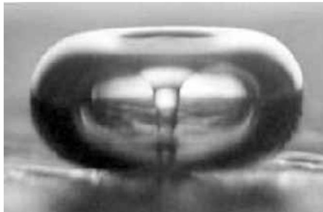
Fig: 1.5. A classic photograph by Crum showing micro jet development during bubble collapse. Bubble diameter approx. 1mm (Crum 1996)
