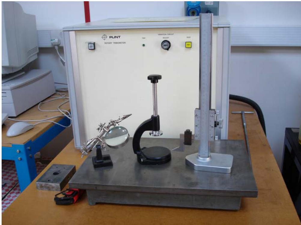
Fig: A3.14. Crack positioning for RCF experiments.
