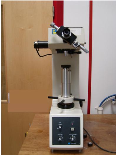
Fig: A3.1 Buehler Vickers Indent generating device
