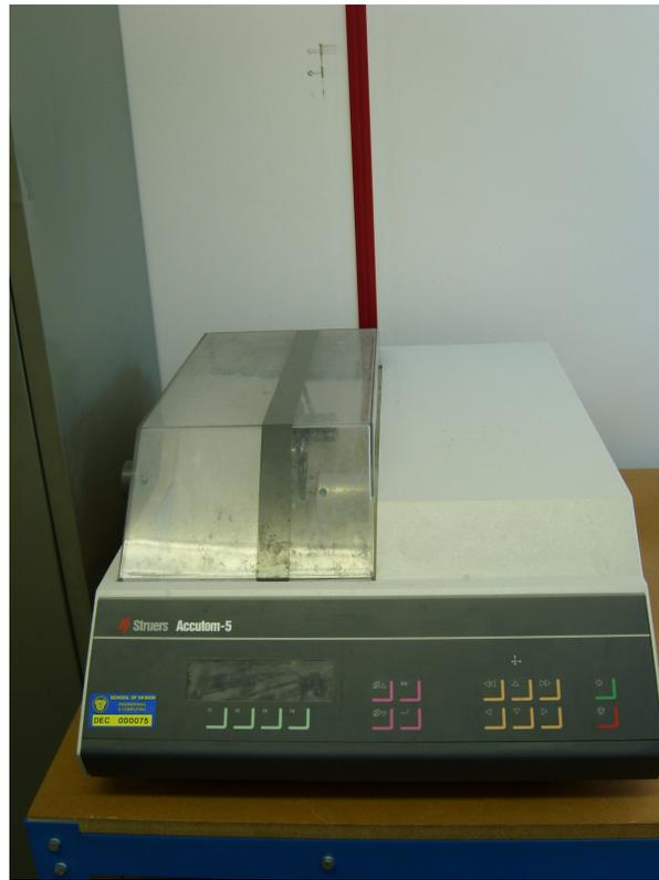
Fig: A3.12. Cutting machine for specimen dicing.
