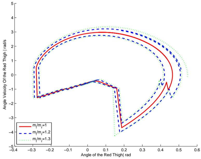
**Figure 6.28:** *Different Leg Mass Stable Gaits*
