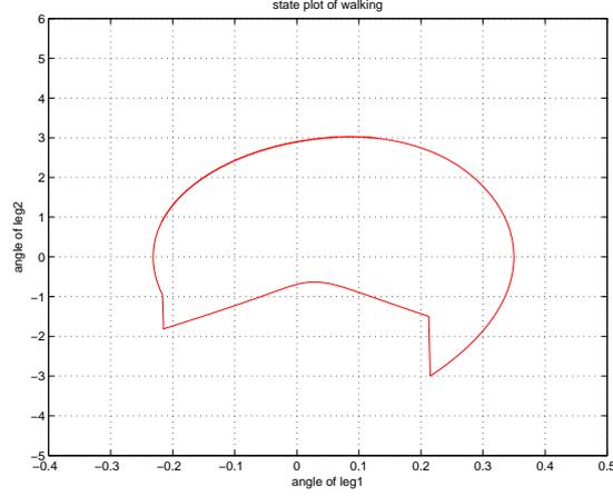
**Figure 8.4:** *the Limit Cycle of arc foot*
