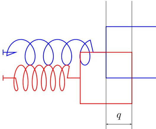
**Figure 1.7:** *the mass spring system*
