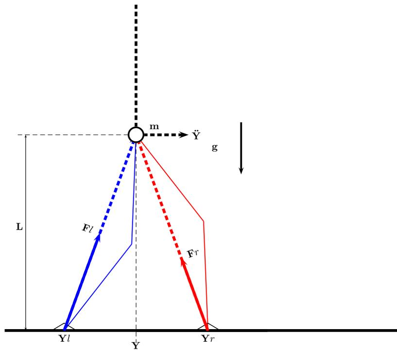
**Figure 7.1:** *The Stance Motion Primitives*
