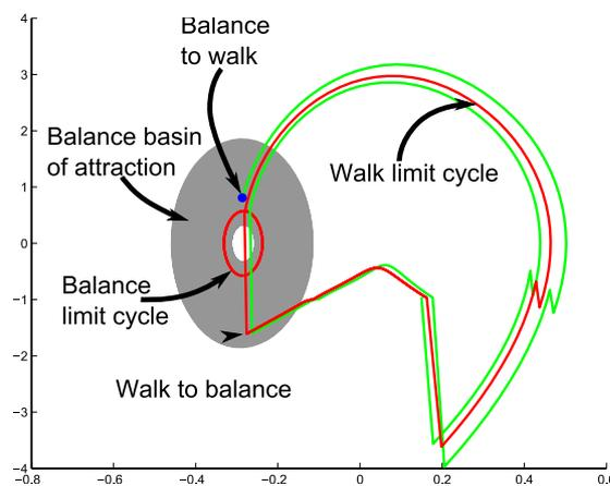
**Figure 7.13:** *The Phase Plot for Stance to Walk*
