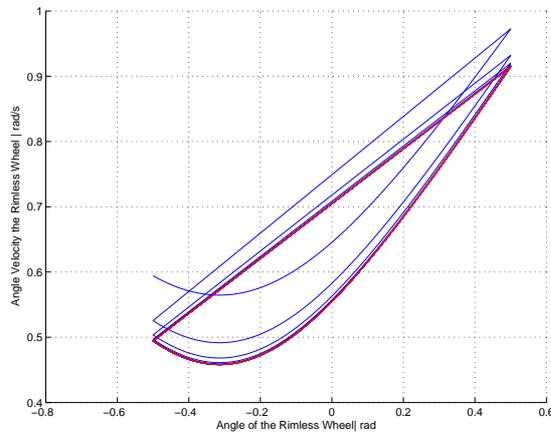
**Figure 1.10:** *The Limit Cycle of The Rimless Wheel*
