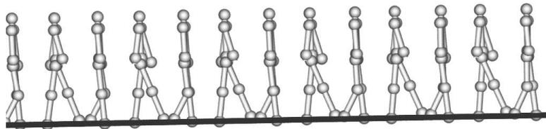
**Figure 6.36:** *Up slope Gait Generate by Lie Group offset Action*
