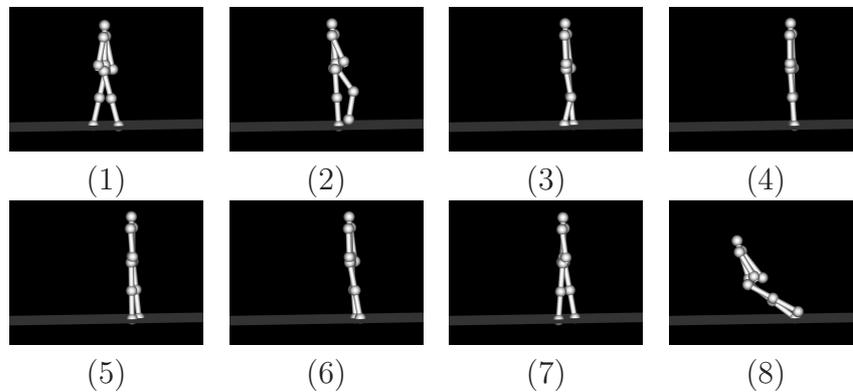
**Figure 6.34:** *Failure of walking upslope*
