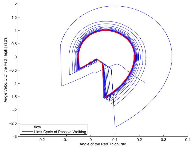
**Figure 6.11:** *Limit Cycle of entrainment gait on plane*
