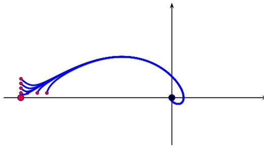
**Figure 1.5:** *Global Properties of the Flows: All the curves start from the repelling posture (Red) and end at the attractive one(Blue)*
