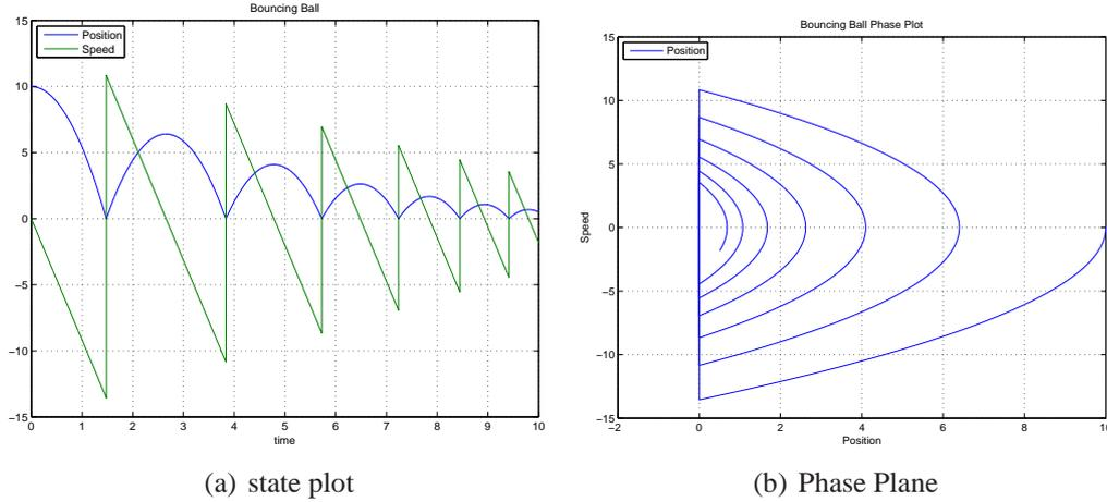
**Figure 3.10:** *Original Bouncing Ball System*
