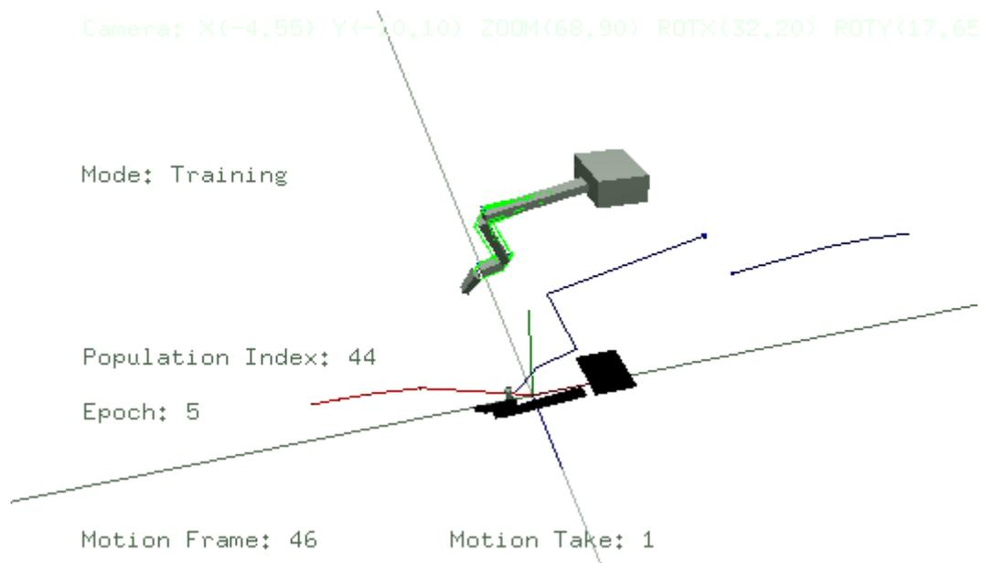
Figure 6.22: An example of constraint violation when the rigid body segment bends in an unnatural manner.
