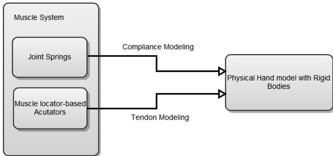
Figure 4.9: Schematic of the combinatorial muscle system in the physics engine.
