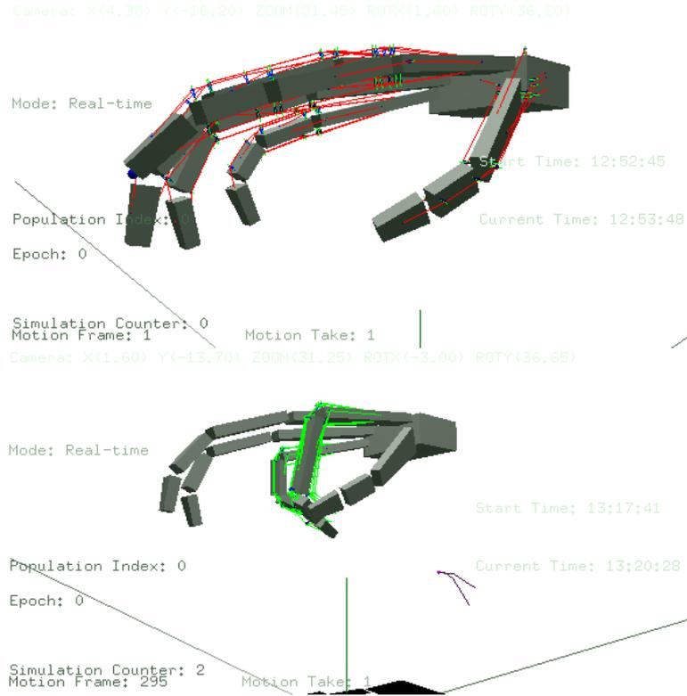
Figure 6.10: The fully dynamic rigid body hand model with the muscles laid out for each finger (top) and the forefinger and the little finger executing a motion (bottom).
