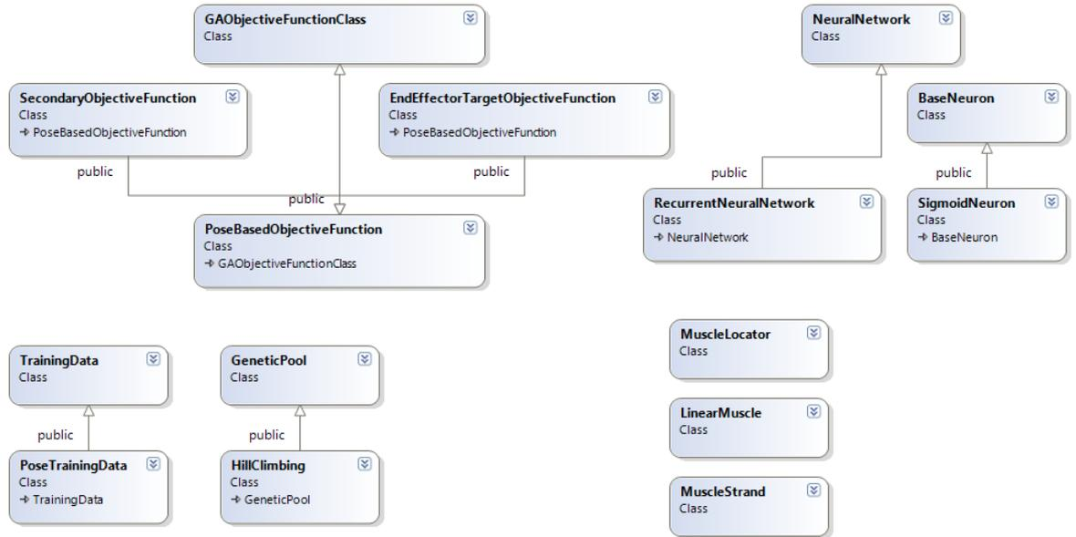
Figure 4.18: Class diagram of the various object classes in the virtual motor control system.
