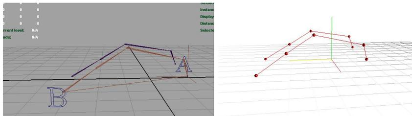
Figure 5.12: The two sets of linkage chains (Maya joint tool) created in Maya. The brown coloured linkage labelled B is the source chain and the chain labelled A is the target chain. On the right, the same two chains are exported from Maya into the external application, which performs the comparison test. Both links are proportionally same and maintain the same pose.
