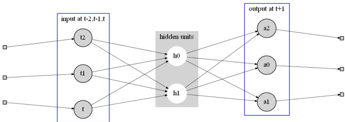
Figure 5.7: Vectors at three preceding time steps are fed into the network. The output is an extrapolated value for time  $t+1$ .
