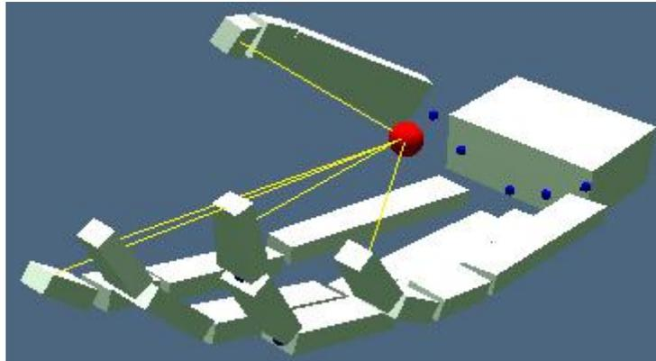
Figure 6.4: Action line convergence point (red sphere), a guide for lines of force.
