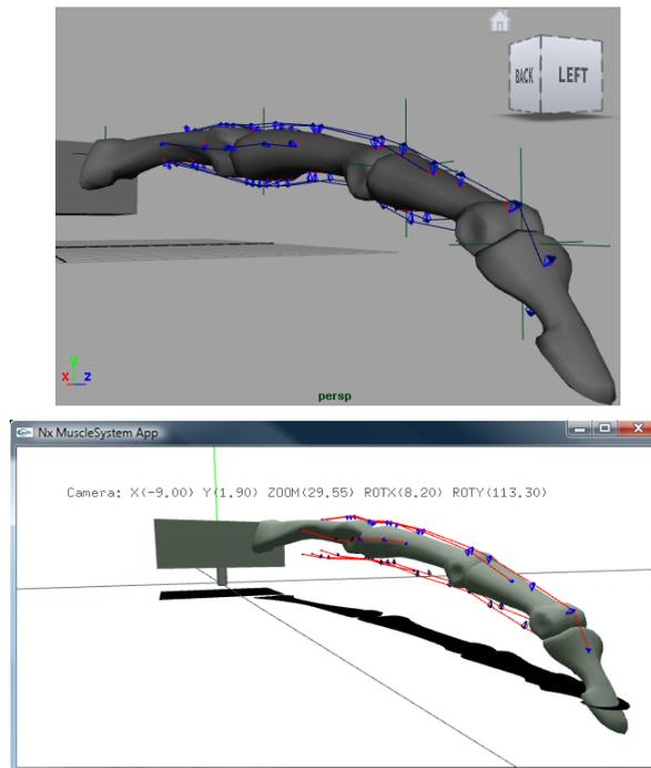
Figure 6.6: The images show the muscle rig laid out in Maya (top) and the dynamic muscle system created in PhysX (below) using the rig information. Extensor, flexor, abductor and adductor muscles are added.
