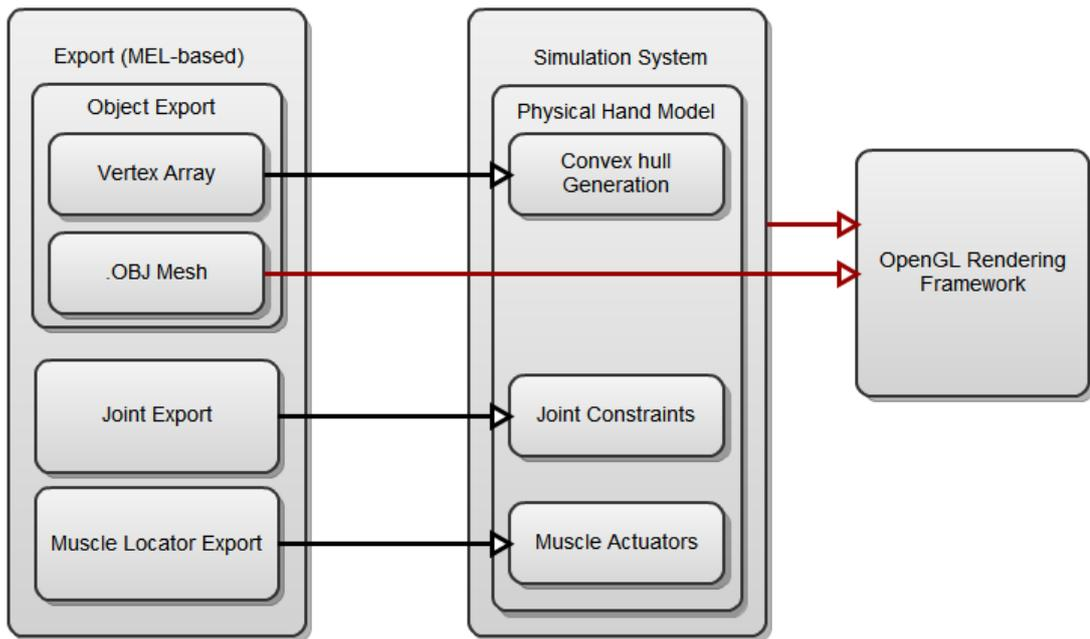
Figure 4.22: Schematic that shows the export system and how it ties in with the simulation and rendering framework.
