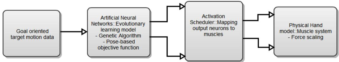
Figure 4.17: Control flow schematic of the neural motor controller
