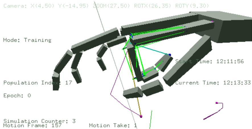
Figure 5.5: The cyan line from the end of the finger to the MCP joint is the end effector vector of the dynamic motion generated and the brown line is the end effector vector of the motion sample superimposed. The orientation of these two vectors provides an indication of differing poses in the input and output.
