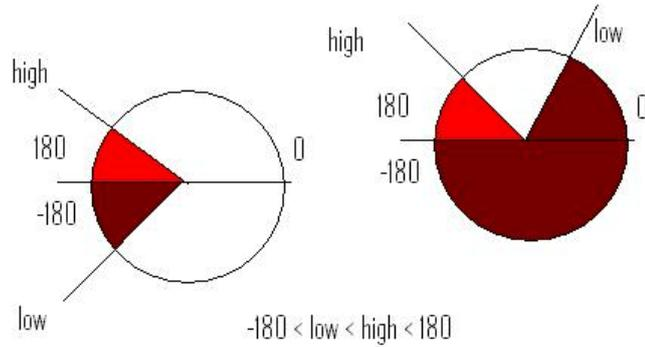
Figure 4.5: Revolute joint limit schematic (Ageia, 2006)
