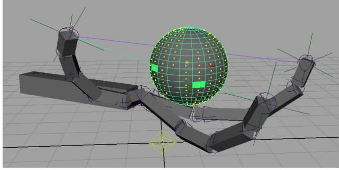
Figure 6.5: Screen capture of the Maya plug-in implementation of contact determination, using a three-fingered gripper. The highlighted green patches on the sphere show possible contact points along the action line.
