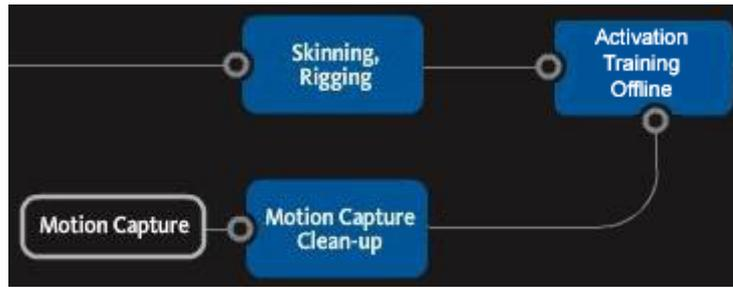
Figure 6: Modified segment of the games pipeline from Figure 3. The activation training is an offline process not directly a part of the pipeline. But existing pipeline processes are used for the training..
