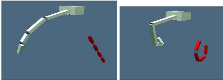
Figure 6.2: The dynamic finger (in white) is equipped with PD controllers on each joint while the linkage (in red) has a line of action force actuator. Both are controlled using the XBox360 gaming controller providing continuous control.
