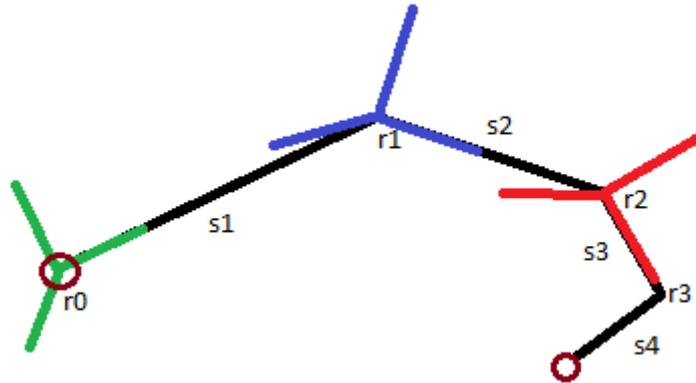
Figure 5.6: The local coordinate axes for each segment root are shown in red, blue and green. The segments are s1, s2, s3 and s4 and the roots are denoted by r0, r1, r2 and r3.
