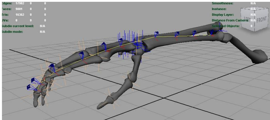
Figure 4.14: The skeletal hand model with joint locators, muscle locators (blue) and the resulting musculo-tendon unit that extends from the distal phalanx of the forefinger down to the arm bone (yellow). The joint locators are in orange and blue, between the bones of the phalanges and between the carpal bones at the wrist. The blue coloured joint locators represent fixed joints with zero DoF and the orange joint locators represent revolute joints with single DoF.
