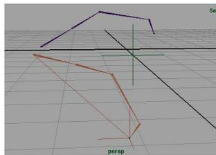
Figure 5.3: In global space, both linkages are different. And yet, in the local space of the parent link, they have the same pose.
