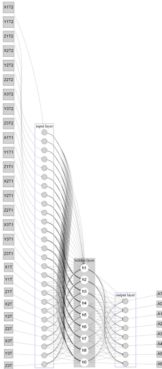
Figure 5.8: The fully connected time series predictor artificial neural network. The input is the pose vector of the forefinger at time states  $t - 2$ ,  $t - 1$  and  $t$ , which is an input vector containing 27 elements. In this particular network, there are 9 hidden nodes.  $A0..A7$  are the activations for the eight simulated muscles of the forefinger.
