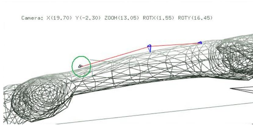
Figure 4.15: Due to the offset, the locator (encircled in green) appears to be floating above the bone surface mesh (shown in wire frame here). The offset places them on the convex hull (not shown here) that encompasses the mesh. The remaining two locators are also floating above the bone surface mesh, but the viewing angle makes it appear otherwise.
