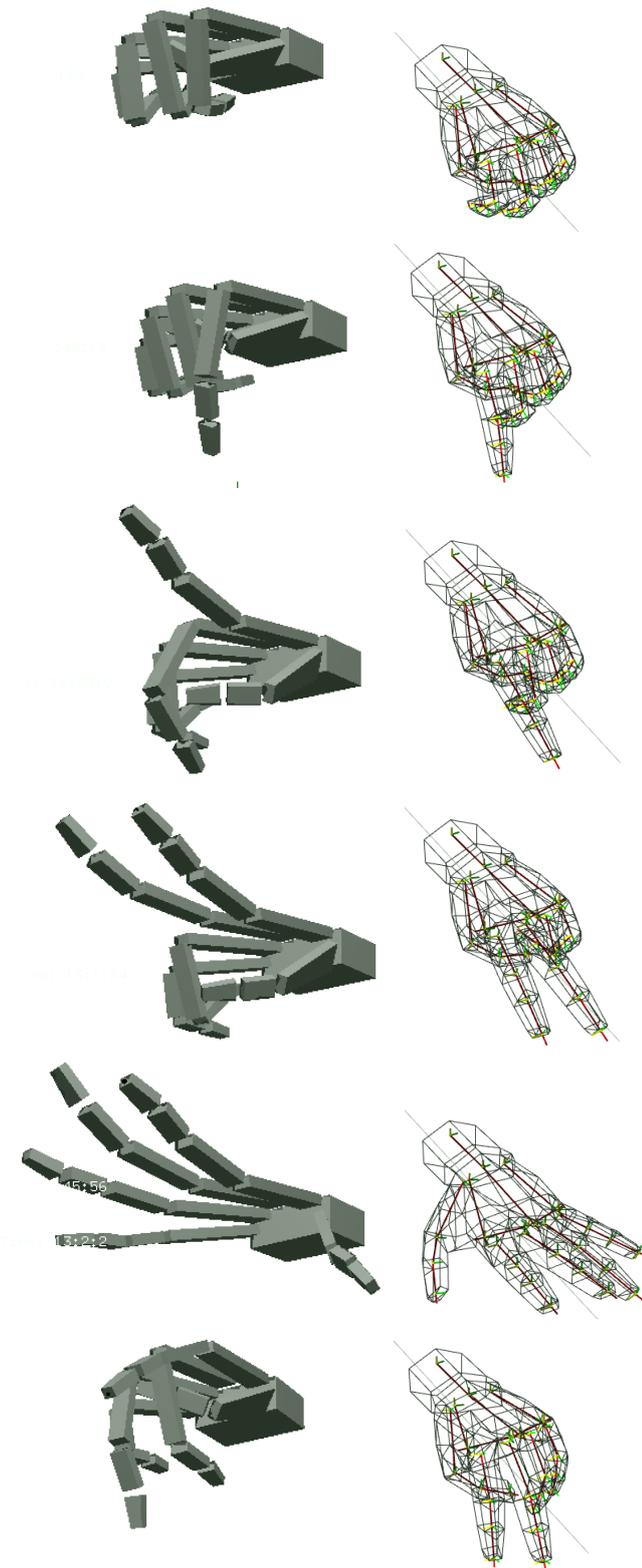
Figure 6.16: A few key frames captured from the generated animation. On the left is the physical hand model and on the right are the corresponding frames from the motion capture data.
