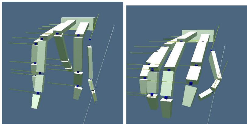
Figure 6.1: On the left, shows the effect of the absence of PD spring muscles. On the right, shows the effect of passive forces on the linkages from the joint springs functioning as muscles (PD). The pale green lines at the joints (blue boxes) denote the axis of rotation.
