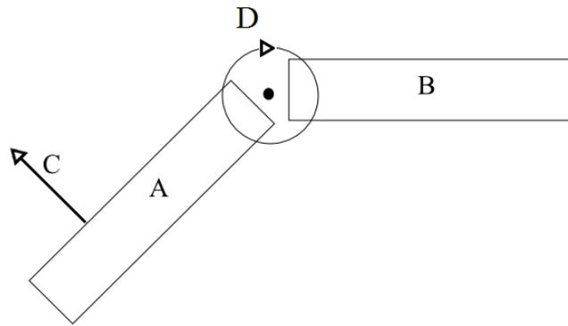
Figure 4.7: The angular force in the given direction D by the joint provides the required movement for the rigid link A to move in the direction C.
