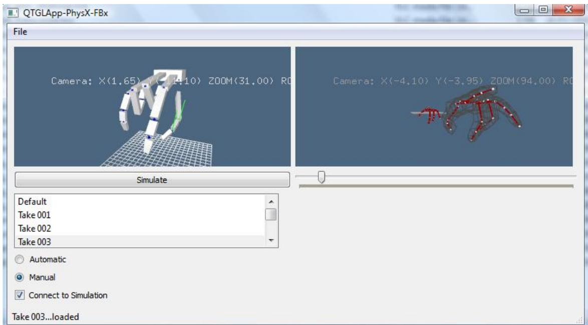
Figure 6.3: A Qt-based application and UI that demonstrates the PD controller. On the right window is the motion capture sample motion (with the animation takes listed in the list box below) and on the left is the simulated rigid body hand model with attached PD controllers at the joints.
