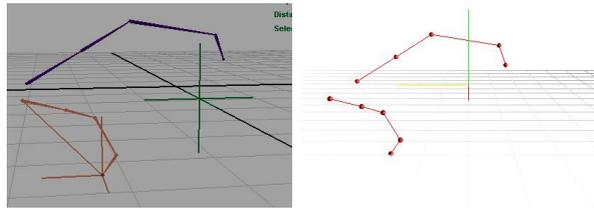
Figure 5.17: On the left Maya and on the right the output of the external application. The modified algorithm recognizes the pose even when the source links are in different proportions.
