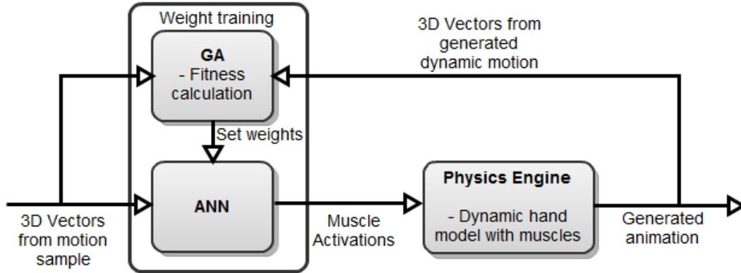
Figure 1.2: An architecture schematic showing the different frameworks and information flow between them.
