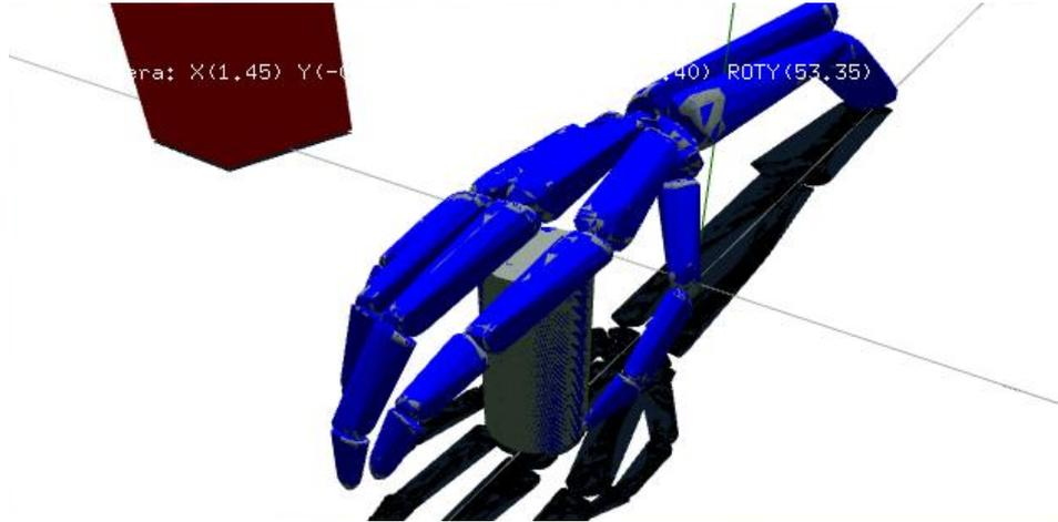
Figure 4.3: The convex hull rigid body overlay of the mesh model. The red cube is another PhysX rigid body. The cylinder is another convex hull rigid body placed for scale reference. The convex hull rigid bodies are the collision objects.
