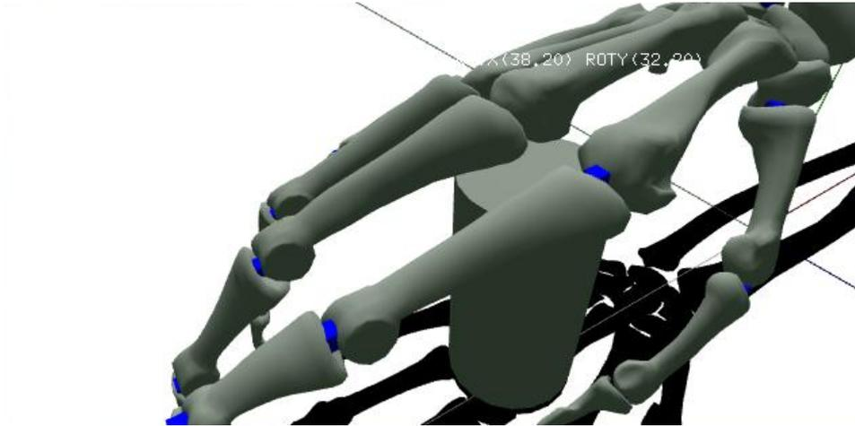
Figure 4.4: The blue cubes depict the joints between the rigid body bones in the hand.
