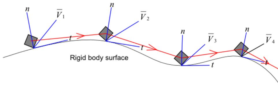
Figure 4.13: Muscle thin structure schematic showing specific contact points, force vectors and components. The grey boxes denote the muscle locators placed on the rigid body bone surface. The muscle locators define the tendon path along which the forces act.
