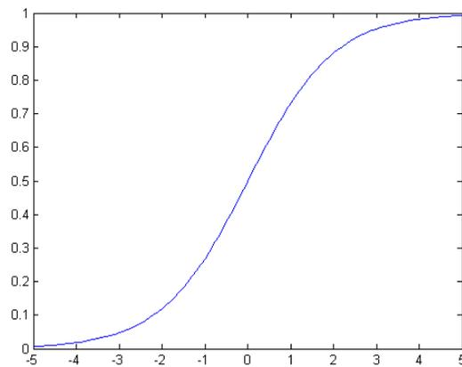
Figure 5.10: The continuous sigmoid function with output between 0 and 1.
