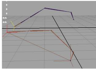
Figure 5.4: The hypothetical local basis vectors (in red and yellow), at the root nodes of the two linkages.
