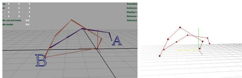
Figure 5.13: On the left, Maya scene and on the right the external application. The source chain is in a different pose from the target chain.
