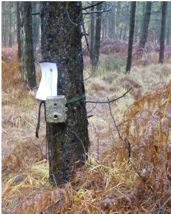
Figure A3-19. SPYPOINT IR-7 infrared motion detection cameras were secured to trees overlooking deposit sites.
