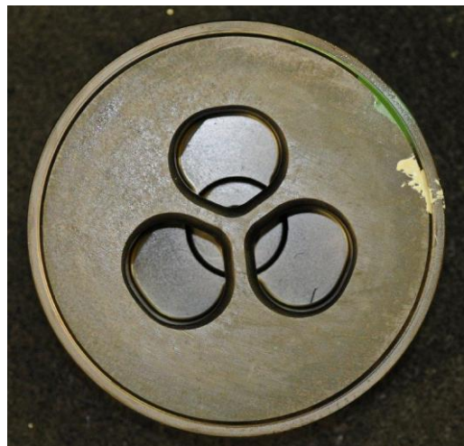
C and D: die consisting of two parts used for the Tube section
