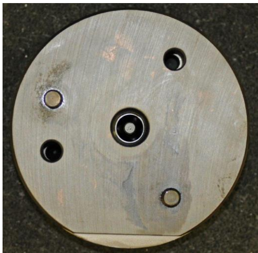
C and D: die consisting of two parts used for the Tube section
