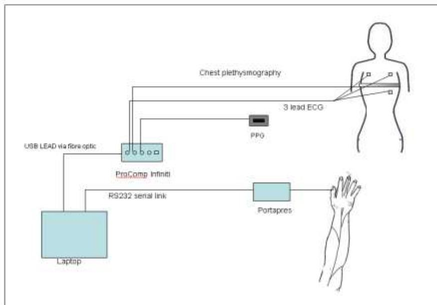
Figure 10 Schematic for Instrumentation showing connections between the patient and the equipment
