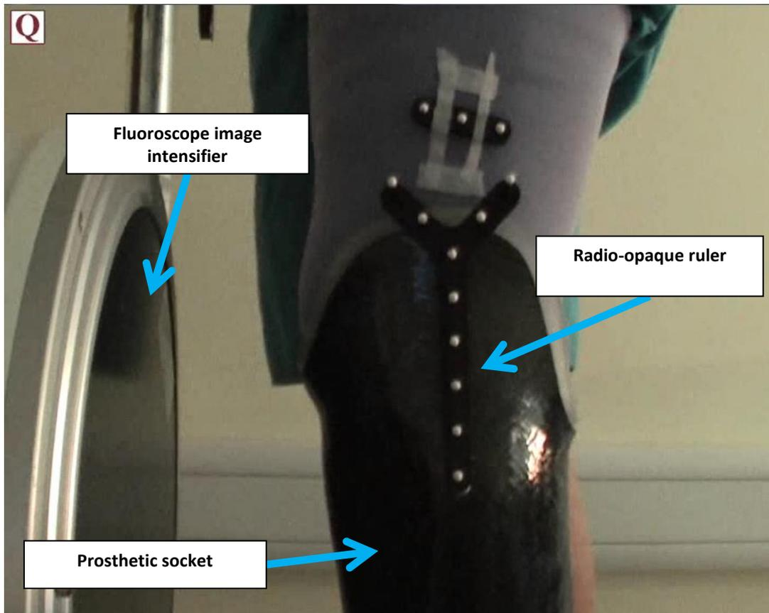
**Figure 45:** A radio-opaque ruler positioned on the lateral aspect of the participants prosthetic socket.
