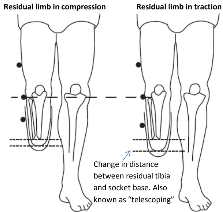
**Figure 11: Telescoping measurement gained by visualising and quantifying the movement of the residual bone within the socket.**
