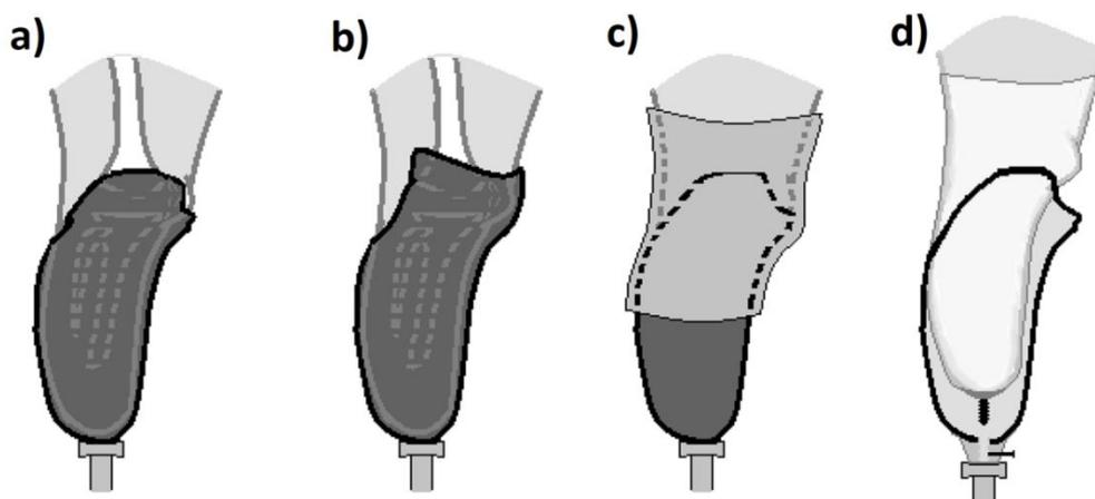
**Figure 9: Examples of socket suspension systems a) Supracondylar Brim b) Supracondylar Supra-patellar Brim c) Elastic Sleeve d) Silicone Liner.**
