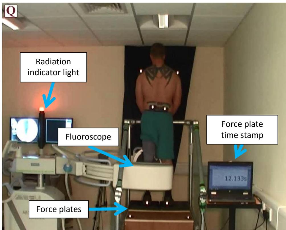
**Figure 43:** Depicting the stance of a unilateral trans-tibial amputee volunteer during residual limb imaging procedure.
