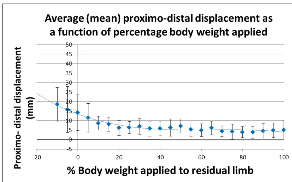
Figure 57: Average (mean) proximo-distal displacement across the population as a function of body weight applied at 5% intervals to the prosthetic limb. (n=12) A 3<sup>rd</sup> order polynomial is displayed on the graph as a trend line.
