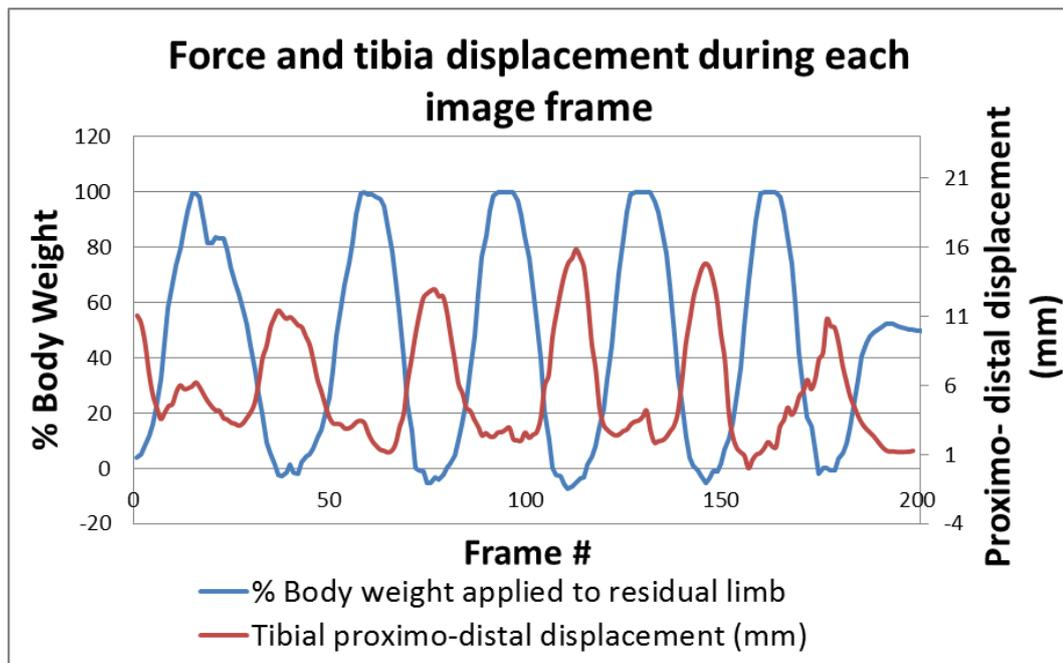
Figure 55: Recordings of participant #1's force distribution and tibial displacement over time while wearing a 5kg mass to simulate traction forces during the swing phase of gait.
