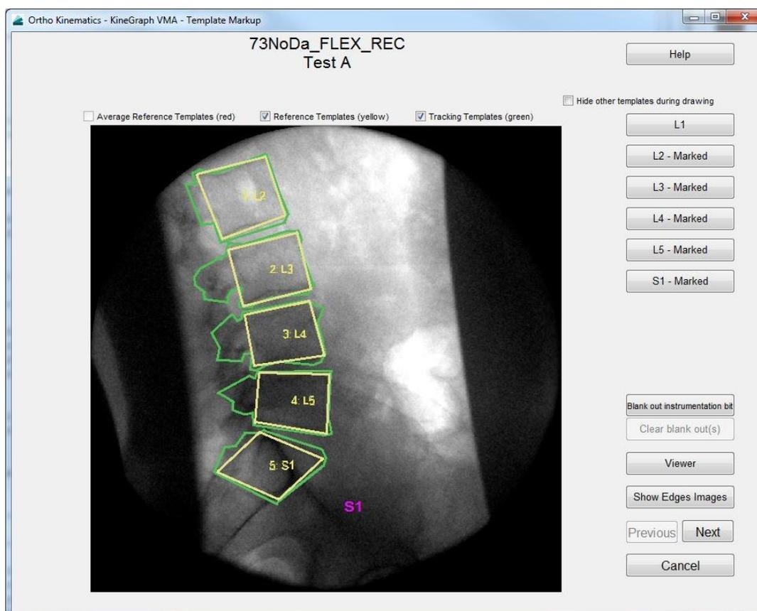
**Figure 22: Manual registration of vertebral body locations Graphic User Interface (GUI)**
