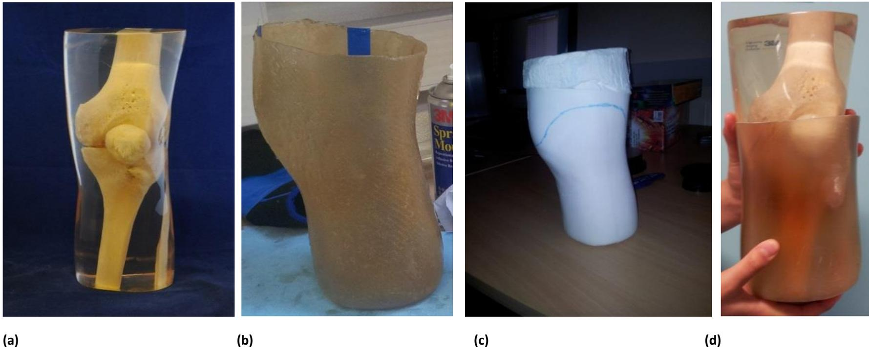
**Figure 35: Building of a prosthetic socket to contain a radiological phantom.**
