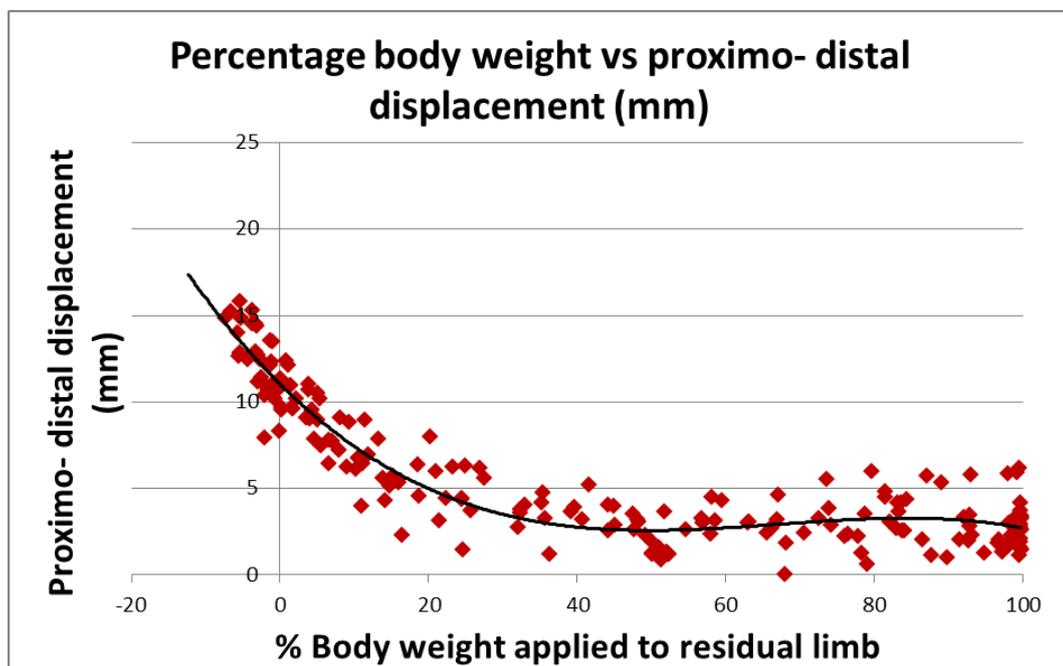
Figure 56: Recordings of participant #1's tibial displacement as a function of weight applied to the prosthetic limb while wearing a 5kg mass to simulate traction forces during the swing phase of gait.
