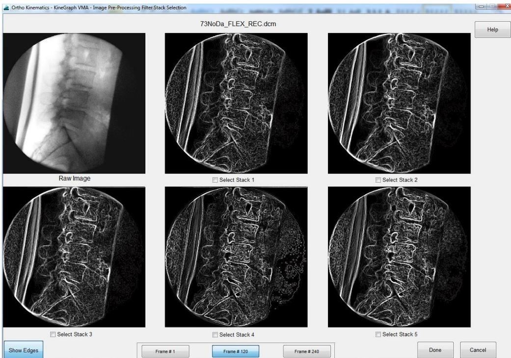
**Figure 21: Image enhancement Graphic User Interface (GUI)**
