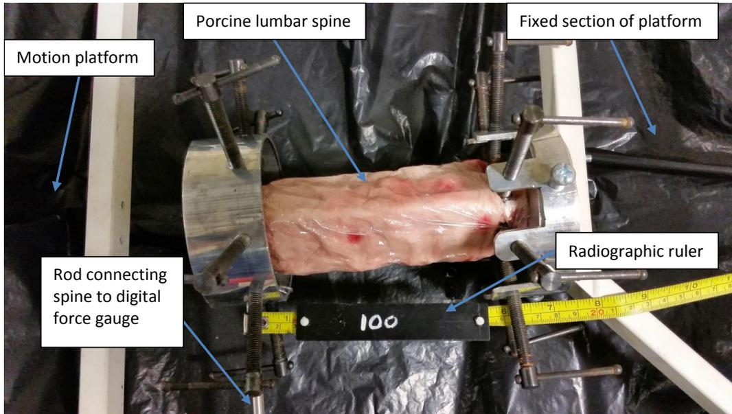
**Figure 38. Porcine lumbar spine testing apparatus and motion platform seen from above**
