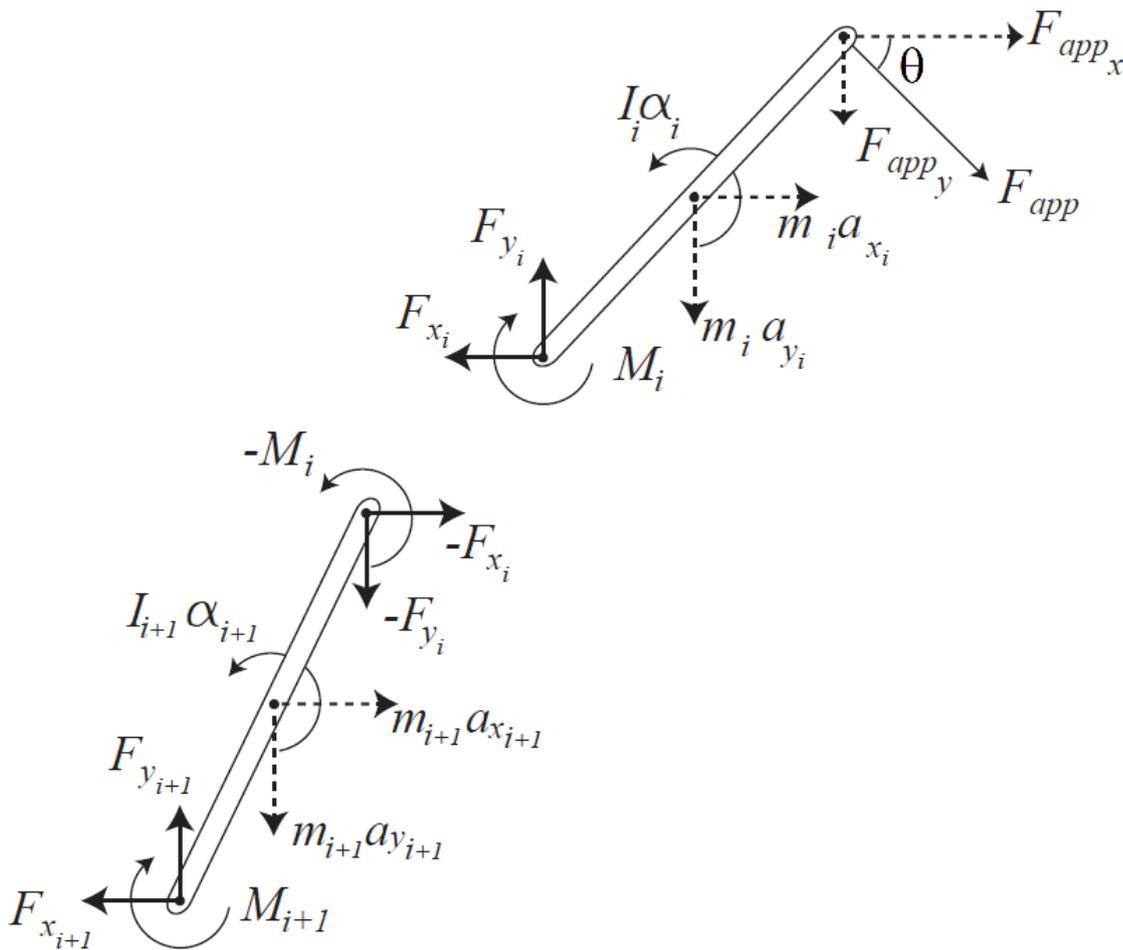
**Figure 40. A mechanical model of two successive vertebrae, modelled as having negligible thickness and uniform mass distribution. The figure shows action and reaction forces, net moments of force, and all linear and angular accelerations. Gravitational forces are ignored as they are not applicable in the plane of motion.**
