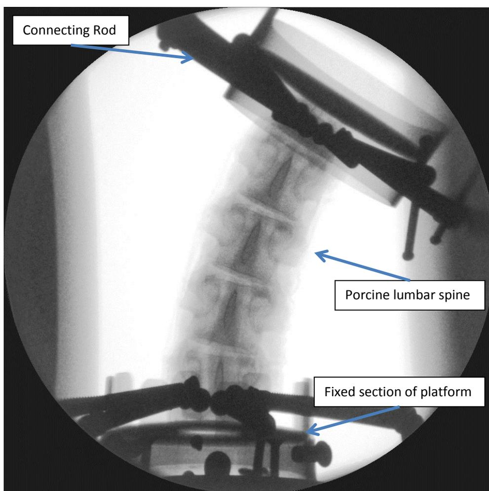
**Figure 39. Example of image acquired of porcine spine under motion (Left lateral flexion)**
