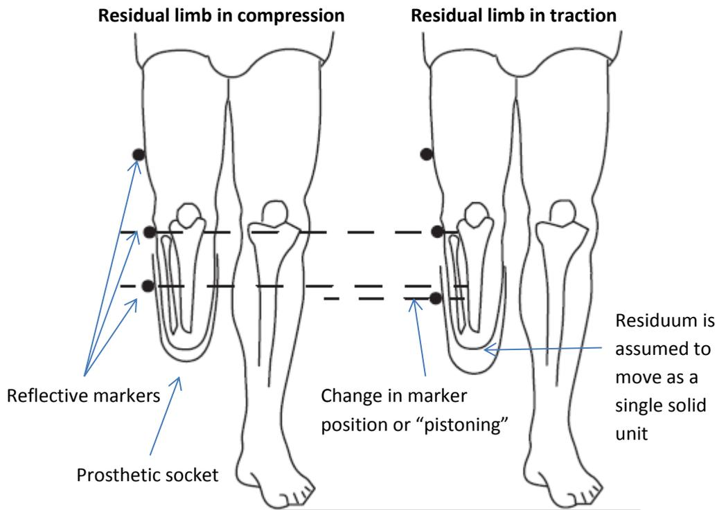
**Figure 10: Pistoning measurement gained by calculating the variations in distances between surface markers placed on the prosthesis and skin.**
