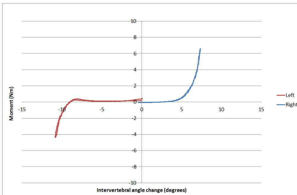
**Figure 41.** Example of a force deformation curve from an L3-4 motion segment undergoing left and right lateral flexion.
