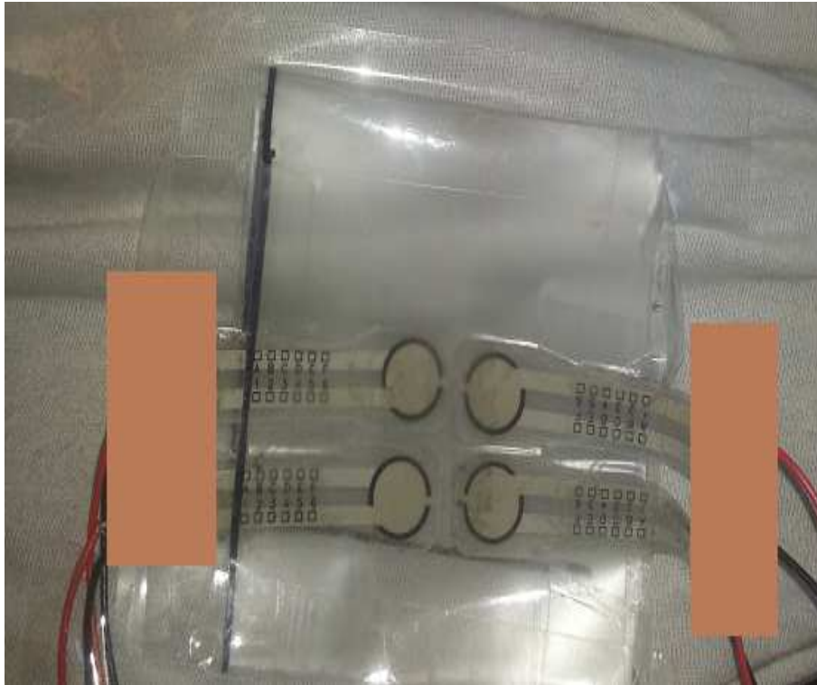
Fig. 6.7 Force sensor array to measure external load at bony areas
