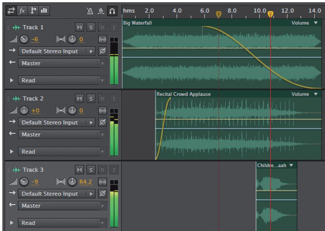
Figure 29. Audio tracks in Adobe Audition. Audio is represented as a container so that it can be repositioned along the time axis.
