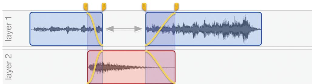
Figure 34. Inserting audio with a crossfade. The yellow line indicates gain adjustment.
