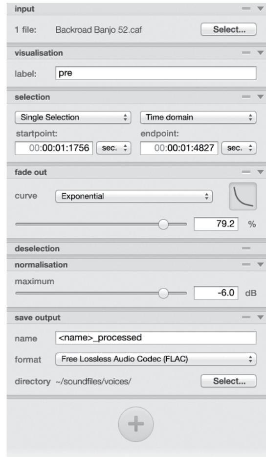
Figure 5. The editing chain, in which each edit is represented as a module.
