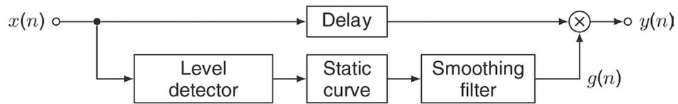
Figure 42. Compression is based on level detection (an envelope follower), a static curve to derive a gain factor from the result of the envelope follower, a smoothing filter to prevent too abrupt gain changes and a multiplier to weight the input signal (Zölzer 2008, p.213; 2011, p.100).
