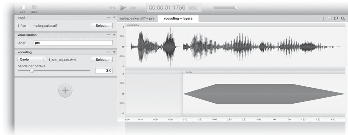
*Figure 51. Audio layers for vocoding. The modulator is the file we loaded, displayed as the topmost waveform. The carrier is a secondary input source loaded through the vocoding module and is displayed beneath the modulator waveform.*
