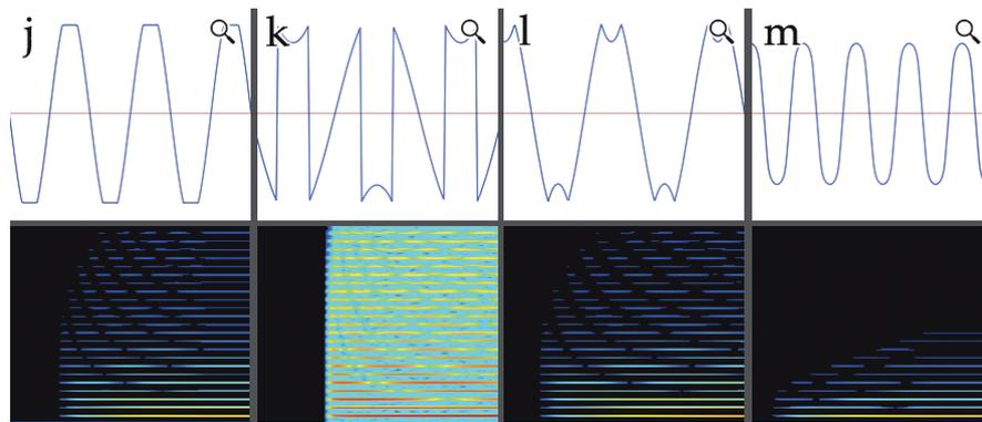
Figure 17. j) A sine wave getting louder than maximum, being clipped. k, l, m) A sine wave getting louder than maximum, respectively being wrapped, folded and soft-clipped.
