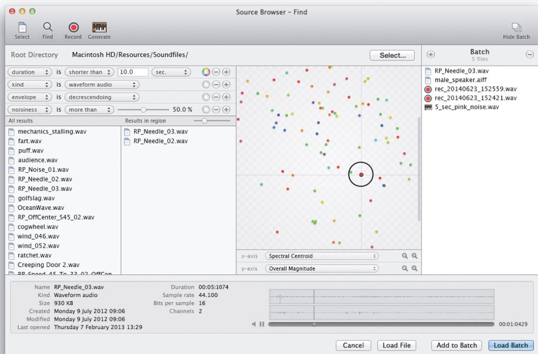
Figure 11. The *Source Browser* allows one to find an audio file not by name but by audible characteristics.
