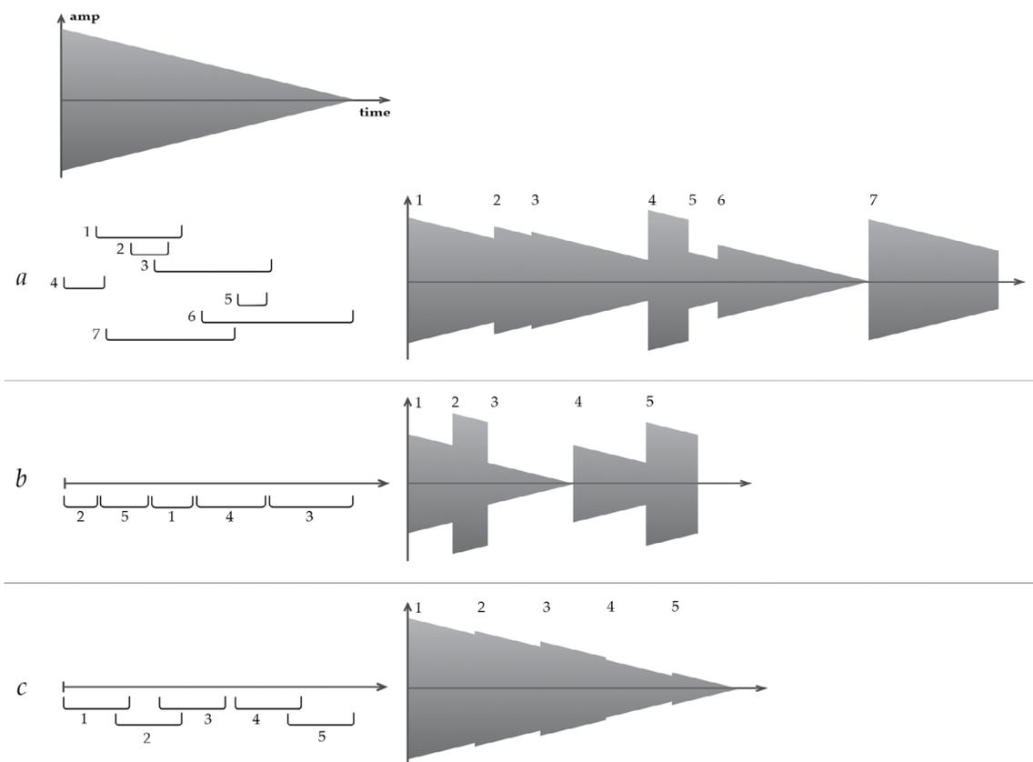
Figure 26. Random cutting (a), shredding (b) and one form of brassage (c). Random cutting: the segments have a random position and length, and can overlap. Shredding: similar, but no overlap. Brassage: overlap is allowed, but segments are sequential, which is characteristic for this technique. (Wishart 1994a, p.60)
