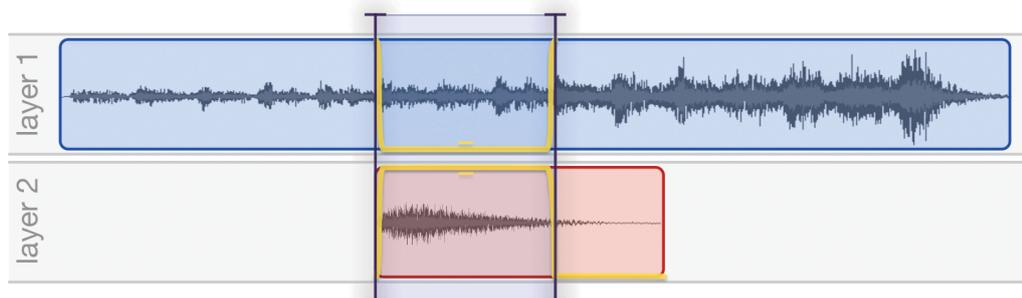
Figure 36. Replacing audio using layers. The gain of layer 1 is set to 0, while the gain of layer 2 is set to 1.
