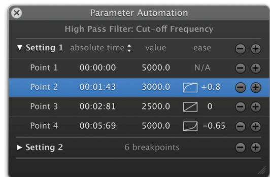
Figure 37. A head-up display for defining a parameter automation curve.
