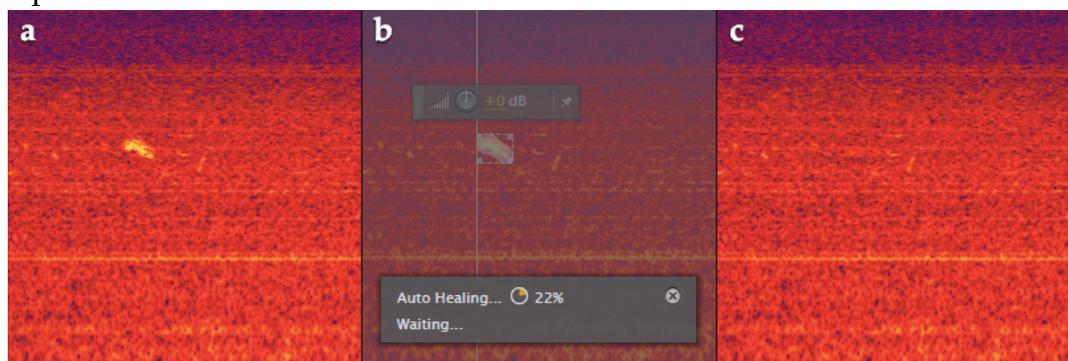
Figure 23. Spot healing in Adobe Audition. a) shows a small but audible noise element amidst background noise. Spot healing allows selection and automatic removal of this element, filling it up with similar background noise.
