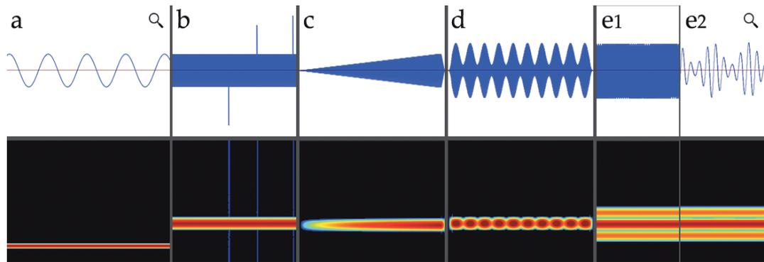
Figure 15. a) A steady-frequency 440Hz sine tone at fixed gain 0.3. b) Signal a, with spikes (1-sample ticks) added. c) Signal a, crescendoing linearly, from 0 gain to 0.3. d) Signal a, with a 5Hz tremolo (amplitude modulation) between 0.1 and 0.5 gain. e) Signal d, but with the modulation frequency at 100Hz.
