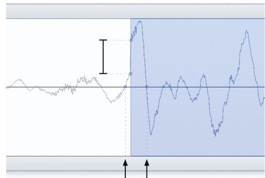
Figure 25. A gain change on a section that doesn't start at a zero-crossing (arrows) can result in a hard tick.
