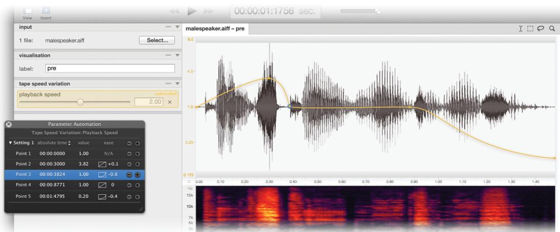
Figure 50. Parameter automation in OFFline. Here the playback speed is varied over time, as specified by the curve that is drawn over the waveform.
