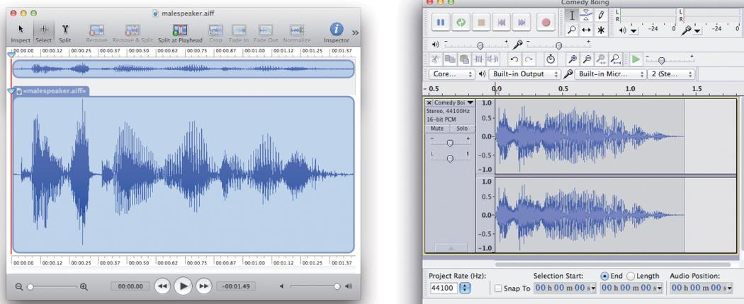
Figure 12. a) The waveform in Rogue Amoeba's Fission only shows positive and negative peak values. b) Audacity (by Roger Dannenberg) displays a waveform that shows both peak and RMS.
