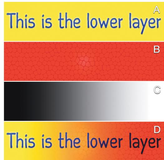
Figure 31. Layer B will be blended with layer A using multiplication. Mask C is applied to layer B before blending. The result of the blend is shown in D.
