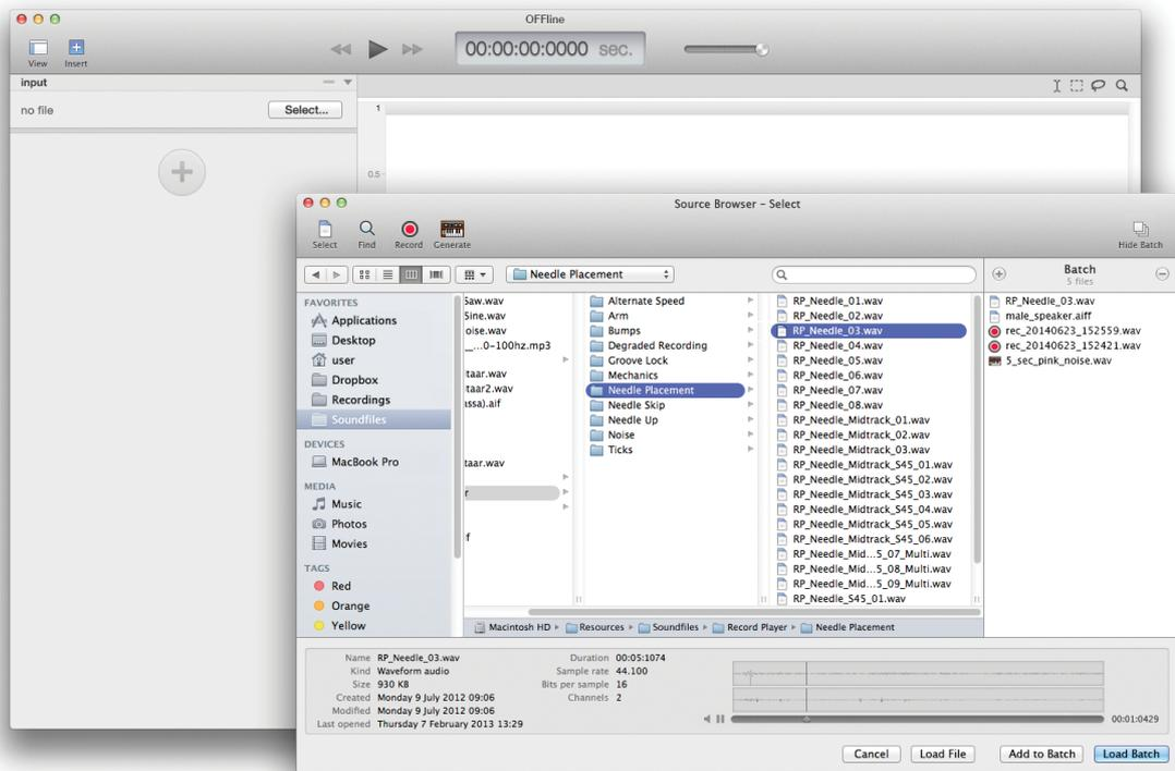
Figure 44. OFFline at launch. The module chain is empty except for an input module. The Source Browser is displayed to allow selecting one or more sources to load through this input module.
