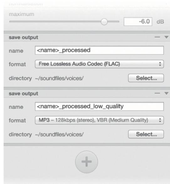
Figure 6. Multiple output modules allow simultaneous saving in different formats.
