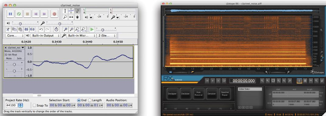
Figure 2a). A wave editor (Audacity) and b) a spectrum editor (iZotope RX)
