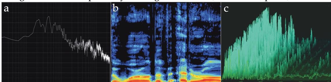
Figure 13. a) a line spectrum with frequency on the horizontal and magnitude on the vertical axis. b) a spectrogram with time on the horizontal and frequency on the vertical axis, using color to represent magnitude. c) a waterfall plot with frequency on the horizontal and magnitude on the vertical axis. Time is represented on the third axis.
