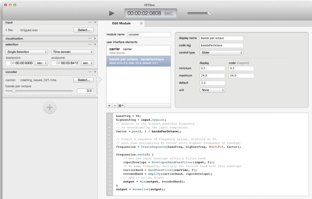
Figure 41. The module development environment in OFFline. A module can be created or edited through this interface. Parameters can be specified for the graphical user interface, and a code editor allows for programming the processing part of the module.
