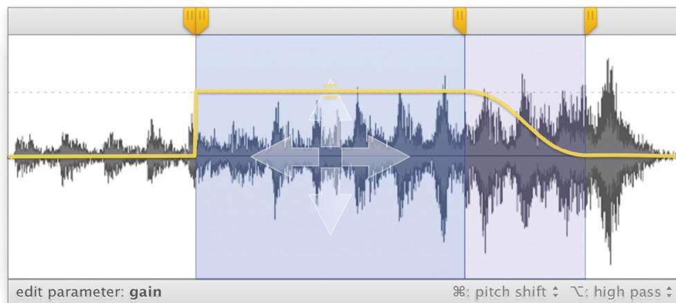
Figure 22. A waveform display that provides gain adjustment by dragging up or down. Other parameters can be adjusted using moderator keys (see bottom-right).
