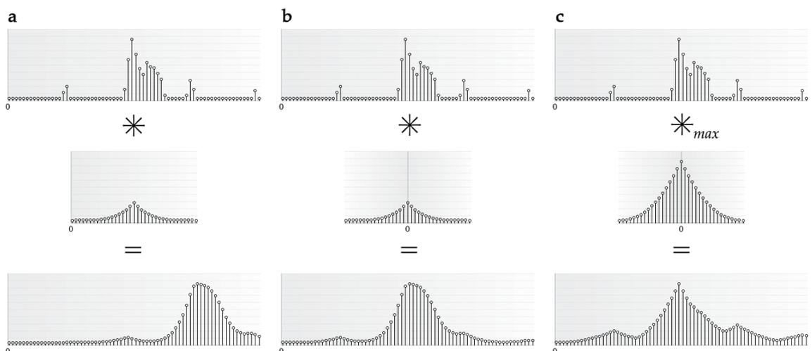
Figure 43. Three modes of convolution. a) shows regular convolution in which every value of the input (top) is multiplied with every value of the impulse response (middle). b) shifts the impulse response relative to the input sample, allowing the convoluted samples to occur before the input sample. c) doesn't add all convoluted samples but returns only the maximum convoluted sample values.
