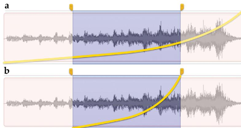
*Figure 38. a) A curve that spans the full length of the audio file. b) The same curve but applied relatively to the selected segment.*
