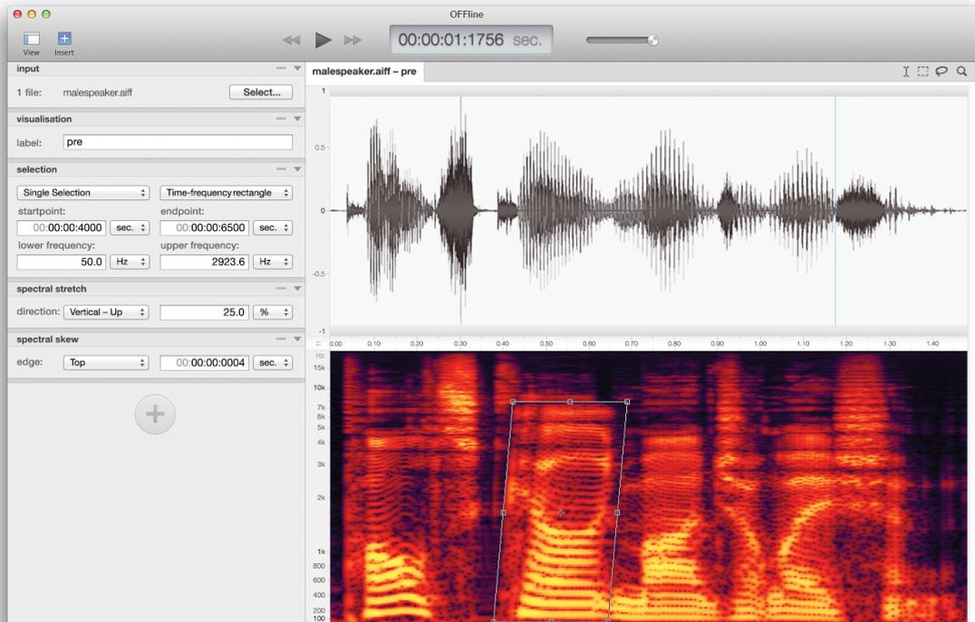
*Figure 48. Offline with a single audio file loaded. Both a waveform and a spectrogram are displayed, visualising the audio at a specific point in the editing chain (here right after the input module). A spectral edit is made through manipulating a spectral (time-frequency) selection.*
