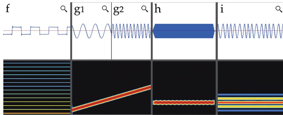
Figure 16. f) A square wave with fundamental frequency 440Hz and fixed gain of 0.3. g) A sine wave at 0.3 gain, going linearly from 220Hz to 880Hz. h) A sine wave with a 6Hz vibrato (frequency modulation) between 435 and 445Hz. i) A sine wave with a 100Hz frequency modulation between 340 and 540Hz.
