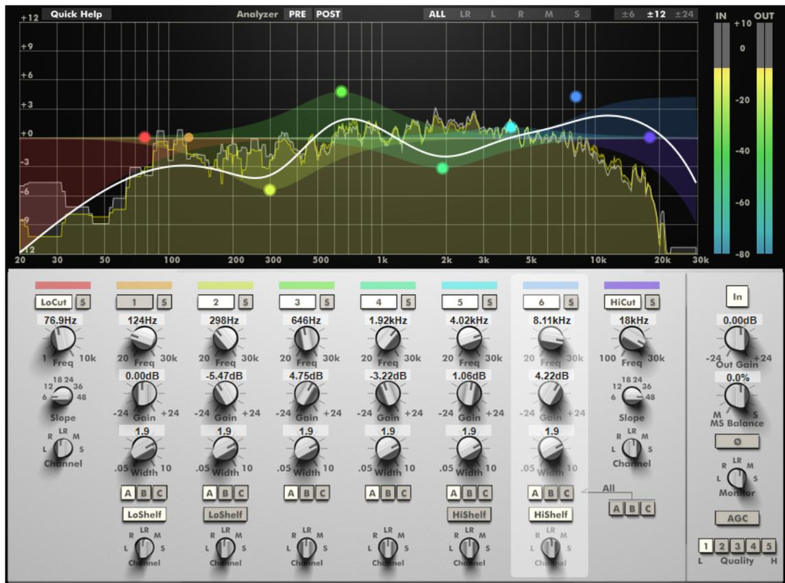
Figure 4. *TranQuilizr* is an equaliser plug-in by A.O.M., that (like many other equalizer plug-ins) offers both a graphical equalisation curve that can be edited by dragging anchor points, and a series of (very skeuomorphic) dials for more precise control over the curve components..
