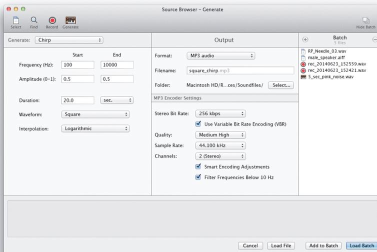
c) Generating an audio file using signal generators.
