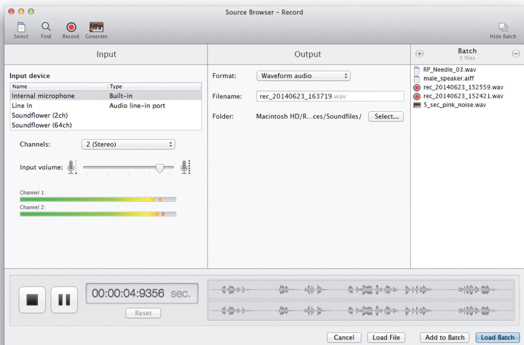
Figure 9. Recording in the Source Browser, allowing specification of input and output. A compact waveform display is provided below. New recordings can be added to the batch.
