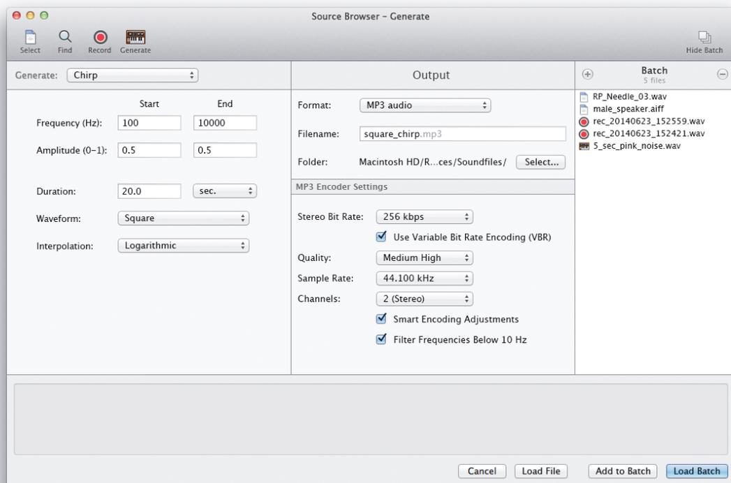
Figure 10. The *Source Browser* facilitates generation of audio sources using basic synthesis techniques.
