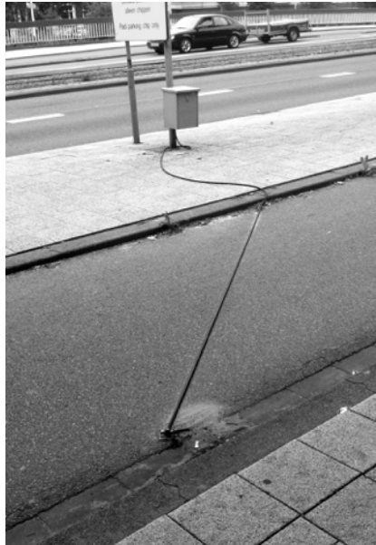
Fig. 34. Tubes placed on the surface of the road to evaluate traffic streams.
