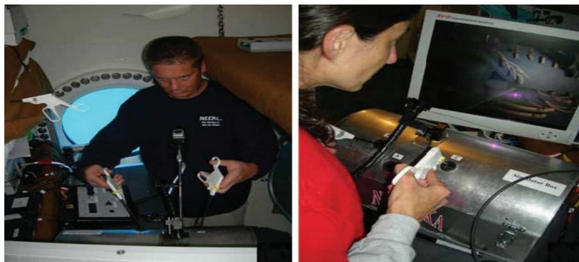
(d) Crew members of Aquarius underwater habitat performing surgical tasks with the assistance of a fixed base camera robot ( Fig. 2.1(a) ) and a mobile camera robot ( Fig. 2.2(b) ) [19]
