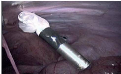
(a) Fixed base pan and tilt camera robot (tripod mounted) [15, 108] (b) Fixed base imaging device in abdominal cavity (suturing mounted) [106]
