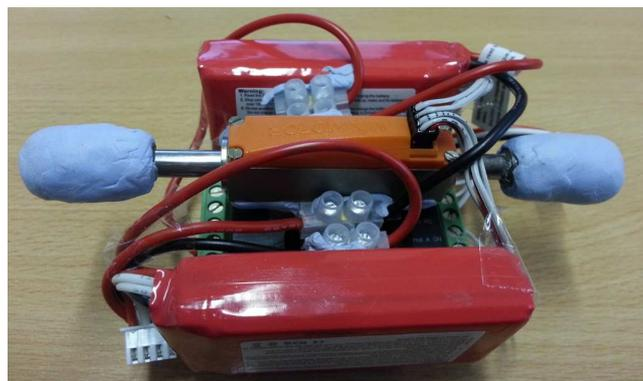
(c) Implemented Capsubot: Without capsubot-shell (Extra masses - blue tack - are added to the cylinder to increase IM to capsobot mass ratio)
