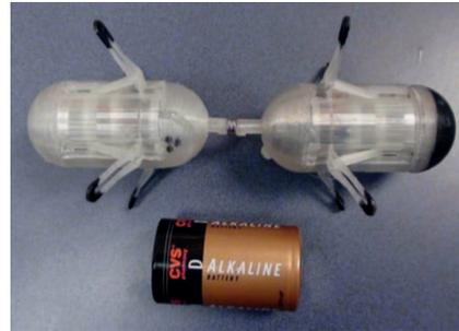
(b) Inchworm-like locomotion based modular robot [119]
