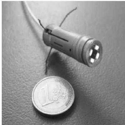
(a) SMA based four-legged robot [111]
