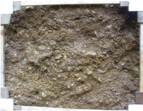
Figure A20.2 Photographs used for image-based automated grainsizing of HA1.1 (a), HA1.2 (b), and HA1.3 (c) and the resulting grain size distributions.
