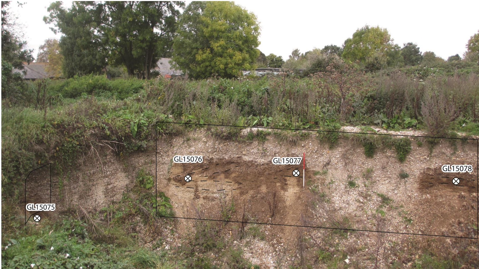
Figure A15.2 Annotated photograph of Bickton pit showing the OSL sample locations in the western and northern walls of the pit.
