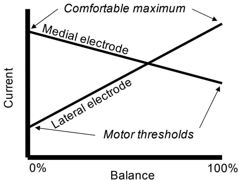
Figure 15: Example of how the current on two channels can be adjusted as a function of the balance parameter. The maximum and minimum currents for each channel are independent and set manually. The two channels can use a common reference electrode.
