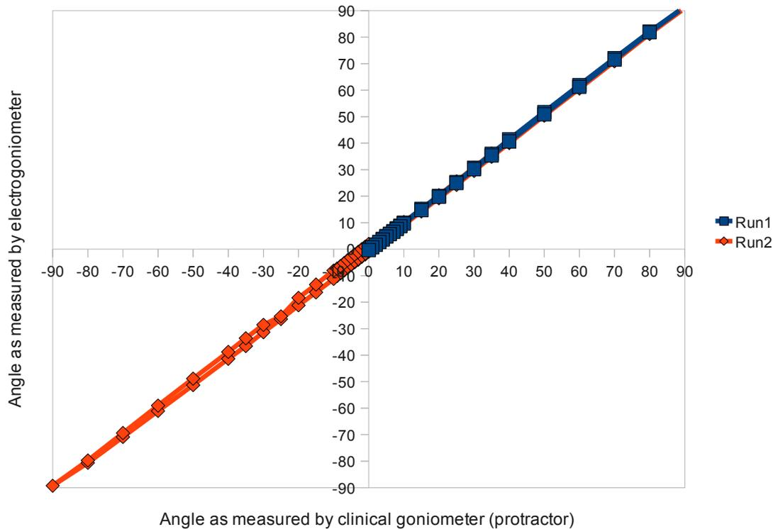
Figure 9: Calibration of the electrogoniometer
