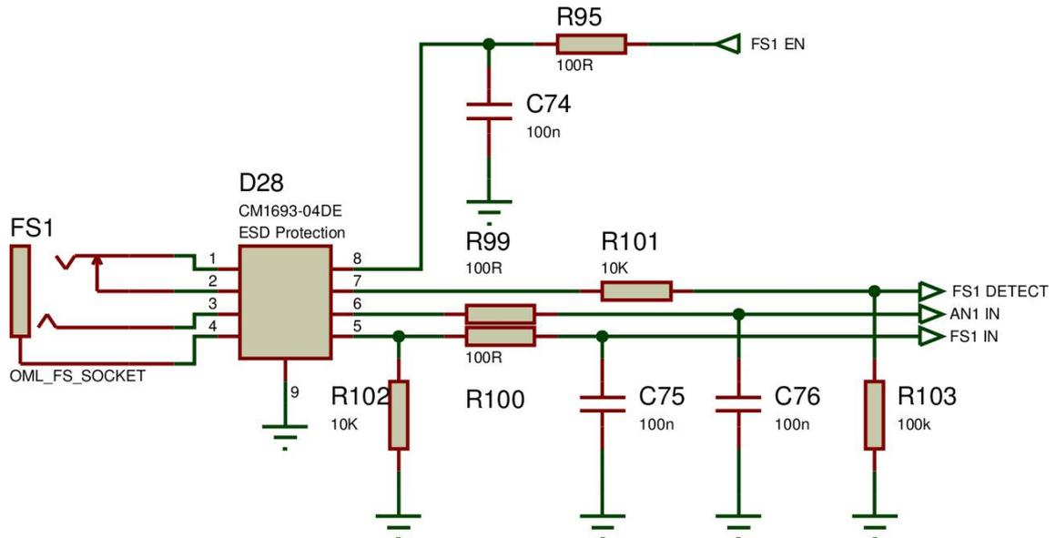
Figure 130: Foot switch input circuit. There are four of these per stimulator.
