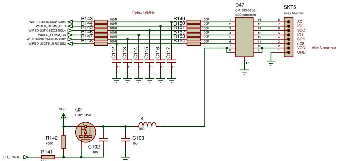
Figure 128: Non-isolated expansion port.
