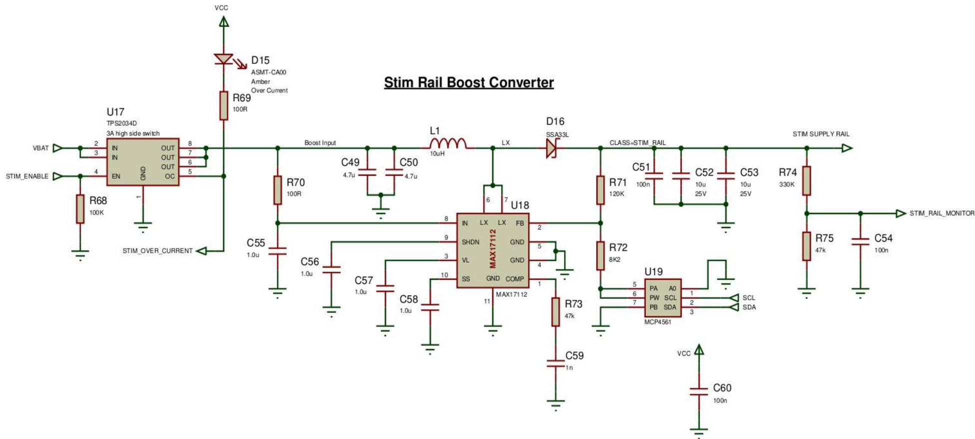
Figure 126: Boost converter supplying the stimulation output stages.
