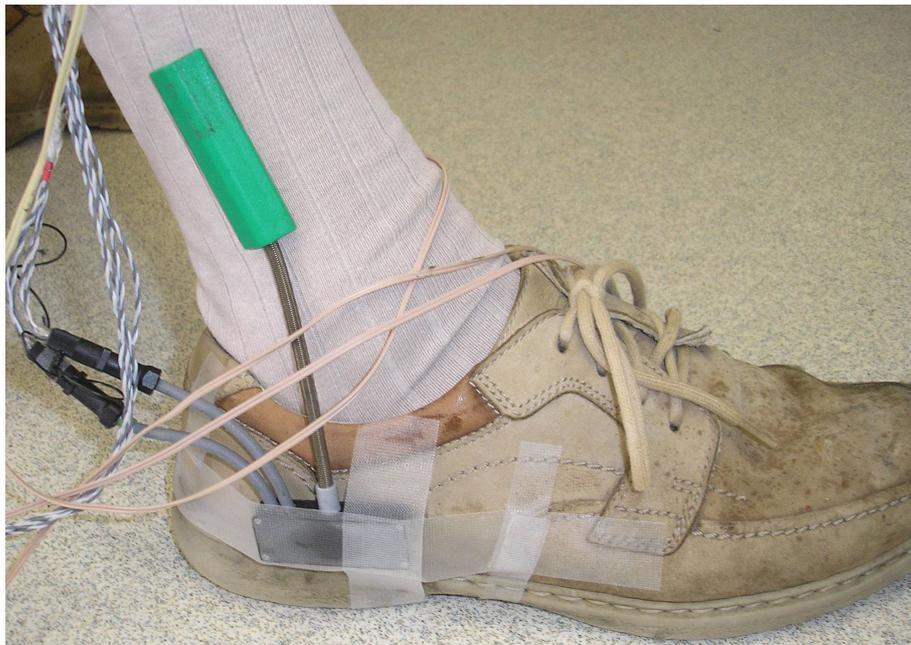
*Figure 16: Ankle goniometer in position*
