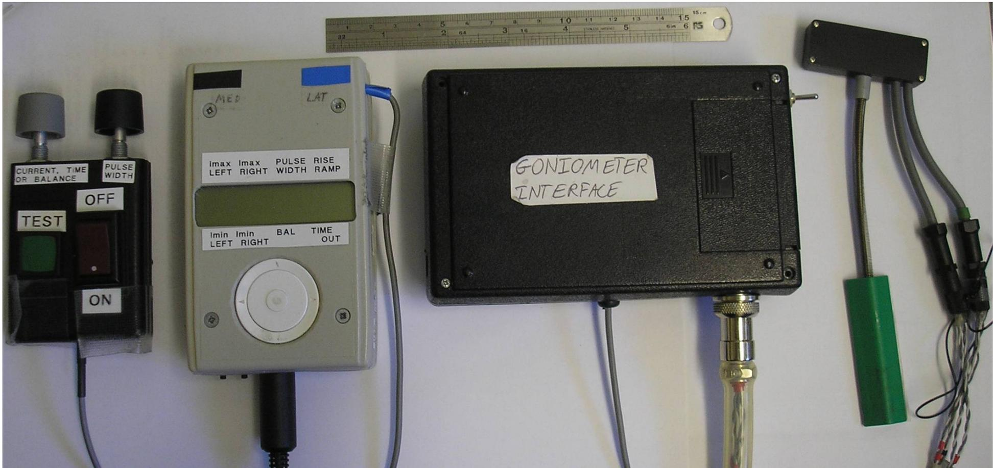
Figure 133: Experimental equipment: (left to right) Remote control, stimulator, goniometer interface, goniometer. The ruler above is 15cm long.
