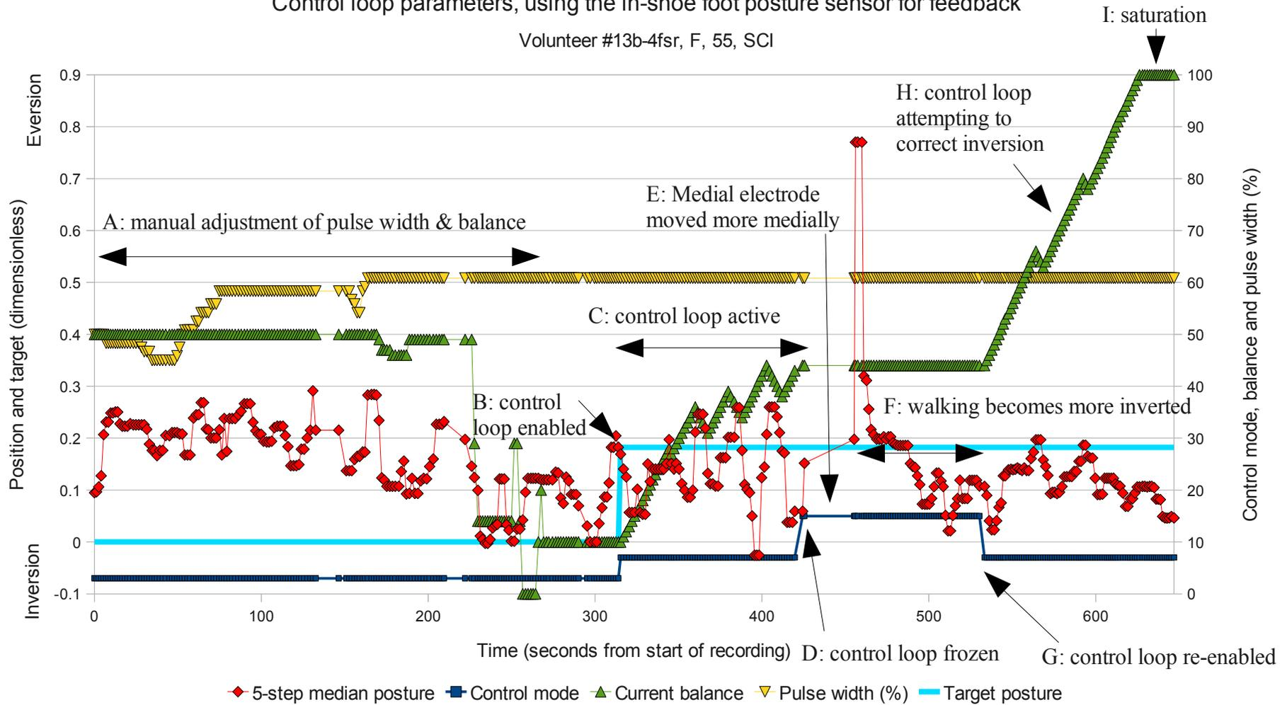
Figure 118: Closed loop control using the in-shoe foot posture sensor for feedback, volunteer 13.
