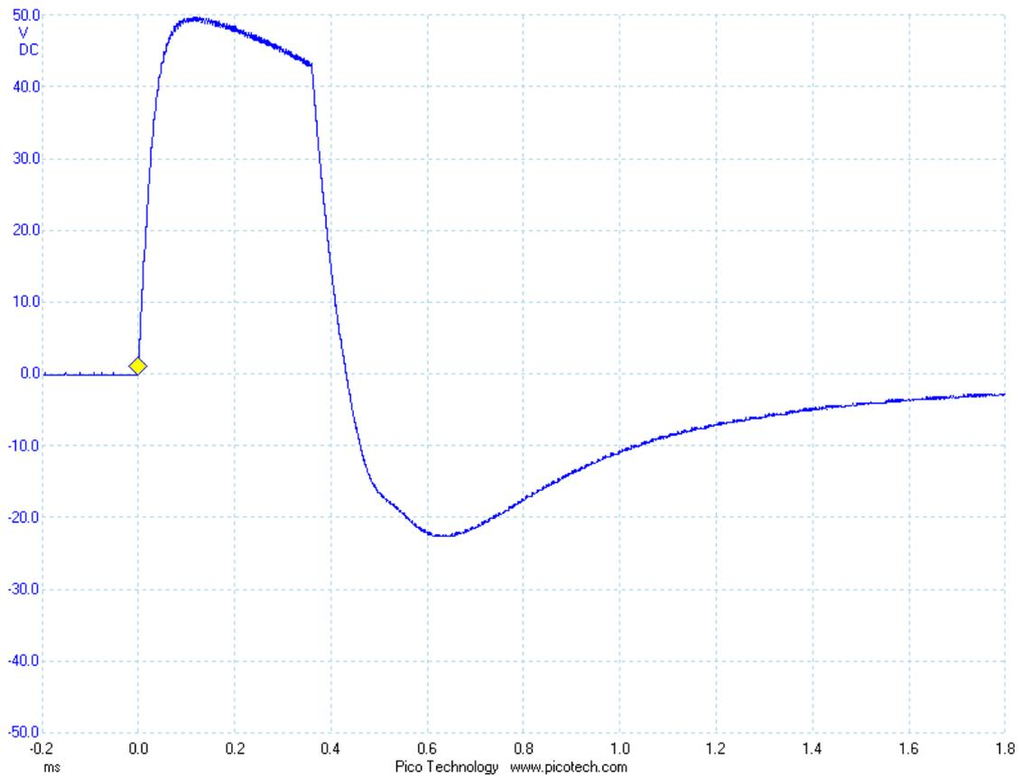
Figure 12: Typical output pulse waveform at 50mA into 1kΩ//100nF load. Axis units: abscissa: milliseconds; ordinate: Volts.
