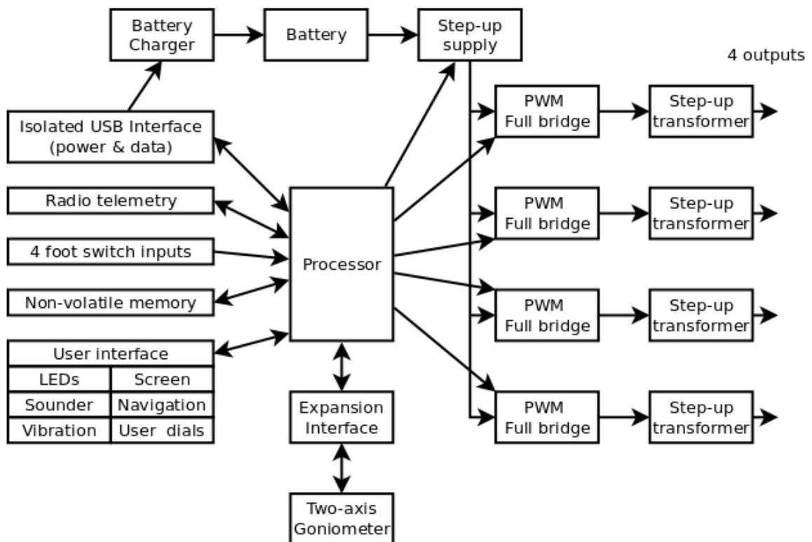
Figure 11: Block diagram of stimulator hardware
