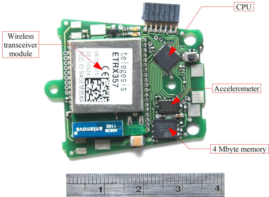
Figure 8: Circuit board for the in-shoe foot posture sensor.
