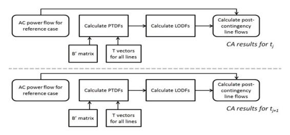
Figure 4: Algorithm flowchart for DC contingency analysis.
