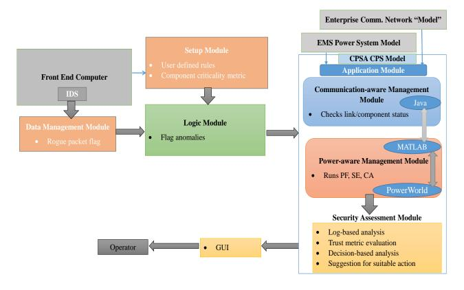
Figure 2: Overall CPSA system module.
