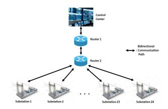
Figure 3: Topology for the communication network.
