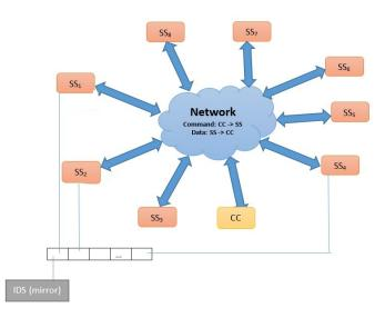
Figure 1: Overview of a cyber-physical power system that consists of eight substations (SS) connected to a control center (CC) over the wireless network and is monitored by a global state estimator.
