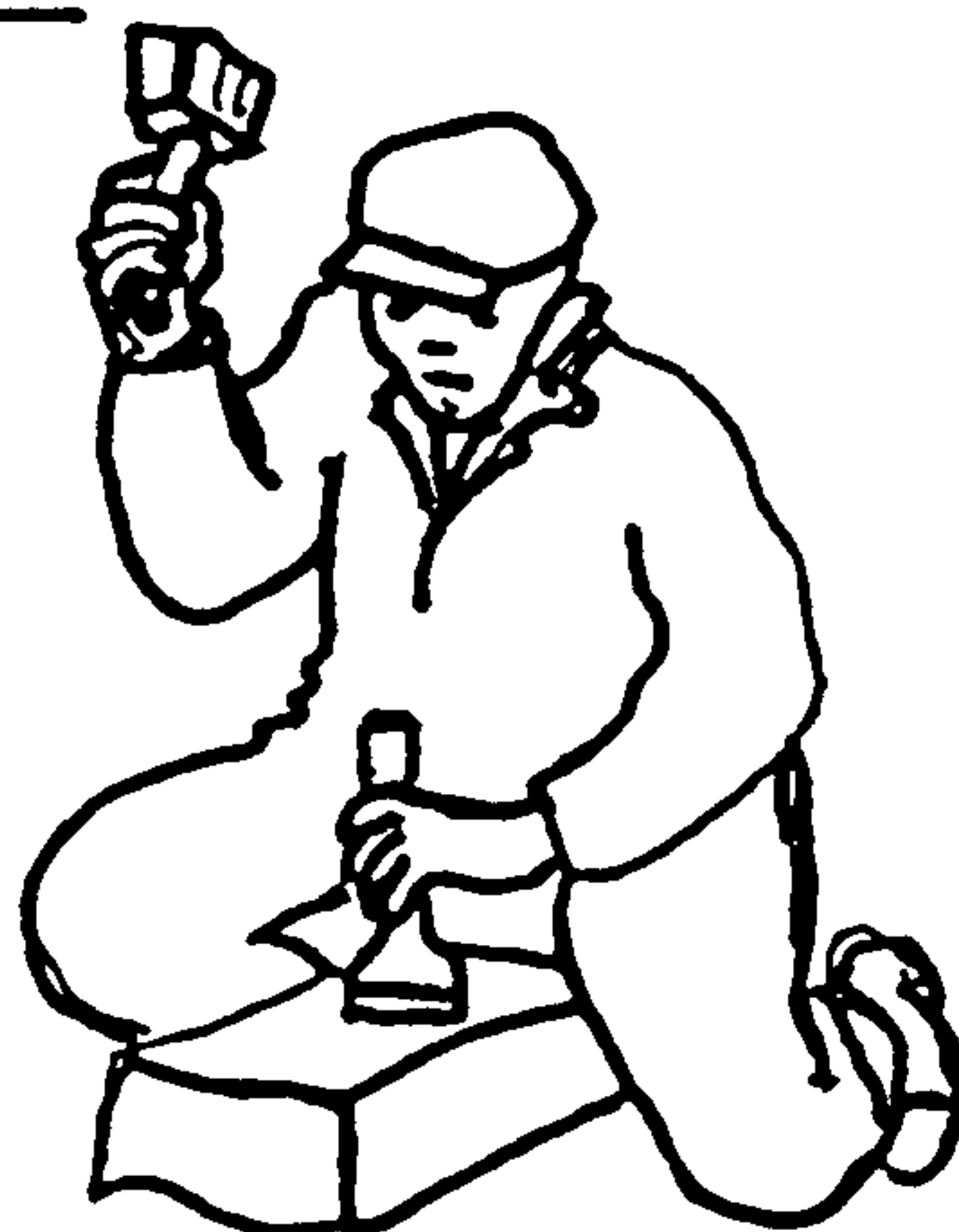
TRIMMING WITH A CHISEL.
