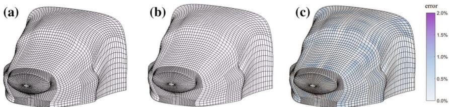
Fig. 8 Error comparison between the original PDE surface-represented (a) and NURBS surface-represented (b) high-speed train head where (c) uses different colours to visualize the errors between them
