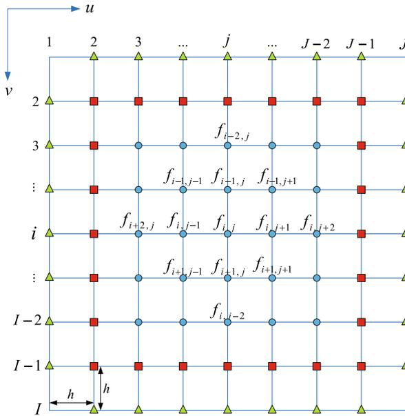
Fig. 2 Typical finite difference grid
