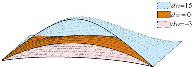
**Fig. 4** Effects of the weight deformation on a NURBS surface
