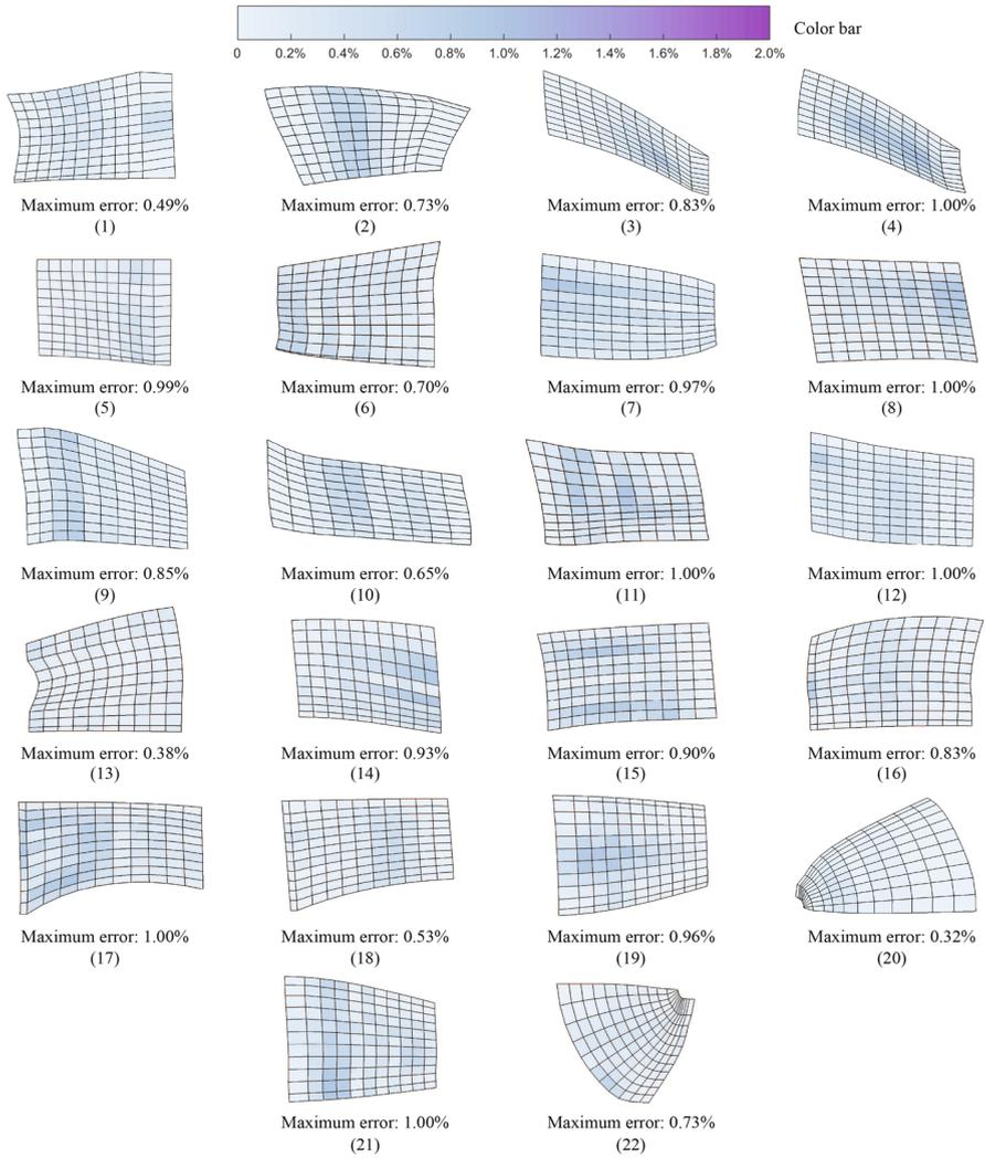
Fig. 7 Visualization of the errors between the PDE surface patches and NURBS surface patches
