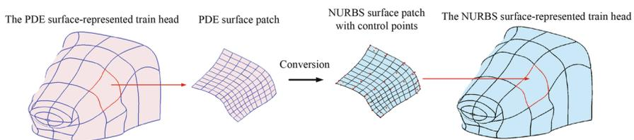
Fig. 5 Process of conversion
