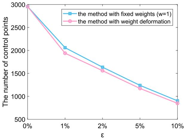
**Fig. 9** Effects of the required conversion accuracy and weight deformation
