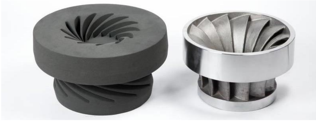
Figure 38: Sandcasting pattern and casting, © Voxeljet
