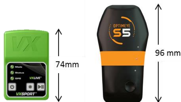
Figure 9 - Dimensions of VX Sport Log and Catapult Optimeye S5 Athlete Tracking Units
