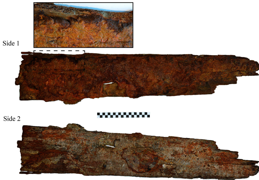
Figure 26. The recovered section of outer sheathing. Side 1 is the inside, revealing the layer of tar and hair and side 2 is the outside showing concretion from the iron nail fastenings. The scale is 20 cm (photo by Daniel Pascoe).
