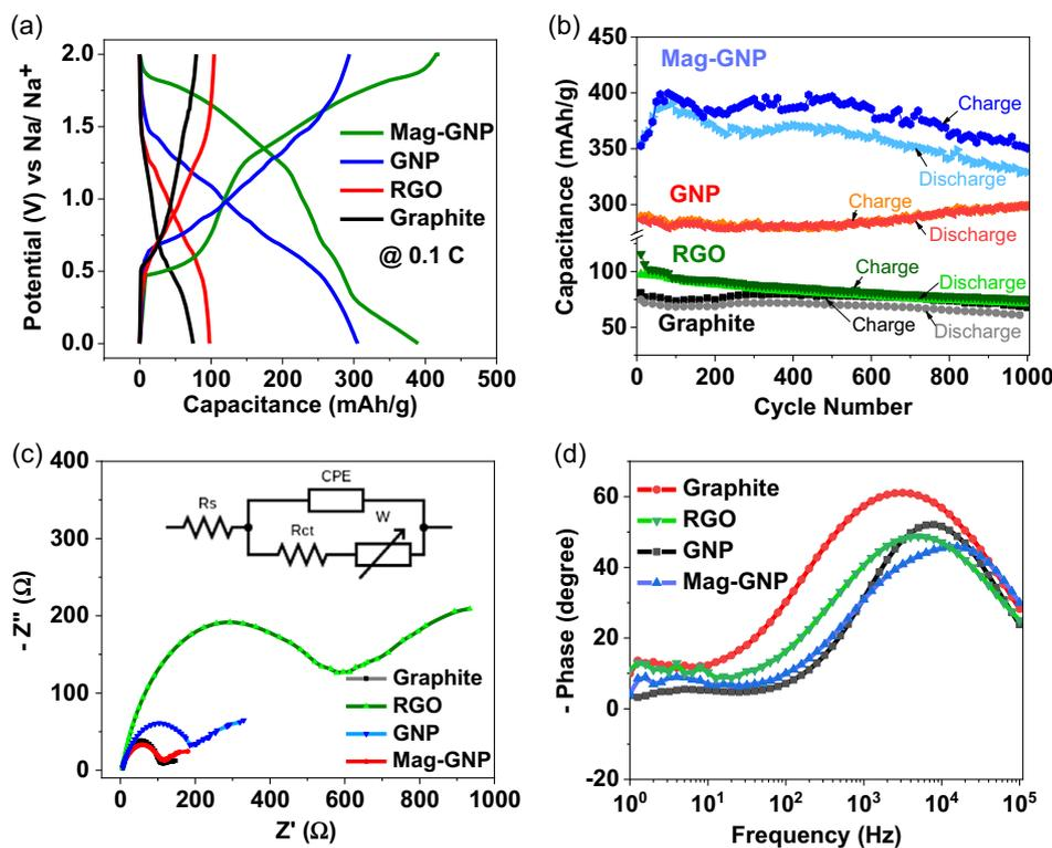
**Figure 5.** a) The comparison of galvanostatic charge–discharge curves, b) cyclability, c) Nyquist plot, and d) bode plot of Mag-GNP with other conventional graphene derivative anode material: graphite, RGO, and GNP.
