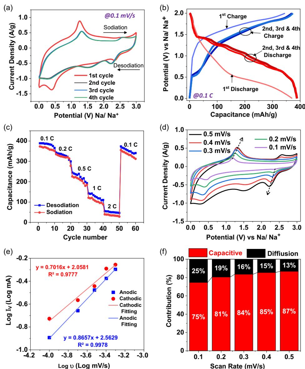
**Figure 4.** The consecutive first, second, and third cycles' a) CV curves and b) charge–discharge profiles of the Mag-GNP electrode in the voltage range of 0.01–3 V (vs Na/Na<sup>+</sup>), c) rate capability profiles of Mag-GNP anode, d) CV curves e) log  $i_p$ –log  $v$  plots of the Mag-GNP composite at different scan rates, and f) contribution of Na<sup>+</sup> ion storage mechanism of assembled SIB of Mag-GNP.
