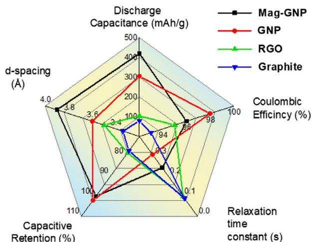
**Figure 6.** Radar chart of discharge capacitance of anodes (from half-cell setup of anode active materials), Coulombic efficiency, relaxation time constant, capacitive retention (at 1000 cycles), and interlayer distance (*d*-spacing) of Mag-GNP, GNP, RGO, and graphite.
