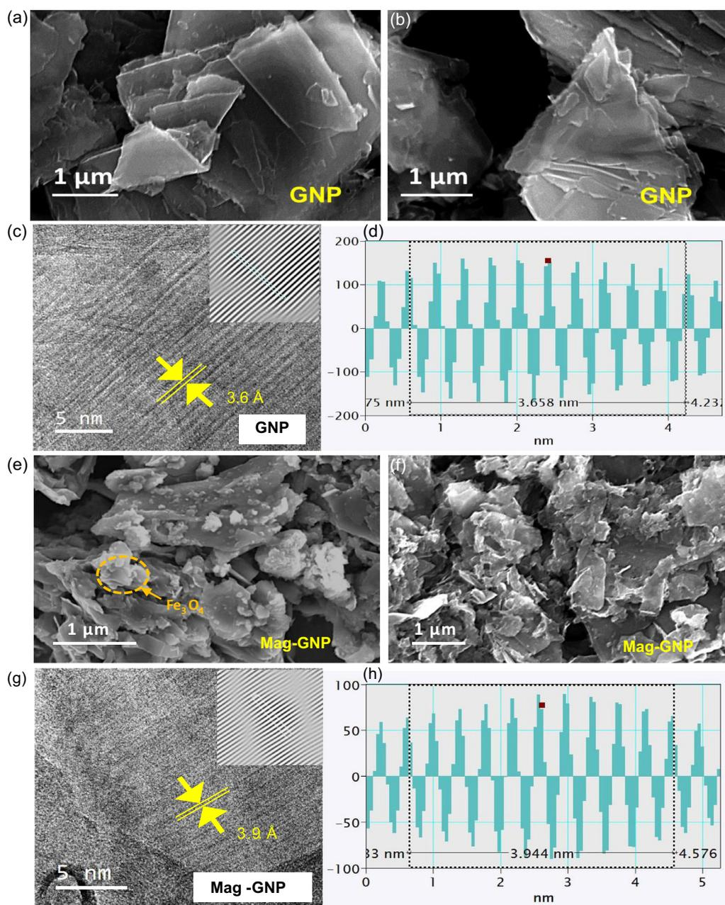
**Figure 2.** SEM images of a,b) the GNP and e,f) Mag-GNP, and high-resolution TEM images of c,d) the GNP and g,h) the Mag-GNP. The inset of the c,g) is the inverse fast Fourier transform patterns, and the d,h) are the interlayer *d*-spacing images of corresponding samples.
