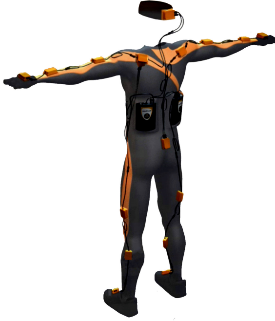
Figure 2.13: An example of a motion-capturing device, consisting of 17 inertial and magnetic sensor modules (Roetenberg et al. 2009).
