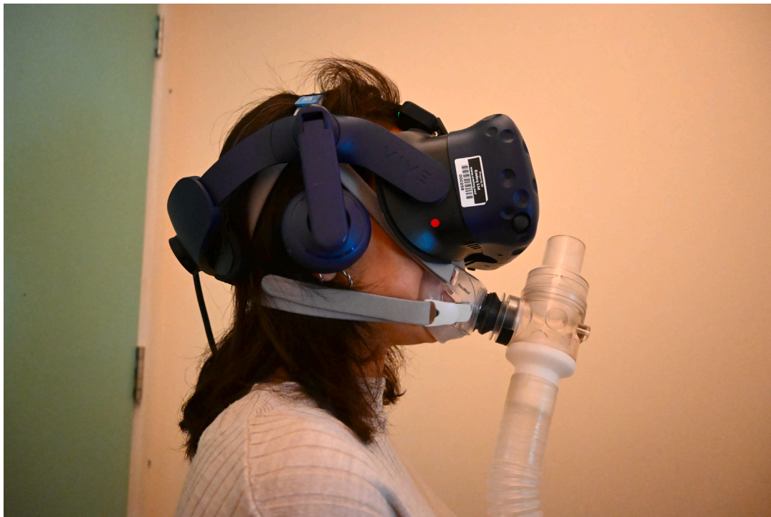
Fig. 2. Researcher demonstrating emteqPro VR device with the oronasal mask attached to a hose via a custom 3D printed adapter.
