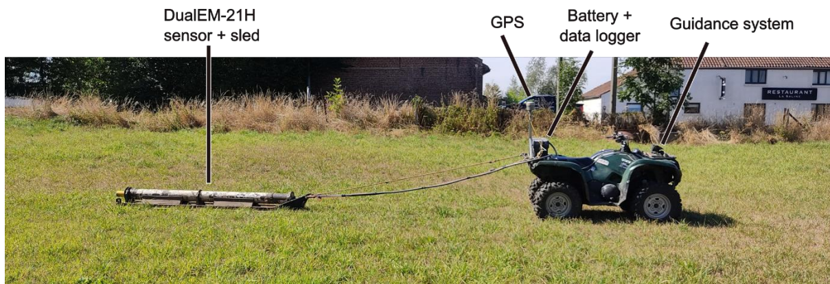
Figure 25: Mobile survey configuration for FDEM surveys. Photo by author.
