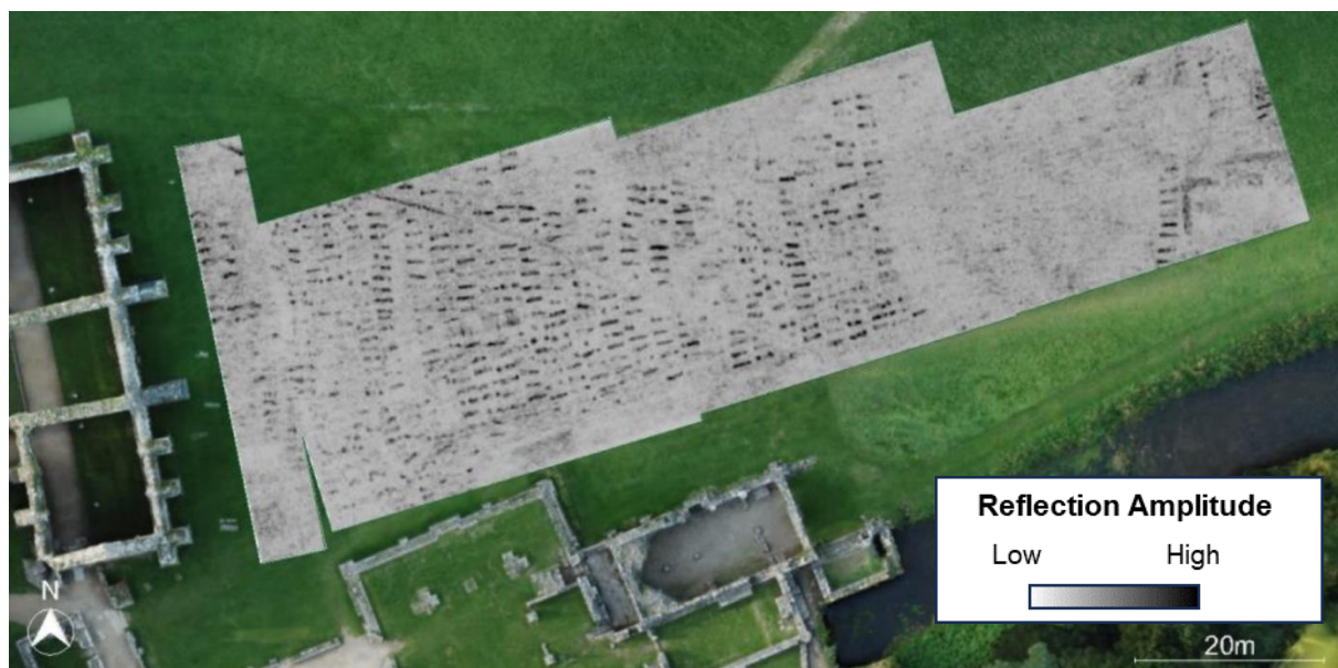
Figure 8: GPR amplitude slice map from Fountains Abbey (UK) showing individual graves as high amplitude anomalies (darker shaded discrete variations). Reproduced with permission (Gaffney et al. 2018, fig. 2)
