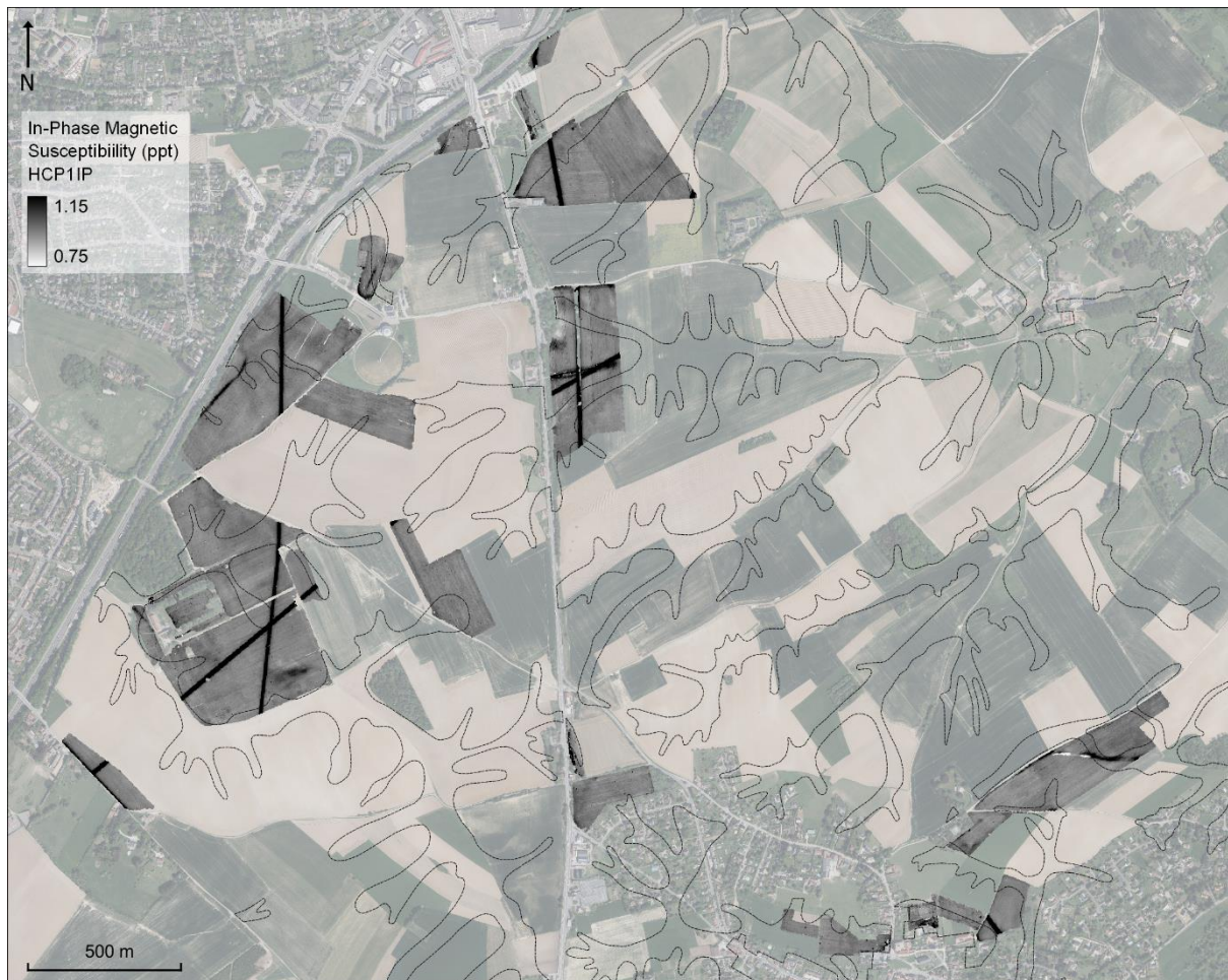
Figure 72: MSa data for coil pair HCP1. Colluvial deposits from 1950s soil surveys (Louis 1958, 1973) indicated by dotted black lines. Air photo basemap from Géoportail de Wallonie (2022). Figure by author.
