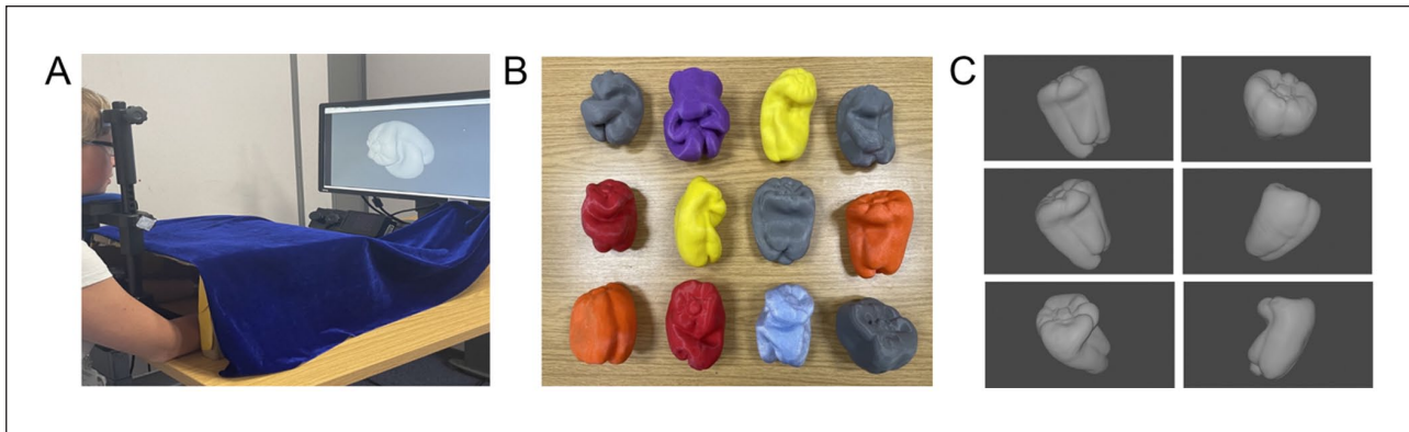
Figure 1. Set up and stimuli. (A.) Experimental setup. The head of the participant was stabilised by a chin and forehead rest. The haptic stimuli and the exploring hands were covered by a box and a curtain. In each trial with haptic exploration, one object was handed to the participant below the curtain from behind the screen. Visual stimuli were displayed on a computer screen. Eye movements were recorded by the EyeLink 1000 eye tracker. (B.) The haptic stimuli were 12 replicas of bell peppers with natural shape variations. (C.) Example of a visual stimulus with six views of the 3D model of the bell pepper showing the full rotation of the object in 60° steps, from top left to bottom right.
